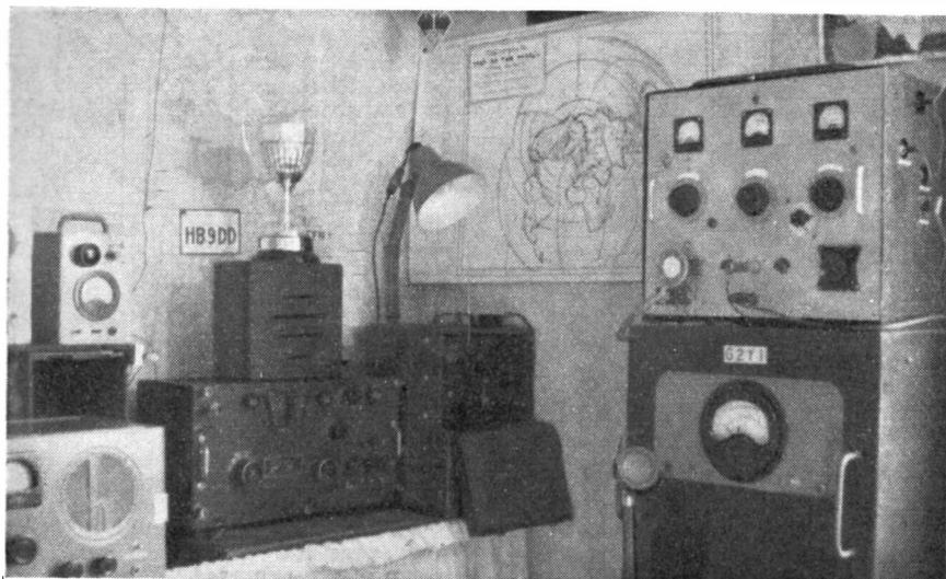
General view of the outfit at G2YI, Reading, Berks. ; his transmitter (on right) is a completely rebuilt 1154 for 1.7 and 3.5 mc operation. Receivers are Sky Champion and BC-342 and the trophy is the Reading Society's Lewis Cup, won by G2YI last year.
