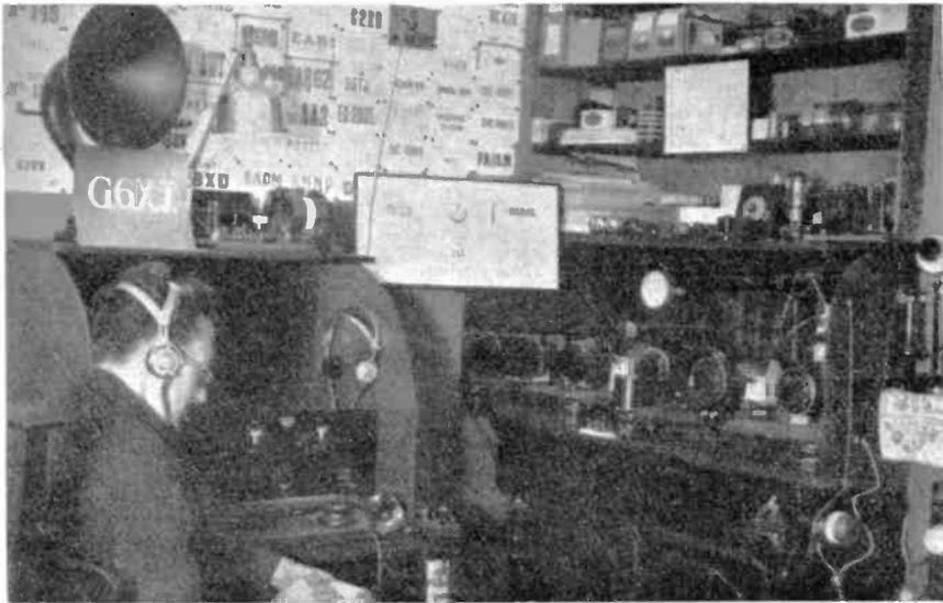
Early in 1929, G6XJ (now a director of Stratton & Co., Ltd., manufacturers of Eddystone equipment) operated this station in Birmingham. Two TPTG transmitters were run off the DC mains boosted by HT accumulators, and the receiver was a 1-V-1. Time marches on!
