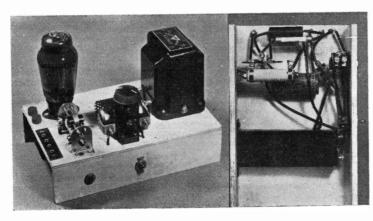
Two views of the modulator. The separate sockets are for filament supply; "P," "400," "PA" and earth are connected via the lower strip. The fixed bias resistor referred to in the text is underneath the left-hand variable resistor (R3).
