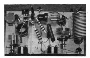
Layout of the RFP.15 tritet transmitter at 2FAG. The circuit is given in Fig. 1.
