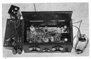
An Eddystone" Everyman Four" complete. The three dials are respectively bandset, reaction and bandspread. Points worth noting are good control with accessibility for coll changing from the top.
