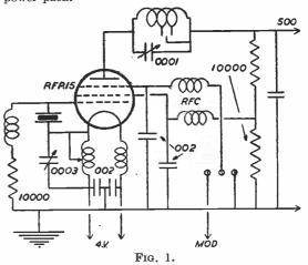
Circuit of the Tritet transmitter at 2FAG. Note the filament chokes for the RFP.15. A tapped tank coil is used, and the screen voltage taken from a potentiometer bleeding the HT supply. Modulation is applied to the sup, grid of the RFP.15.
