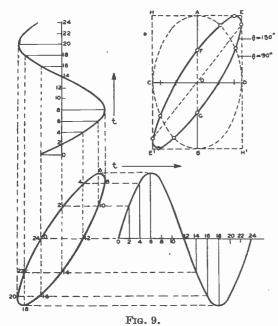
Diagram showing the formation of an ellipse from two sine waves out of phase and of different amplitude
