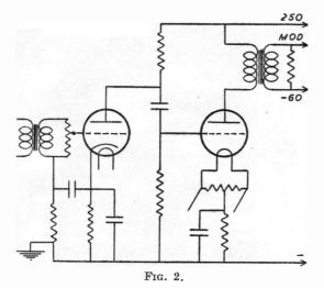
The speech amplifier-modulator used with the RFP.15 transmitter. A negative bias of -60 volts is applied to the sup. grid for 'phone working. The values in the resistor-condenser network in the amplifier depend largely on the valves used, but the resistance across the output of the modulation transformer can be 10,000 chms in most cases.
