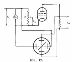
Circuit arrangement for measuring the amplification of a valve.
