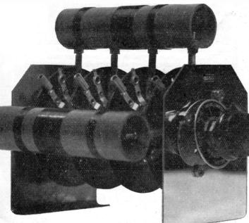
such switching system should be arranged so that the unused windings are left as much as possible "in the air," to avoid the losses and difficulties already mentioned.
