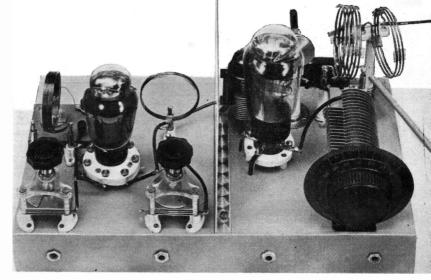
tive of input, i.e., the whole transmitter is tuned up for maximum output, as indicated by a rise on the PA plate meter, and brighest glow--or highest ammeter reading--in the AA. Note that too close coupling "kills" the PA output as shown by a *decrease* in RF indication in the AA, together with a big rise in PA plate current.
