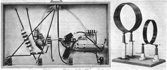
Under-chassis wiring is easily followed and on the right is a pattern of the PA and cathode coils.
