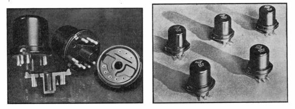
The Telefunken Steel Valves with their sockets and the new German octal base types.
