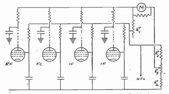
Skeleton Circuit showing position of an R-meter as described in the text
