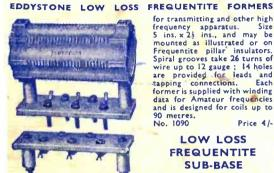
for transmitting and other high for transmitting and other high frequency apparatus. Size 5 ins. x 2½ ins., and may be mounted as illustrated or on Frequentite pillar insulators. Spiral grooves take 26 turns of wire up to 12 gauge ; 14 holes are provided for leads and tapping connections. Each former is supplied with winding data for Amateur frequencies and is designed for coils up to 90 metres. No. 1090
