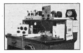
The AA Station of 2DBQ, C. Grant Dixon, Ghyll Bank, Whitehaven, Cumberland. He has a TRF receiver, and the transmitter is a two-stage 6L6 osc.dbir-6L6 PA. A C.R. tube unit is visible on the top shelf.
