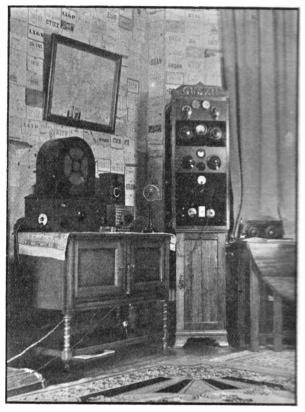
GW5XN has carried out a great deal of experimental work with aerials, the most successful up to date being a 67-foot Windom link coupled to the PA. The aerial tuning network can be seen at the top of the rack, with the PA, doubler-CO, and modulator speech-amplifier stages in order underneath. The receiver is a straight 1-V-2, and a monitor and test set are also visible to the right on the operating table.
