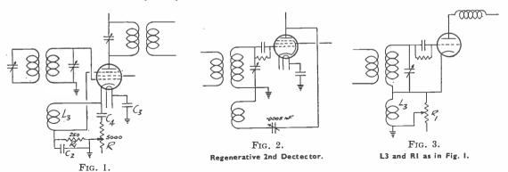
Condenser C3 from one side of the heater to earth prevents modulation hum.
