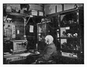
1.7, 3.5 and 14 Mc, on which he is normally, active. The 14 Mc rig is the QRO job, CO-FD-BA-PA, with 100 watts input to the pair of '10s in the push-pull final amplifier.
