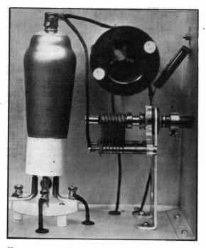
Close-up of the HF stage. Note the insulating bushes on C1, the HF tuning condenser.
