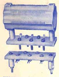
FREQUENTITE LOW LOSS FORMER Cat. No. 1090. Ideal for Amateur transmitters. Former size  $5^{\circ} \times 2\frac{1}{2}^{\circ}$ , spiral grooves take 26 turns of wire up to 12 gauge. Winding data supplied with former. Price 4/-
