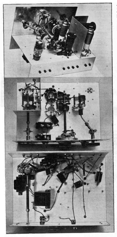
extension set. Slow motion is fitted, again by means of Eddystone driving heads and dial assemblies, to both Cl and C5. The mounting of R8 will be clear from the under-chassis photograph; remember that a B.T.S. bracket must be used here, to get both the correct height and the required insulation.
