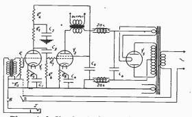
Theoretical Circuit of the Amplifier used for Modulating the Hartley Oscillator described in the March, 1938 article.
