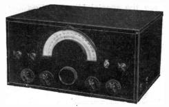
in five steps from 10 to 160 metres. Three models are available, priced from £20 to £22. The power supply is not incorporated in the receiver, separate packs are available for purchasers who have not a supply to hand.
