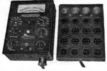
valve will work in a set. This is a great advance over the usual emission test, which does not give a reliable indication of valve "goodness."
