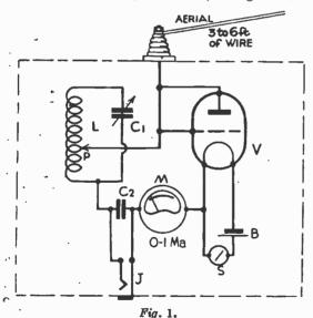
Circuit of field strength meter with diode rectifier.
