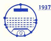
THE ALL-STAGE VALVE. This is a Multi-Grid Critical Distance valve which is so constructed, that it makes possible the production of a Multi-Valve receiver, such as a superhet, using only one type of valve throughout.
