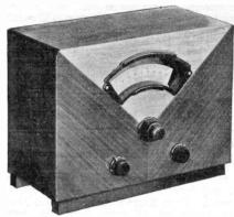
By the use of a carefully developed circuit arrangement, the two self-contained aerials and a powerful valve combination, having six separate functions, this receiver measuring only 11 in. x 12 in. x 8½ in. provides performance which is equal in sensitivity and quality of reproduction to instruments of standard size of similar type. The set weights but a few pounds, is neat and compact, and with carrying handle, may be taken from room to room as required.
