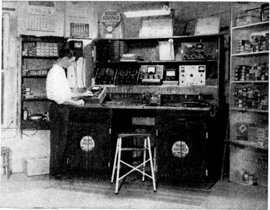
Fig. 5. Example of good service bench having many of features described in this chapter. Bench should be located for shortest possible path to car or truck, so heavy television sets will not have to be carried too far. (Sylvania photo)
