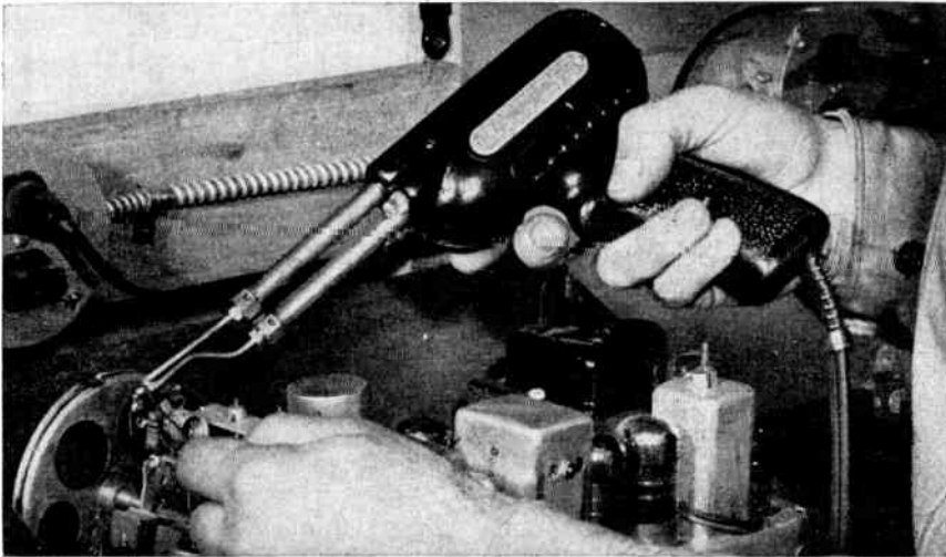
Fig. 1. Using a Weller soldering gun for unsoldering the leads of a defective part in a radio receiver. Spotlight bulb on gun throws needed light directly on joint. (GE photo)
