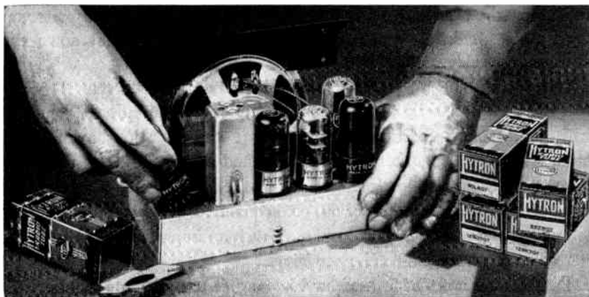
Fig. 4. Putting an entire new set of tubes in a table-model radio will make it work again about half the time. The old tubes can then be put back one by one, to find the tube that makes the set go bad again. (Hytron photo)
