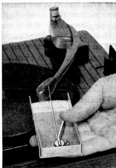
Fig. 7B. Measuring horizontal friction of tone arm. Three nuts serve as weights at rear of tone arm to balance it. Under 3 grams is correct. (Philca photo)
