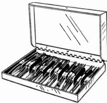
Fig. 11. Examples of IRC carban-resistor stack cabinets having sizes most needed for repairing television and radio sets. The larger the kit, the more likely it is to have the particular resistance value needed. Note that up to six resistors are furnished for the most needed sizes
