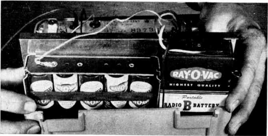
Fig. 8. Inserting tray of new batteries in cabinet of three-way portable, after tying the 67½-volt B battery to the tray with a piece of wire. The five flashlight cells are installed with caps alternately up and down to provide the required series connection for 7½ volts. Always note battery positions carefully before removing them. (Ray-O-Vac photo)
