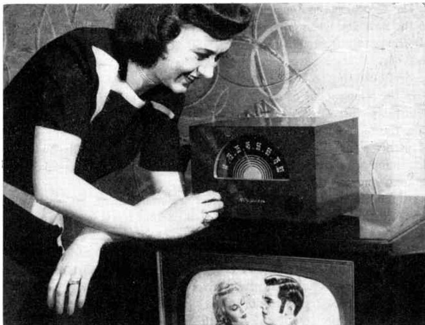
Fig. 9. Converter unit being used with vhf television receiver to bring in stations. Dial is marked in uhf channel numbers from 14 to 83. (RCA Victor photo)
