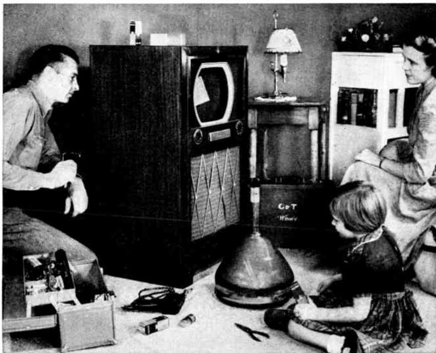
Fig. 2. Example of another good toolbox for home calls. On television calls, many servicemen carry the required large number of spare tubes in a traveling bag like that directly behind the picture tube on the floor here
