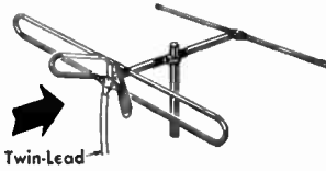
(B) Broadband Batwing and Reflector
