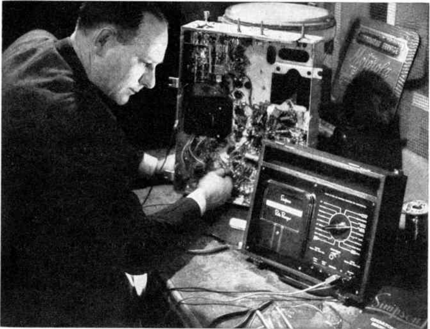
Fig. 3. A simple bench, a few tools, and a good multimeter get you started in profitable television servicing. (Simpson photo)
