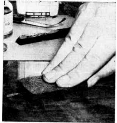
Fig. 4. Rubbing hardened stick shellac in scratch with felt pad moistened with shellac rubbing fluid, to make the repair level with the surrounding finish. (General Cement photo)
