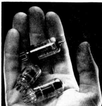
Fig. 6. Examples of miniature tubes, which have no separate bases. Most are 7-pin and have a wider gap between two of the pins to ensure correct insertion. (Sylvania photo)
