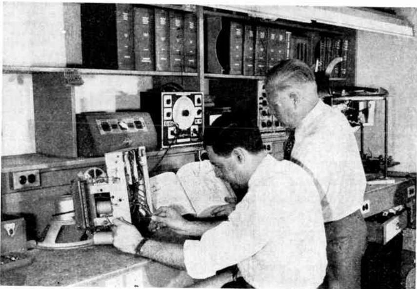
Fig. 7. Using a Rider's Manual for reference while hunting for trouble in the chassis of a console radio. Other manuals are within easy reach on the shelf. (John F. Rider photo)
