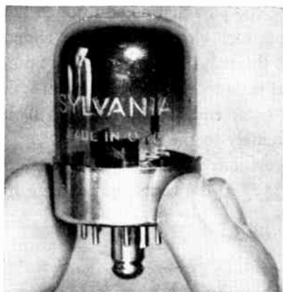
Fig. 5. Example of a Ioktal tube, showing glass envelope, metal base, metal aligning key, and solid wire pins that go right through the glass envelope. (Sylvania photo)
