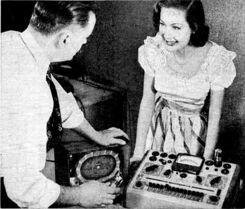
Fig. 2. Home calls provide an interesting change in the daily routine of servicing. Tubes are tested right in the home because they are the commonest cause of trouble. (Sylvania photo)
