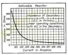
Fig. 2. Change in secondary reactance vs. primary current.
