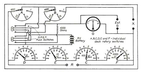
Fig. 2. Wheatstone bridge circuit.
