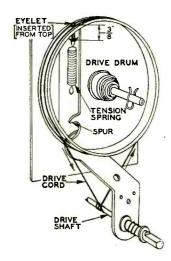
panel and bring the cord mentioned in the previous paragraph down to the drive shaft. Wrap this cord directly below the drive drum three and one-half turns around the drive shaft, as shown in Fig. 1, progressing toward the back of chassis.
