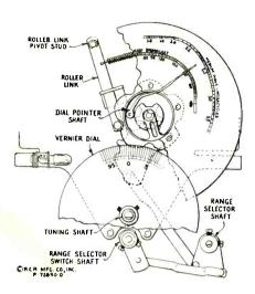
Fig. 2. RCA tuning mechanism.
