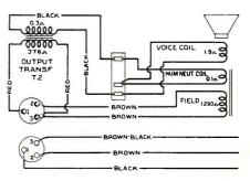
Fig. 4. RCA speaker connections.
