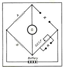
Fig. 1. Fundamental bridge circuit.
