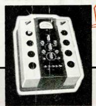
The WESTON Model 772 Analyzer. Sensitivity of 20,000 ohms per volt . . . resistance ranges readable up to 30 megohms ance ranges readable up to 30 megohms indications as low as ½ . . . eurrent indications as low as ½ microampere. Will put you years ahead microampere. Will put you years ahead of competition. Price \$46.50 net to dealers in U.S. A.
