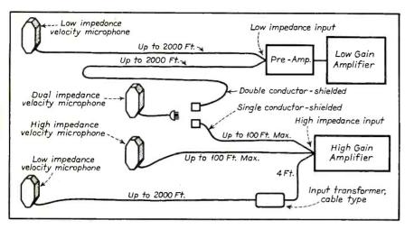
Fig. 5. Velocity microphone connections.
