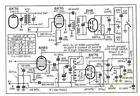
Fig. 2. Philco magnetic tuning circuit.
