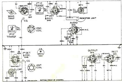
Fig. 2. Socket voltages and trimmer locations.
