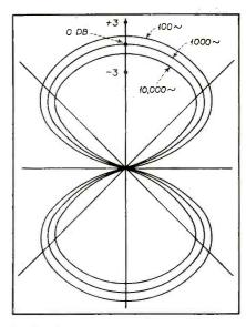
Fig. 2. Directional characteristic of velocity microphone.
