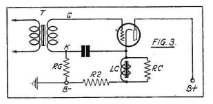
This is a simplified version of the first section or input of the Triple-Twin tube. It will better serve to clarify the action of this part of the tube as an amplifier. The function of the resistor RG is to supply bias to the grid
