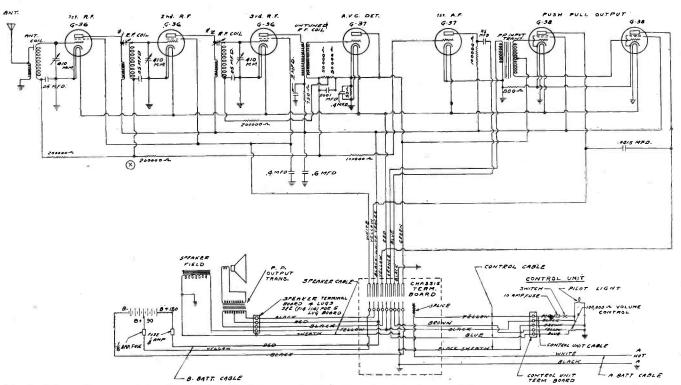
Fig. 1. Circuit diagram of the Majestic Model 110 Auto Radio. Note that this chassis utilizes an automatic volume control system in combination with a diode detector, the G-37 tube serving both functions. (Courtesy, Grigsby-Grunow Co.)
