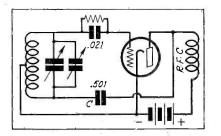
Fig. A. Circuit of a capacity-coupled Hartly oscillator
