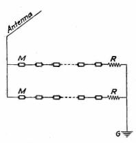
Fig. 2. Typical layout when two horizontal branch risers are used. Maximum, eighteen Multicouplers shown in Fig. 1; (3) Three downleads having three to six Multicouplers in series in each lead (It is not well to use more than three downleads with each antenna.); (4) One or two horizontal risers connected to a single antenna for two- or three-story buildings, as shown in Fig. 2.
