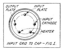
When testing a set with a **Triple-Twin** tube, keep in mind that both plates are connected to the tube prongs, as shown. The input grid connects to the cap on the tube
