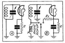
The above circuits indicate the manner in which a phonograph pickup should be connected into the grid circuit of a detector tube
