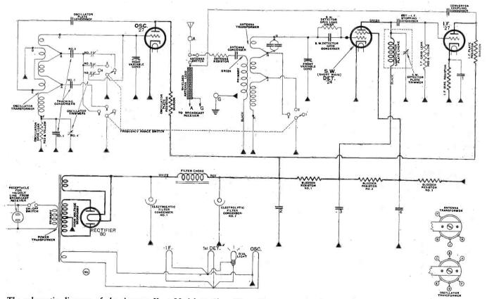
The schematic diagram of the Atwater Kent Model 93 Short-Wave Converter, with its attendant power unit. An intermediate frequency of 1,000 kc. is employed. Note that tapped coils are used in connection with a series of condensers to effect a change of waveband. The lettering on the terminals of the antenna and oscillator transformers, as shown in the right hand corner, correspond to the lettering in the circuit diagram above. (Courtesy, Atwater Kent Mfg. Co.)
