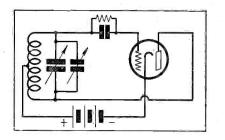
Fig. B. Circuit of the conventional Hartly oscillator
