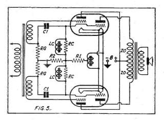
The circuit of two Triple-Twins in push-pull. This arrangement, with 250 volts on the plates and a load impedance of 8,000 ohms, will furnish about 14 watts output
