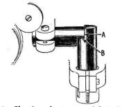
Fig. 3. Showing the two special studs in place for the exciter lamp socket adjustment
