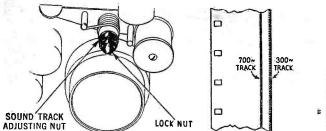
Fig. 4. (left) This sketch shows the pressure roller adjusting screws referred to in the text. Care should be taken in tightening the lock nut. Fig. 5. (right) A section of Buzz Track Film, which carries sound tracks of 300 and 700 cycles
