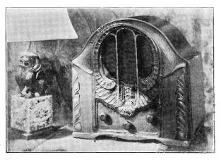
and mechanical refinements embodied in the design, the outstanding features are to be noted. The tubes required for this set are two type '35 tubes, three '24s, one '47, and an '80. These few words tell the whole story to the technician; that of ultra-modernism in radio set design. Referring now to the schematic circuit, Fig. 1, we find that V1, one of the new type '35 tubes (first known as the variable-mu, and now vari-
