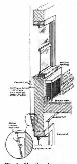
Fig. 3. Showing the manner in which the individual installations should be made. Note the special terminal resistor, in circle
