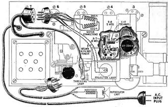
when operated at about 110 volts. The normal life of this lamp is about 25 hours. This rating is the equivalent of about 75 reels carrying 400 feet of film each, or about 300 reels of 100 feet each. The usual run of 16 mm. film is projected at a rate of about 20 feet per minute.
