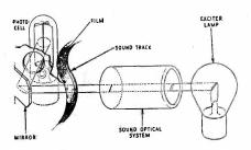
Fig. 2. View of the sound system. Note the slits through which the light must pass
