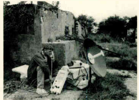
In remote areas beyond the reach of telephone links, or in places of natural disaster where telephone lines are down, the Inmarsat-A transportable communications terminal is a vital link for rescue workers and the media.
