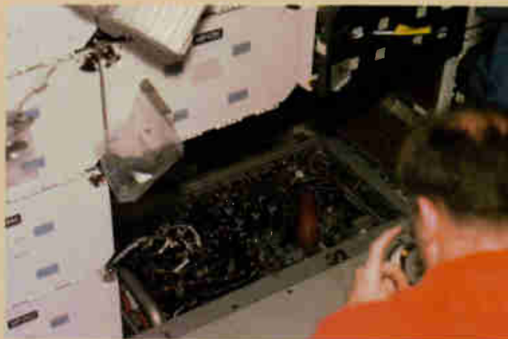
This Electronic Still Camera (ESC) image shows astronaut Richard A. Searfoss, commander, performing in-flight maintenance (IFM). The Regenerative Carbon Dioxide Removal System (RCRS) shutdown April 24, 1998, setting off an alarm and delaying the crew's sleep period several hours. Searfoss removed a hose clamp and used tape to bypass a check valve that had threatened to cut the flight short. The valve, part of the air-scrubbing systems plumbing that recirculates nitrogen back into the cabin atmosphere, was allowing cabin pressure to leak into the system throwing off its electronics control unit. This ESC view was taken on April 25, 1998 at 17:26:49GMT.
