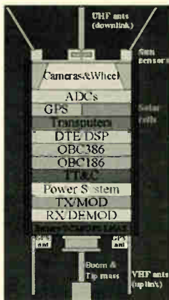
Basic structure of TMSAT-1 showing placement of the satellite's various subsystems. (SSTL Web site photo)
