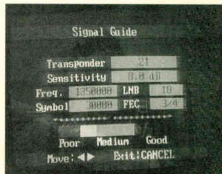
The Pansat 100A Signal Guide screen gives you all the data you need to adjust your dish for optimum signal strength.
