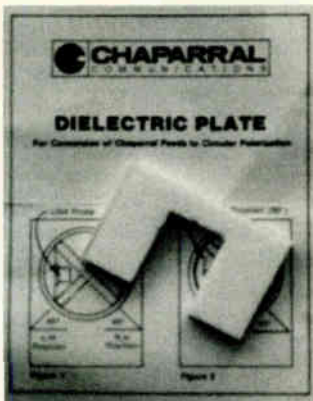
Chaparral makes a Teflon insert which, when inserted into the feed horn, allows a linear polarity feed horn to receive circularly polarized signals. This insert was modified to accommodate a C/Ku-band feed (note large notch).
