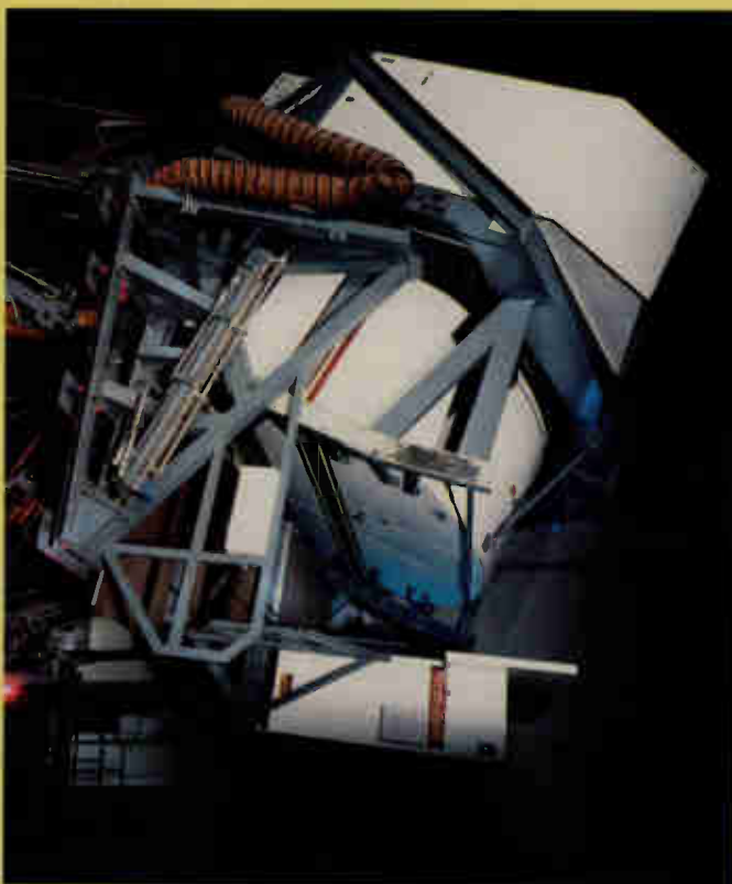
The motion base Shuttle Mission Simulator in Johnson Space Center's Mission Simulation and Training Facility.
