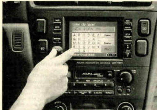
Acura's system incorporates electrogyros as well as GPS for its navigation
