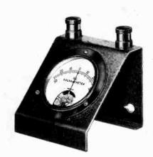
Fig. 1-5. A Weston center zero galvanometer.
