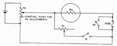
Fig. 3-10. Method for determining meter resistance.
