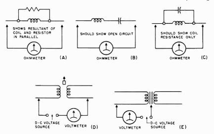
Fig. 10-30. Various combinations of coils, capacitors and resistors which can be tested as explained in the text.
