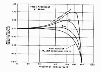
Courtesy of Sylvania Fig. 9-22. Graph of voltmeter reading error versus frequency of measured voltage for various voltage values measured on a v-t voltmeter using a diode-rectifier probe with a 5647 tube.
