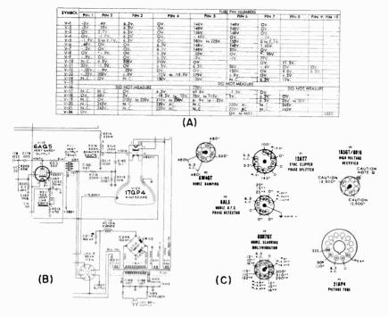
Fig. 10-32 (A) Voltage chart. (A) Emerson. Fig. 10-32 (B) Partial schematic showing operating voltages next to tube electrode symbols. (B) RCA. Fig. 10-32 (C) Voltage labels adjacent to socket terminals or underside of chassis. (C) Stewart Warner.
