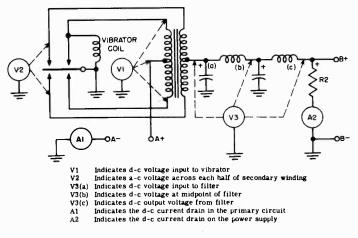
Fig. 10-46. Full wave synchronous vibrator power supply.
