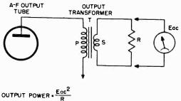
Fig. 10-54. Measuring the power output of an a-f amplifier.
