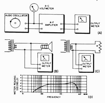
Fig. 10-55. Arrangements for making frequency-response measurements of an a-f amplifier.
