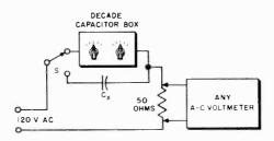
Fig. 10-17. Comparison method for measuring capacitance.
