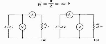
Fig. 5-2 If the ammeter A is connected as shown in A at the left, only the current drawn by the load  $R_L$  will be indicated on it; if it is connected as in B, right, then the ammeter reading will be the current drawn by both the load and the voltmeter, V.
