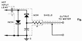
Fig. 9-21. Simple peak-to-peak r-f probe for VTVM.
