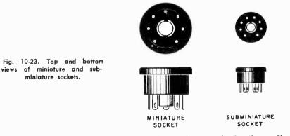
Many octal sockets have only five active terminals (for a five-pin tube), and others make use of every terminal, because the tube inserted in the socket has eight live electrode connections. Other kinds of sockets may bear more than eight terminals, depending on the tube used, and
