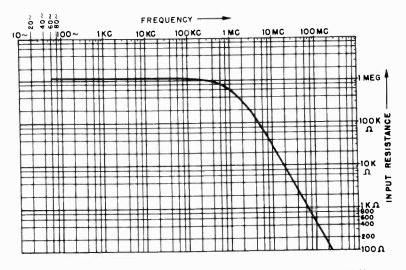
Fig. 9-24. Input resistance vs frequency curve for RCA type WV-75A.
