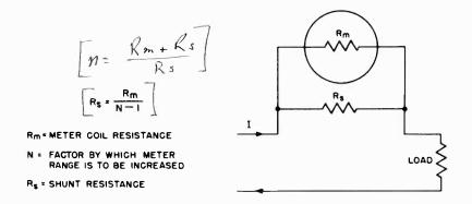
Fig. 3-4. Formula for calculating shunt resistors to increase the current range of a basic meter movement.
