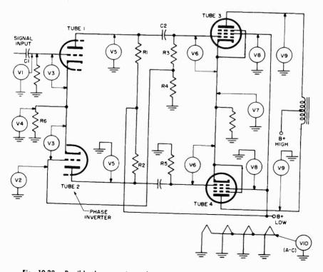
Fig. 10-38. Possible d-c operating voltage measurements in a typical phase inverter push-pull amplifier system.
