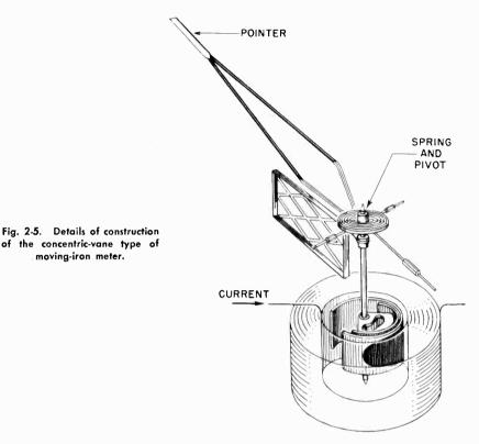
Because of the square relation between the displacement and current, explained above, the displacement of the moving iron in this type of meter is directly proportional to the rms value of the current being measured. Thus this type of meter can read a-c and d-c values on the same scale and is not sensitive to waveform.
