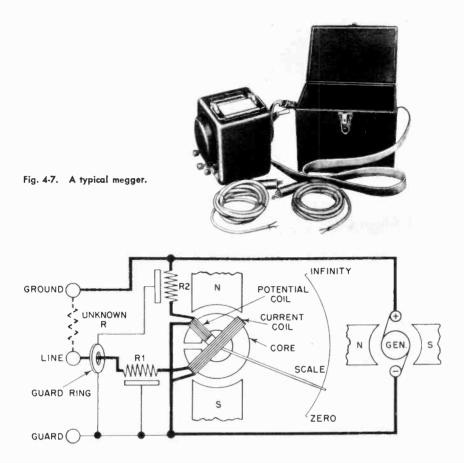
Fig. 4-8. Circuit of a typical megger. The metal guard ring and associated components prevent leakage currents along the surface of the instrument case when readings over 100 megohms are being made.
