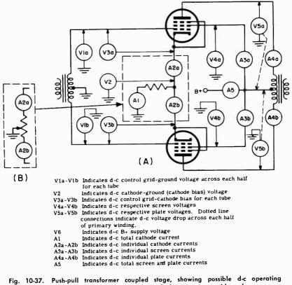
Fig. 10-37. Push-pull transformer coupled stage, snowing possible are operating voltage and current readings. For triodes, eliminate screen grid and suppressor grid circuits.
