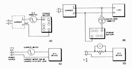
Fig. 10-9. (A) An ammeter connected to indicate rate of battery charge. (B) A centerzero meter used as a charge-discharge instrument. (C and D) Ammeter and voltmeter connected to measure current drain and power of device operated from the power line.
