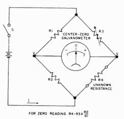
Fig. 10-10. Wheatstone bridge circuit for measuring resistances.
