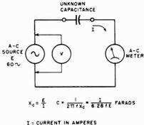
Fig. 10-16. Use of a-c source and current meter to measure capacitance. The a-c voltage source can be an isolation transformer with 120-volt output.
