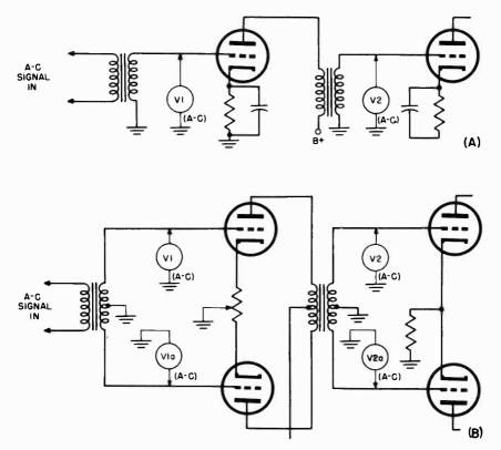
Fig. 10-53. Measuring gain in transformer-coupled amplifier.
