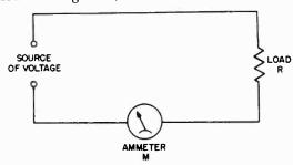
Fig. 3-13. For current readings, the meter should always be connected in series with the load whose current is to be indicated, as shown here.
