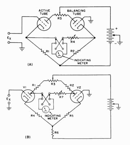
Fig. 9-4. (A) A two-tube v-t voltmeter in which the resistance arms are connected in series with the cathodes providing degeneration as well as a bridge balance. The meter is connected between the cathodes. (B) Two-tube push-pull bridge d-c amplifier, with meter connected between the plates.
