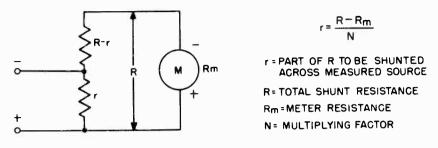
Fig. 8-2. The universal shunt and applicable equation.
