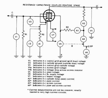
Fig. 10-36. A pentode resistance-capacitance-coupled amplifier stage and typical meter reading locations. For a triode in the same circuit, simply eliminate the screen grid and suppressor circuits.
