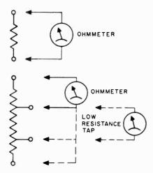
Fig. 10-27. When the resistance of a tapped resistor is being measured, each tap should be checked against a common point at one end, as indicated by this Figure. In addition, if the resistance of one section is relatively low, a separate reading directly across it is in order.
