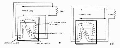
Fig. 5-4. Organization of dynamometer type wattmeter.
