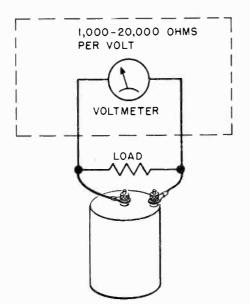
Fig. 10-8. Determining terminal voltage of a battery.
