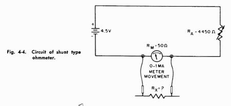
deflection of the meter. A typical shunt-type ohmmeter scale is shown in Fig. 4-5. Notice that the direction of increase of resistance is just the opposite of that for the series-type ohmmeter scale shown in Fig. 4-4. **4-5. Voltage-Divider or Potentiometer-Type Ohmmeter**
