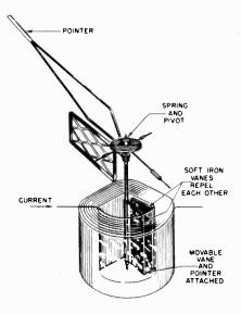
Fig. 2-4. Details of construction of the radiol-vone type of moving iron meter.
