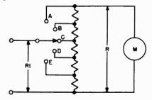
Fig. 3-2. Example of multiple current scale.
