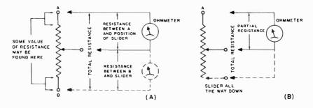
Fig. 10-28. Diagrams illustrating the measurement of variable resistors.
