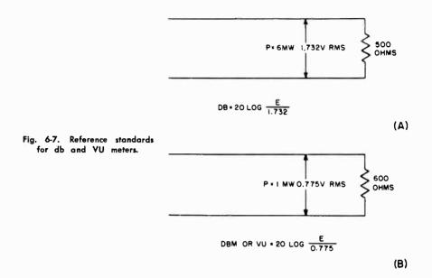
In most applications, VU and other level meters are used for *relative* readings, and the zero level may be any voltage desirable or convenient at the moment. If an absolute reading is required, however, it must be taken across an impedance of 500 or 600 ohms, whichever the scale calls for.
