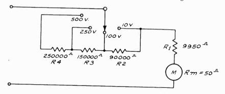
Fig. 8-7. Switching system for series connected voltmeter multipliers, using 50 μα meter for 500-volt maximum scale.
