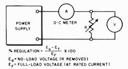
Fig. 10-19. Determining voltage regulation of a power supply.
