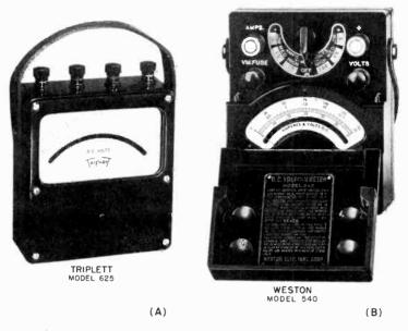
Fig. 8-1. Photos of multi-range instruments with terminals and with switch selector. (A) Triplett, (B) Weston.
