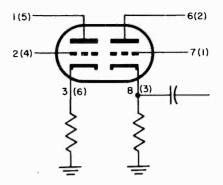
Fig. 10-26. Alternate numbers adjacent to tube pin symbols indicating difference in numbers when alternate tubes are used in socket.
