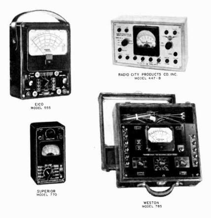
Fig. 10-2. Photographs of typical, modern volt-ohm-milliammeter. (Note: The above photos are reproduced through the courtesy of the manufacturers indicated.)
