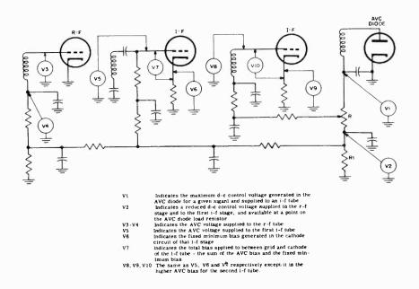
Fig. 10-39. Examples of d-c control voltage measurements in radio receiver.
