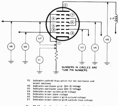
Fig. 10-43. Another type of converter circuit.
