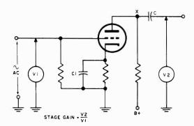
Fig. 10-52. Arrangement for measuring stage gain of an a-f amplifier using a-c meters of suitable type.
