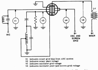
Fig. 10-42. Typical converter circuit with voltage-checking points.
