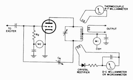
Fig. 11-3. Two methods of using meters to indicate r-f in the plate circuit of a class C amplifier during neutralizing procedure.
