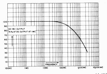
Fig. 9-23. Frequency correction curve for the Millivac Instruments model MV-18B using crystal probes.
