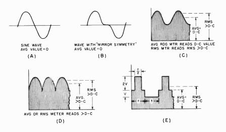
Fig. 10-33. How combinations of a-c and d-c voltages affect meter readings. A d-c voltage reading with a permanent-magnet moving-coil meter is affected by the presence of an added a-c component only if the latter has an average value different from zero, as in (D). Note, in (E), that an a-c component wave does not have to be symmetrical to have an average value of zero.
