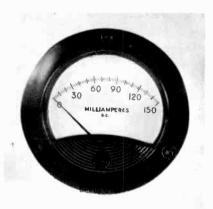
Fig. 1-4. The linear scale used with a typical moving coil meter.
