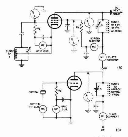
Fig. 11-(A) Electron-coupled oscillator circuit, such as is used for the frequencycontrolling circuit of transmitters, and locations of typical meter measurements. Fig. 11-(B) Crystal oscillator circuit and meter measuring locations.
