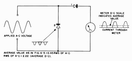
Fig. 6-3. Double-rectifier arrangement, which minimizes "back-current."
