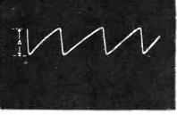
Horizontal Saw Gen Tube V2 Pin 5 A=50 volts
