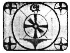
Fig. 23. Focus Control Misadjusted
