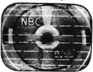
Fig. 17 Auto Ignition Interference
