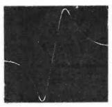
Figure 15-L Properly aligned discriminator curve. Birdie at 21.9 mc.
