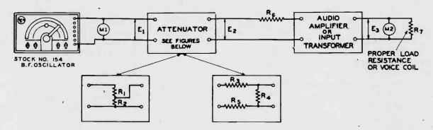
Connections for Measurement of Audio Amplifier Frequency Response
