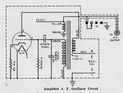
Part of Circuit of Triplett Model 2432 Signal Generator
