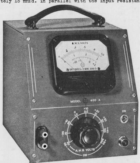
The instrument is calibrated to indicate the RMS value of a sine wave, but the instrument responds to the average value of the rectified full wave applied. Because both the positive and negative portions of the applied wave thus influence the meter, "turn-over" effects are negligible and errors caused by the presence of harmonics in the applied voltage are minimized.
