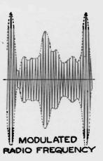
frequency which is modulating the signal. Notice that the lower envelope is this audio frequency also, but in reverse.
