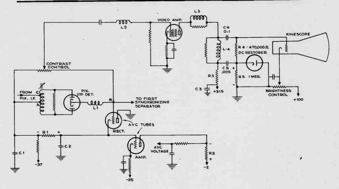
Picture Second Detector, Video Amplifier and D.C. Restorer
