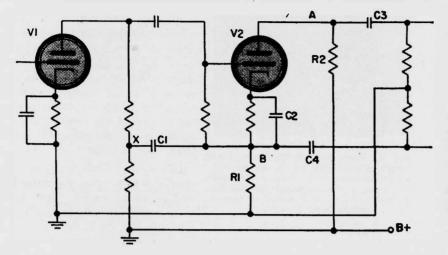
Fig. 4 A phase inverter utilizing the cathode follower principle.
