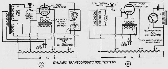
The dynamic transconductance tester like the previous one, applies recommended D.C. voltages to each tube electrode. These voltages are obtained and checked in the same manner as before. But, unlike the static test, the dynamic transconductance test requires an A.C. grid signal, which more closely approximates tube operating conditions. A 60-cycle voltage from the secondary winding of a step-down transformer is a satisfactory signal.
