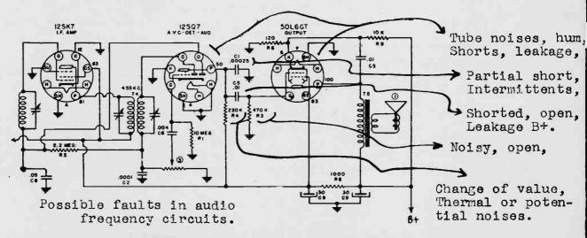
The majority of faults in audio voltage amplifiers lie in the tube itself or in the coupling condenser. Generally, this stage gives little trouble. Plate coupling condensers must be of high quality, since even the slightest amount of leakage may cause the grid of the next tube to become positive.
