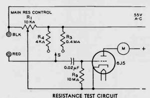
Dual range a-c Wheatstone bridge used for resistance measurements.
