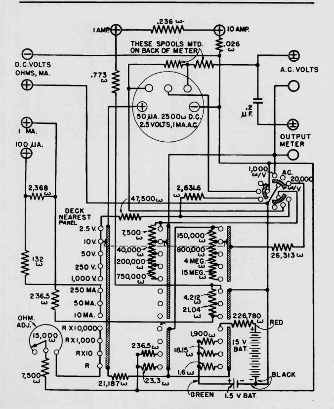
Wiring Diagram of Model 772
