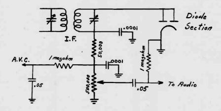
The diode load may be in the form of a smaller R.F. filter resister of 50,000 ohms by-passed on each side by small condensers which offer low impedance to R.F. (or I.F.) and do not pass audio frequencies which exist across this resistor in series with the 500,000 ohm volume control. At the junction of these two resistors, is connected an audio filter so that the A.V.C. voltage applied to various other tubes is essentially D.C. changing in value with carrier intensity and not audio variations.
