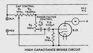
figure. Here Rl and R2 together comprise the calibrated adjustable ratio arm of the bridge. R5 is the power-factor balance rheostat in both figures.
