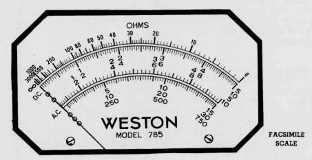
An ohmmeter should provide means for determining values commonly encountered in radio service work. However, the more popular instruments will not measure accurately above 1/2 megohm, and higher values if present cannot be tested.
