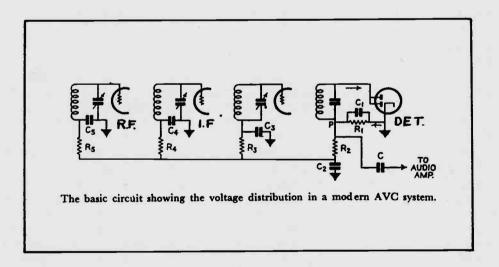
Overloading or distortion traced to A.V.C. is usually due to leaky filter condenser in A.V.C. circuit. Remove old condenser and connect a new one to test for fault — do not shunt the new one across the old condenser.
