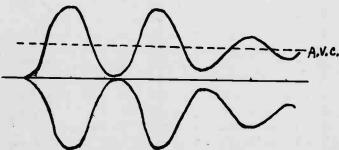
Envelope of Audio Modulated Carrier Signal Showing Value of Filtered A.V.C. Voltage with Steady Carrier but Variable Modulation.
