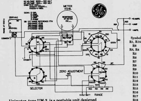
Unimeter, type UM-3, is a portable unit designed for simplicity, attractive appearance and rugged construction, for the rapid and accurate measurement of volts, ohms, current and decibels as encountered in the repair of electronic equipment. All components with the exception of the ohmmeter batteries are mounted on an aluminum panel. The unimeter is contained in a fabricated steel case with removable cover. With reasonable care the unit should give many years of service.
