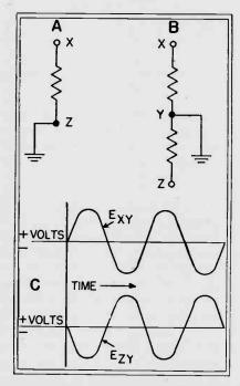
Fig. 1 A representation of single- and double-ended circuits. A represents the load circuit of a single-ended amplifier and B represents the load circuit of a double-ended amplifier. C shows the phase relationships of the voltage present in B when a sine wave signal is applied across points X and Y.
