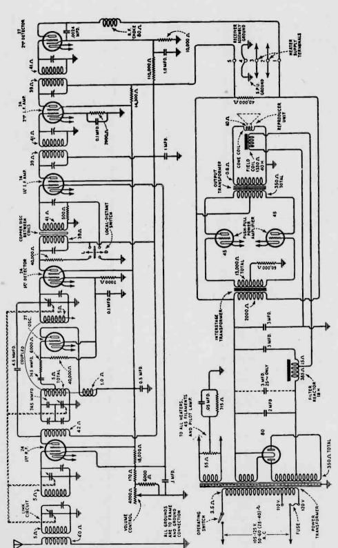
We illustrate circuit of R.C.A. Model 80 radio receiver to offer some suggestion for resistance point-to-point testing. Please note that this diagram includes many resistance values for components other than resistors. This additional information is helpful for detecting variations which may be the cause of existing fault.
