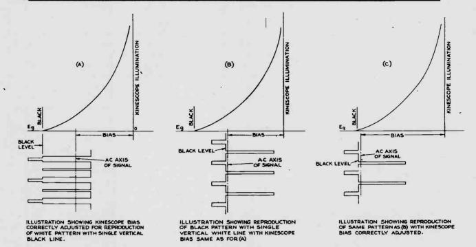
Operation of D.C. Restorer or Automatic Brightness Control
