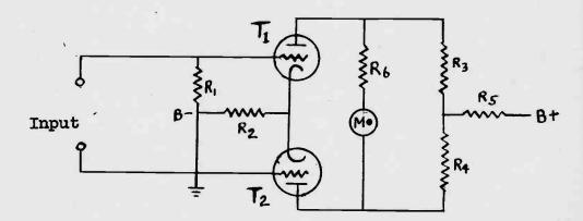
Almost all of the electronic type volt-ohmmeters designed for use by the radio serviceman employ a balanced vacuum tube circuit designed to measure D.C. voltages. To introduce this subject, I will present the basic vacuum tube circuit employed. As you can see in the illustration below, two similar triodes are employed in what, at first, appears to be a peculiar arrangement.
