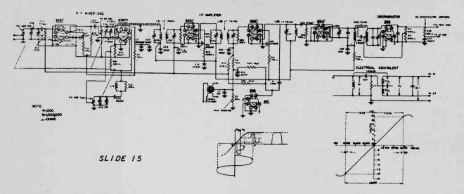
To correct, realign the discriminator transformer primary and secondary trimmers.
