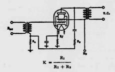
Audio degeneration is obtained by feeding part of the output signal back, in proper relationship, to be exactly out of phase. Due to the effects of reactances in the circuit, exact phase shift is difficult to accomplish in practice. The feedback path may be such as to include several tubes in the circuit, but is usually confined to one or two tubes.
