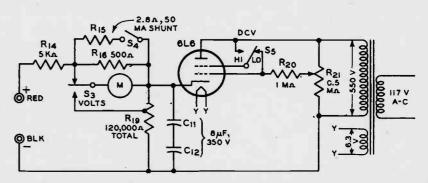
measurements on capacitors rated at 100 volts D.C. working or less, closer control of the test voltage is secured by throwing S5 to connect the rectifier tube screen grid to the control grid instead of the plate (Lo position of switch).
