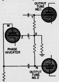
Fig. 3 A partial circuit diagram of the self-balancing type of phase inverter.
