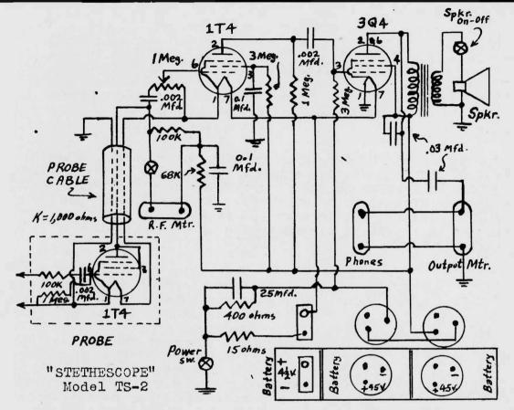
As you progress with the test suggested, the signals should become stronger. Should any of the tests indicate a weakening of the signal, the stage preceding this point is not operating properly and is producing a loss instead of a gain.
