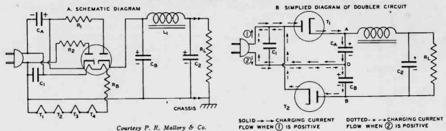
In power supplies of this type, there exists a potential difference between every cathode and heater even if one tube in the set has one filament connection grounded. Any cathode leakage in a tube will create much more trouble in a set using a voltage doubler circuit. You may have to try several tubes for best results and use the unsuitable tubes in a regular type
