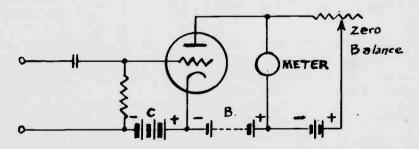
One type of vacuum tube voltmeter (VTVM) employs a vacuum tube (triode or pentode) which is operated over its curved characteristic as a detector. Under such operation, the D.C. plate current will depend on the A.C. voltage applied to the control grid. It is possible, therefore, to calibrate a milliammeter placed in the plate circuit (and which will measure the plate current) in terms of the input grid voltage. The value of plate current present
