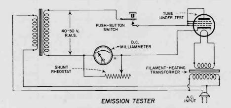
To enable a milliammeter to cover the wide range of current values encountered with the numerous receiving tubes (0.1 to 100 ma.), a shunt rheostat is connected in parallel with this meter. The rheostat must be set to a specific resistance for each type of tube tested. After the power is switched on, readings may be taken by depressing the push-button switch. The latter serves to protect the milliammeter from over-load while the shunt rheostat is being set.
