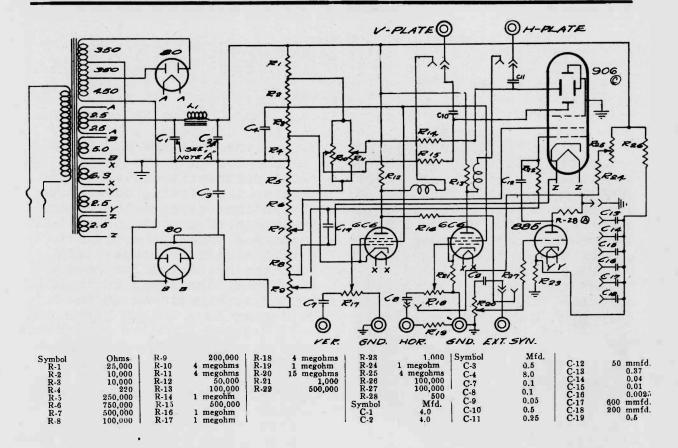
covering from 15 to 30,000 cycles per second and overlapping each other for easy adjustment. Once the band of sweep frequencies, which include the frequency required is selected, the fine frequency control (potentiometer R<sub>25</sub>) is used to achieve the exact adjustment.
