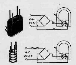
Several diagrams showing the method for connecting a four element bridge of copper oxide discs are shown on the left. These illustrations are reproduced through the courtesy of Weston Electrical Instrument Corp. It is important to realize that the sensitivity of the meter is reduced when a rectifier is used and different scales must be employed for A.C. and D.C. measurements. Any rectifier meter reads average values but is calibrated in terms of R.M.S.
