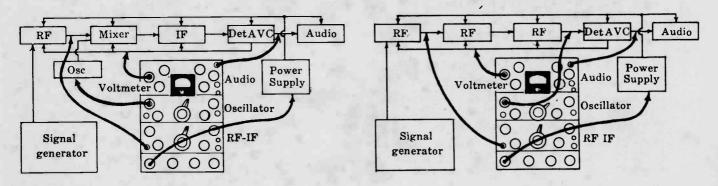
The figure at the left shows a block diagram of a conventional superheterodyne receiver and the points where the various channels of the Analyst are normally connected for the first test on an intermittent receiver. The figure at the right shows, in a similar type of diagram, the most logical places to connect the indicators to a conventional T.R.F. receiver.
