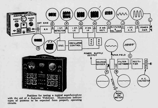
While the majority of signal tracers depend on hearing an audio signal or measuring voltage values, as indicated on a tuning-eye tube or a standard meter, additional information can be supplied by a cathode ray oscilloscope used in conjunction with the signal tracer. In fact, Supreme Instruments have built a visual type signal tracer, which is illustrated below together with a chart showing its application and the type of patterns obtained when a typical receiver is tested at various points.
