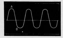
Fig. 6 Distortion of the wave form which results from an improperly balanced phase inverter circuit. The positive peak is of higer amplitude than the negative peak. This condition results in harmonic distortion.
