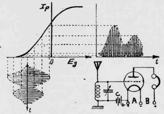
A biased or power detector is operated at that point of its characteristic curve where a much greater plate current change occurs on positive peaks than on the negative peaks.
