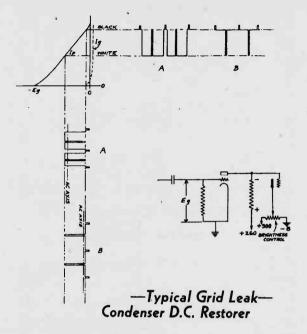
Another method of restoring the D.C. component is by reinserting it in the signal at the grid of the video amplifier tube by operating the tube at zero fixed bias. This method is illustrated at left. The operating bias is then determined by the D.C. drop across the grid resistor caused by the grid current.
