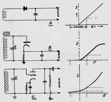
A crystal detector circuit is shown in (A). This detector is essentially linear to the signal in one direction and has infinite resistance to the signal in the opposite direction. In illustration (B) a diode detector is shown. The principle of operation is similar. A power detector, using a self biasing resistor, is shown schematically in (C).
