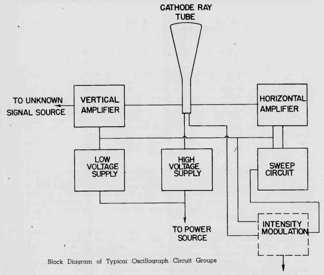
Illustration courtesy Allen B. Du Mont Laboratories, Inc. TIMING SIGNAL
