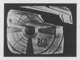
Horizontal Hold Control Incorrectly Set; Two Different Effects.
