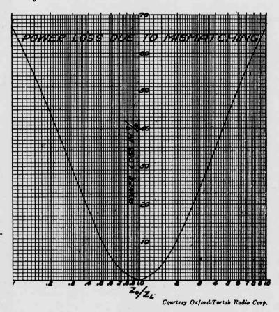
To consider the usefulness of the graph, let us take the problem where the only speaker available is one with a 6 ohm voice coil, and the amplifier output is available in either a 4 ohm or 8 ohm tap. The question in this case is what tap on the amplifier will give the best results. The ratio of
