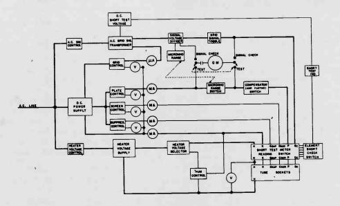
Simplified Block Diagram Of Model 686 Type 9
