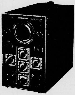
The illustration of this instrument will suggest to you the physical position of the various controls, which are also indicated in the schematic diagram. The intensity control varies the brilliance of the spot. Usually this control also has the on-off switch. The focus control is used to adjust the resulting picture to a bright image and is dependent on the adjustment of anode voltages for proper electron-optical focus.
