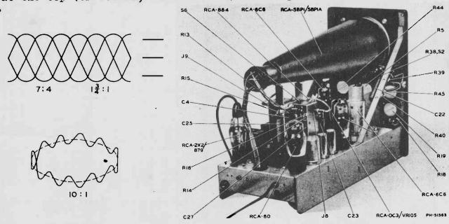
For the study of ratios greater than 10 to 1, the wave form is produced on a circle or ellipse. A phase splitting circuit consisting of a condenser across one set of deflecting plates and a resistor across the other plates will displace the pattern around the ellipse for easy analysis.
