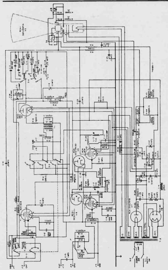
lecture we include the circuit diagram and type R.C.A. Model 160-B oscilloscope. To complete this other data on a 5 inch
