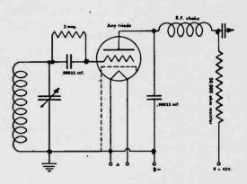
A grid leak detector is especially useful in circuits requiring considerable sensitivity. It is not used in modern radio sets.
