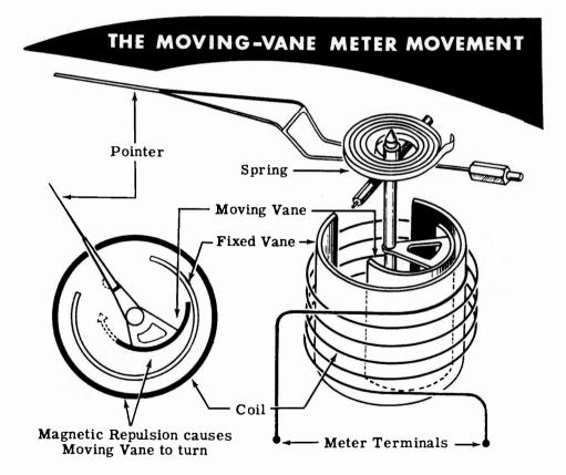
Moving-vane meters may be used for voltmeters, in which case the field coil consists of many turns of fine wire which generate a strong field with only a small current flow. Ammeters of this type use fewer turns of a heavier wire, and depend on the larger current flow to obtain a strong field. These meters are generally calibrated at 60 cycles AC, but may be used at other AC frequencies. By changing the meter scale calibration, movingvane meters will measure DC current and voltage.
