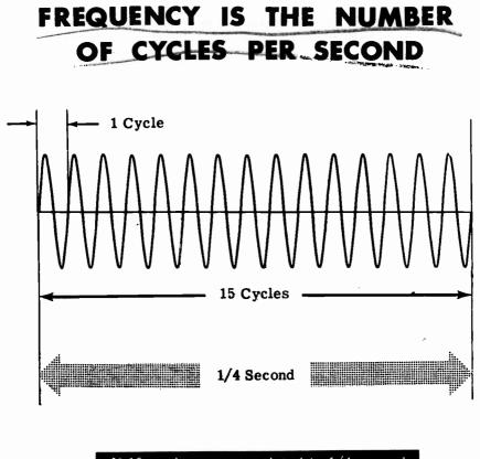
If 15 cycles are completed in 1/4 second, the frequency is 60 cycles per second.
