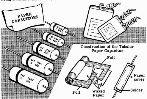
Some types of paper capacitors are encased in a mold of very hard plastic. Capacitors which are so constructed are very rugged and may be used over a much wider temperature range than the cardboard case type, since the wax used in the tubular cardboard type melts at high temperatures and escapes through the open ends of the cardboard case.
