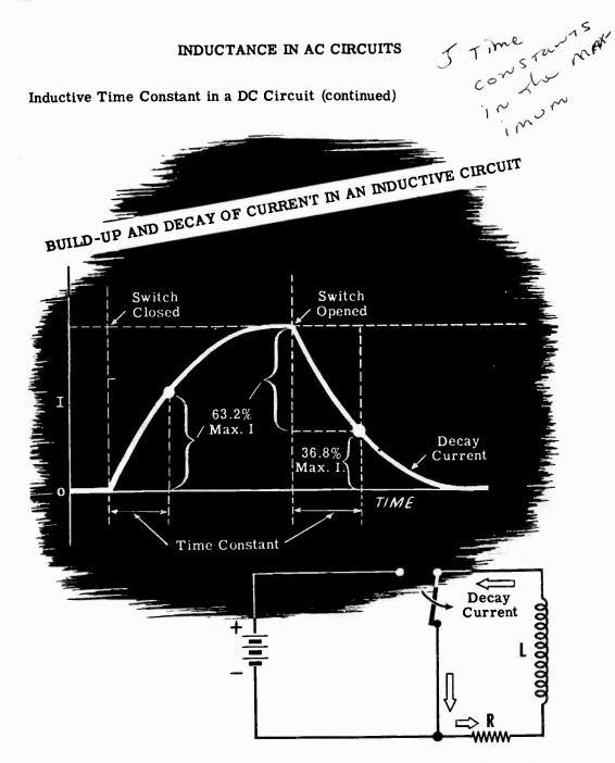
If the coil terminals are shorted together at the same moment that the battery switch is opened, the coil current continues to flow due to the action of the collapsing field. The current falls in the same manner as the original rise in current, except that the curve is in the opposite direction.
