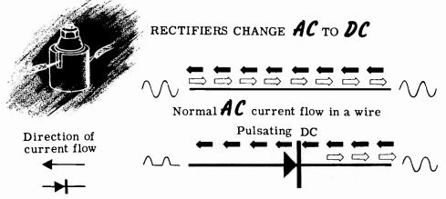
Rectifier allows current flow in one direction only
