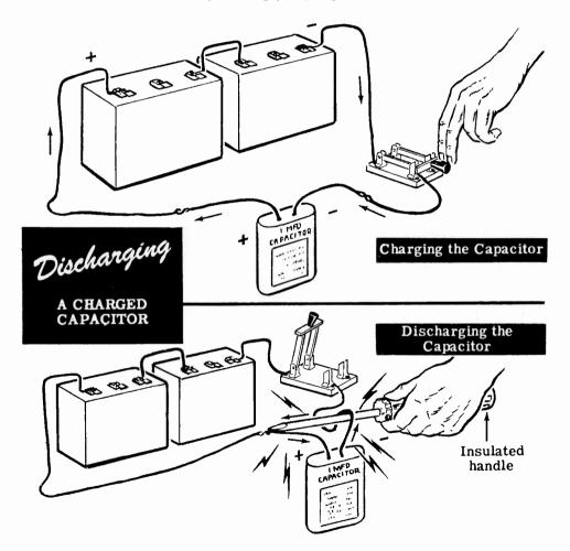
As the instructor repeatedly charges and discharges the capacitor, you see that the resulting arc is the same each time. This shows that the charge left in a capacitor when the circuit voltage is removed is always maximum in a DC circuit. <u>CAUTION</u>: Never discharge a capacitor while it is connected to the circuit voltage, whether the voltage source is a battery or AC power line.
