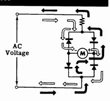
Because the meter reading is the average of the half-cycle current pulses, the scale is not the same as that used for DC. Although the amount of deflection is a result of average current flow through the meter movement, the scale is calibrated to read effective values of voltage.
