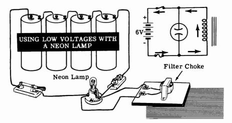
As the switch is opened you see that the lamp flashes, indicating that the voltage across the lamp and coil in parallel is higher than the starting voltage required for the lamp. This voltage is the induced emf generated by the collapsing field of the choke, and is a visible effect of inductance.
