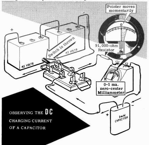
Demonstration—Current Flow in a DC Capacitive Circuit (continued)
