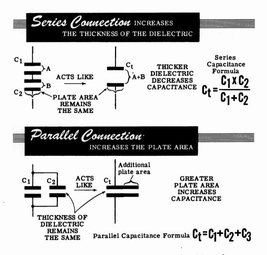
When resistors are connected in parallel, the total resistance decreases since the cross section through which current can flow increases. The reverse is true of parallel-connected capacitors. The total capacitance increases, since the plate area receiving a charge increases. The total capacitance for parallel-connected capacitors is found by adding the values of the various capacitors connected in parallel.
