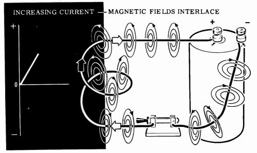
The lines of force around each turn continue their expansion and, in so doing, cut across adjacent turns of the coil. This expansion continues as long as the circuit current is increasing, with more and more lines of force from the coil turns cutting across adjacent turns of the coil.
