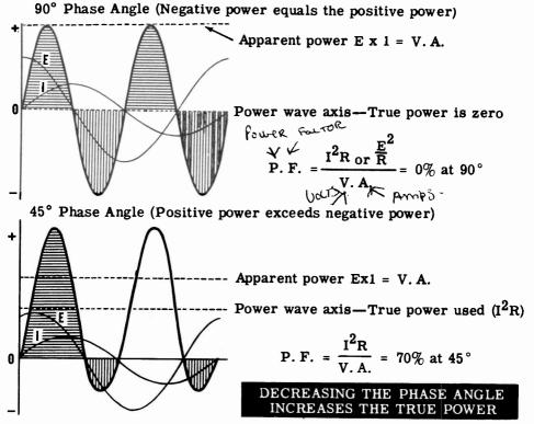
The average value of actual power, called "true power," is represented by an axis drawn through the power wave halfway between the opposite maximum values of the wave. As the phase angle increases, this axis moves nearer to the axis for voltage and current. In AC circuits the apparent power is found by multiplying the voltage and current just as in DC circuits (Apparent power = Voltage x Current). When apparent power is divided into true power, the resultant decimal is the power factor.
