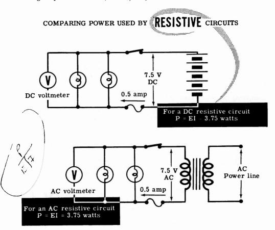
Next the battery is disconnected and the DC voltmeter is replaced with an AC meter of the same range. The 6.3-volt transformer is used as an AC voltage source, and you see that the lamps light as brightly as they did in the DC circuit. Notice that the voltmeter reading is almost the same as that obtained using DC, about 7.5 volts.
