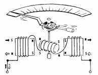
HOT-WIRE AMMETER — Meter movement based on the expansion of a wire heated by current flow through it. Used only to measure current.
