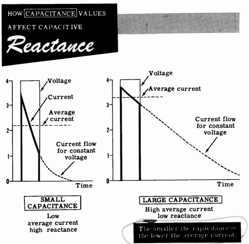
The current flow in a capacitive circuit, assuming that there is no change in the resistance, increases with an increase in either frequency or capacitance. Then capacitive reactance—the opposition to current flow through a capacitance—must decrease when the frequency or capacitance
