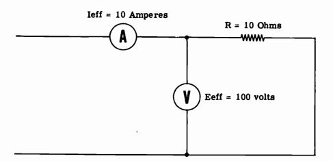
$I^2R \text{ or } E^2/R = \text{Eeff x Ieff}$   $I^2R \text{ or } E^2/R = \text{Watts}$ Power Factor =  $\frac{I^2R}{\text{Ieff x Eeff}} \text{ or } \frac{E^2/R}{\text{Ieff x Eeff}} = \frac{1000}{1000} = 1. \text{ or } 100\%$ Power Factor =  $\frac{\text{Watts}}{\text{Volt-Amperes}}$
