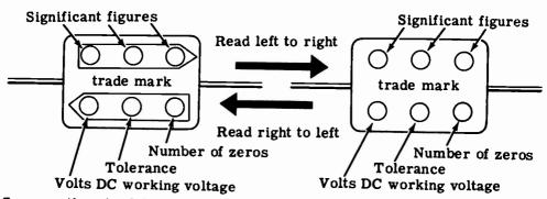
Suppose the six dots read in the correct order are brown, orange, green, red, silver and blue. The capacitor then has a capacitance of 13,500 mmf, a tolerance of 10 percent and a voltage rating of 600 volts.
