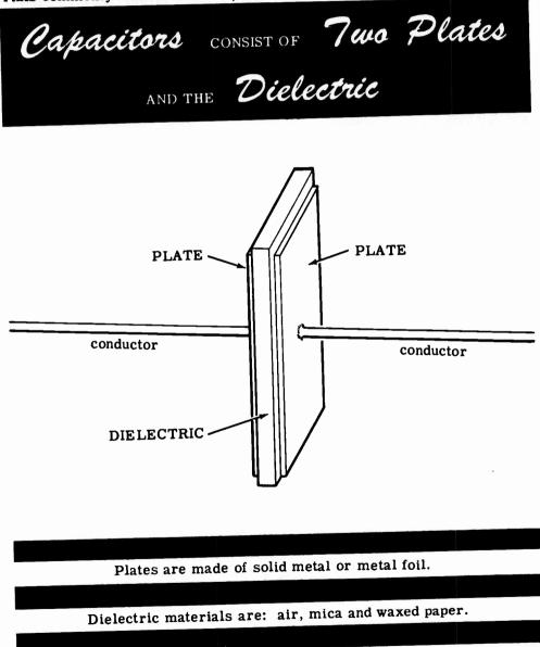
Three basic factors influence the capacity of a capacitor or condenserthe area of the plates, the distance between the plates (thickness of the dielectric) and the material used for the dielectric.
