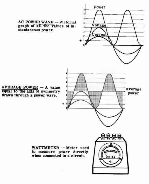
Remember that the power formula (P = EI) can be used to find the power used in a resistive AC circuit, provided effective values of E and I are used.
