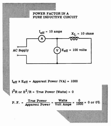
Power Factor is a method of determining what percentage of the supplied power is used in watts, and what percentage is returned to the source as wattless power.
