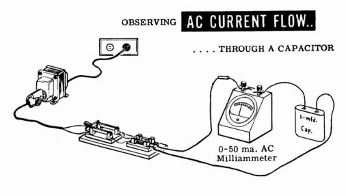
To prove that capacitors appear to block DC but permit AC to pass, the instructor sets up the circuit shown to the right. When DC is applied the lamp will not glow and a DC voltmeter across the lamp will read zero volts. When AC is applied the lamp will glow and an AC voltmeter across the lamp will give a reading.
