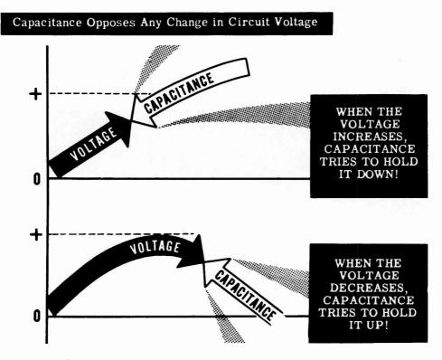
Because DC voltage usually varies only when it is turned on and off, capacitance affects DC circuits only at these times. In AC circuits, however, the voltage is continuously changing, so that the effect of capacitance is continuous. The amount of capacitance present in a circuit depends on the physical construction of the circuit and the electrical devices used. The capacitance may be so small that its effect on circuit voltage is neglibible.
