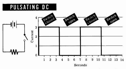
Waveforms of voltage and current are not always made of straight lines connecting points. In most cases waveforms are curved, representing gradual changes in voltage and current. This is particularly true of pulsating DC waveforms.
