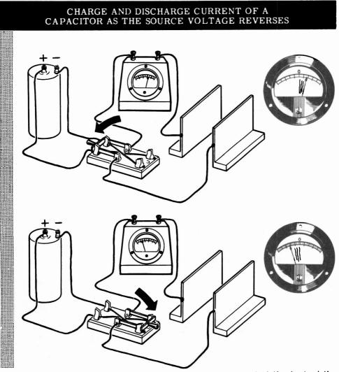
Suppose you switch the cell polarity fast enough so that at the instant the condenser plates become charged in one polarity, the cell polarity is reversed. The meter needle now moves continuously—first showing a current flow in one direction, then in the opposite direction. While no electrons move through the air from one plate to the other, the meter shows that current is continuously flowing to and from the condenser plates.
