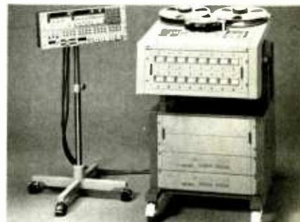
Amplifiers are all direct-coupled for lowest distortion and optimum LF response. Improved transient response and phase characteristics are obtained with the MS-16's first-stage sync and replay head amplifiers, which use differential paired, ultra-low-noise FETs. The multitrack also has separate low-frequency compensation alignment for record/sync and repro heads, plus both +4 dBm balanced XLR and -10 dBV unbalanced RCA output.
