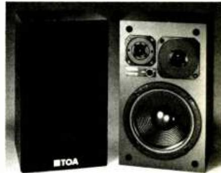
The two-way 265-ME is said to be ideal for either primary or secondary reference applications, and handles continuous program at 75 WRMS. Response is a quoted 60 Hz to 20 kHz. Components comprise a 6.3-inch woofer, and a 1.2-inch soft dome tweeter with diffuser.
