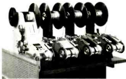
A digital counter on the control module provides the user with the number of tapes recorded per slave, and the machine will stop automatically when the preset number of passes has been reached.
