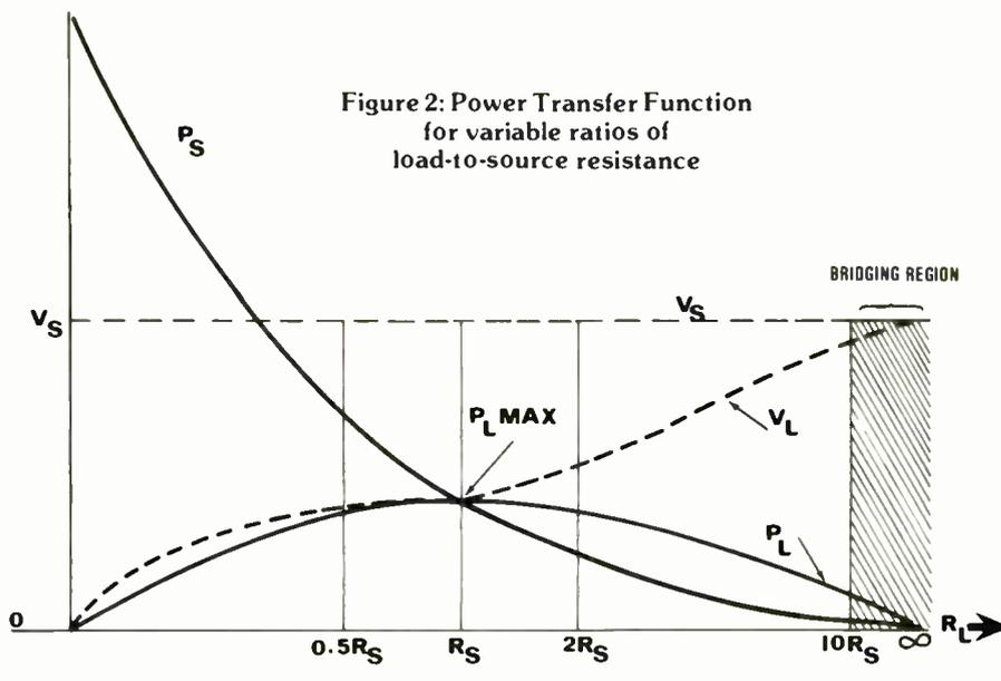
Figure 2: Power Transfer Function for variable ratios of load-to-source resistance
