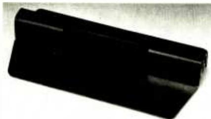
Capable of withstanding up to 120 dB SPL without distorting, the electret condenser capsule provides a quoted frequency response from 50 Hz to 18 kHz; sensitivity is -52 dB re: 1 volt per microbar and self-noise less than 22 dBA. Output impedance is 150 ohms, balanced.
