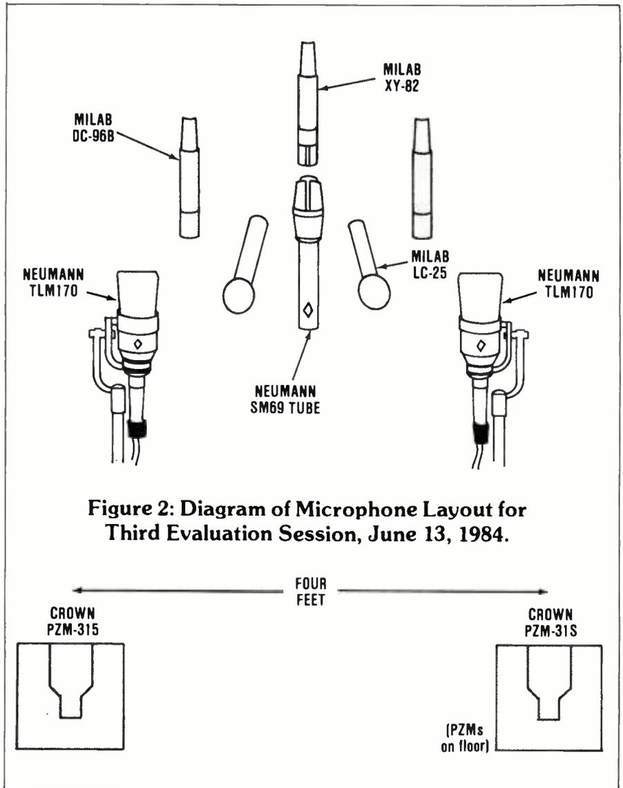
Figure 2: Diagram of Microphone Layout for Third Evaluation Session, June 13, 1984.
