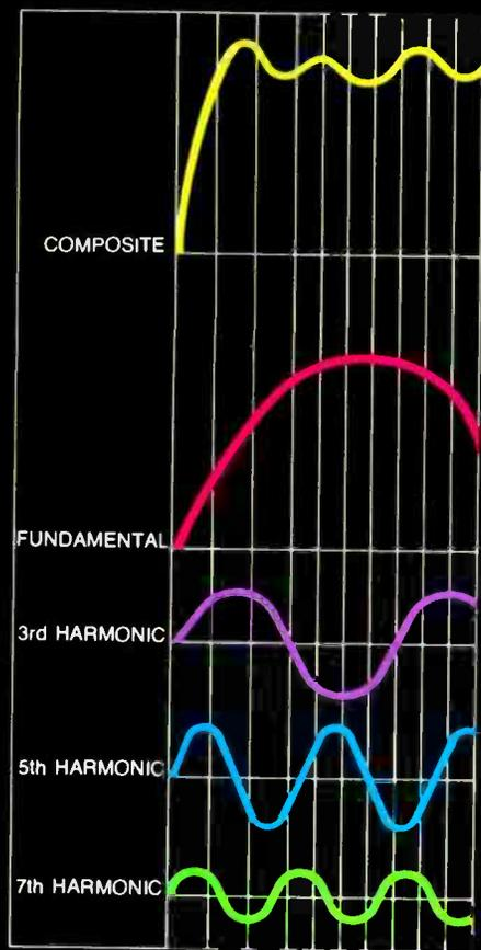
The completed figure to the left is a composite illustration of how a transient pulse looks when the fundamental, 3rd, 5th, and 7th harmonics are all in phase.
