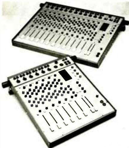
The microphone/line input switch on each input channel selects either a low or high impedance input. Both are electronically balanced, and together cover the range -55 to +10 dBm, with 25 dBm overload margin. Three-band EQ offers  $\pm 15$  dB of midrange sweep control from 330 Hz to 6.5 kHz.
