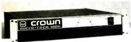
Hum and noise are a quoted 105 dB below rated output (A-weighted), harmonic distortion less than 0.05% from 20 Hz to 1 kHz, and increasing linearly to 0.1% at 20 kHz, delivering 250 watts into 8 ohms, per channel; IM distortion is less than 0.05%, and slewing rate greater than 13 volts per microsecond.
