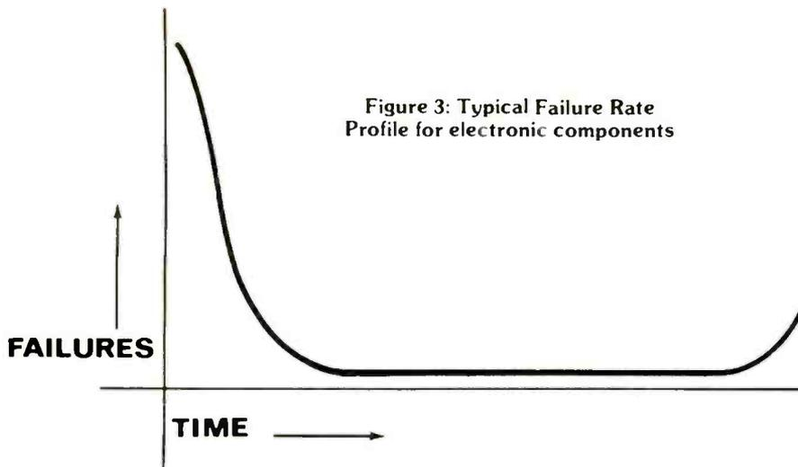
Figure 3: Typical Failure Rate Profile for electronic components
