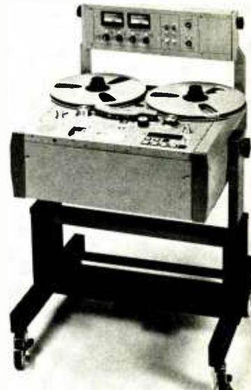
Other features include: extensive user programmable functions for both transport and electronics; an integral four-point search-to-cue, RTZ and Search-start, ±45% variable speed; direct-coupled active balanced I/O; cue speaker and headphone amp; tape time/speed display; a cue shuttle level, and a controlled wind "library pack" mode.
