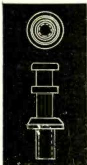
It's as simple as that with these heavily silver plated C. T. C. Turret Terminal Lugs. Quick soldering, too. Sufficient metal is used to give them strength but there's no surplus metal to draw heat and increase soldering time.
