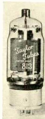
Electrical characteristics: Filament (thoriated tungsten) voltage—10 volts a-c or d-c at 5 amperes; transconductance for plate current of 50 ma is approximately 3750 umhos; interelectrode capacitances—grid to plate (with external shield)—0.2 (max.) mmf, input—16.3 mmf, output—14 mmf.
