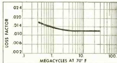
Based on Power Factor Measurements made by Bonton Radio Corp. on standard Mykroy stock.
