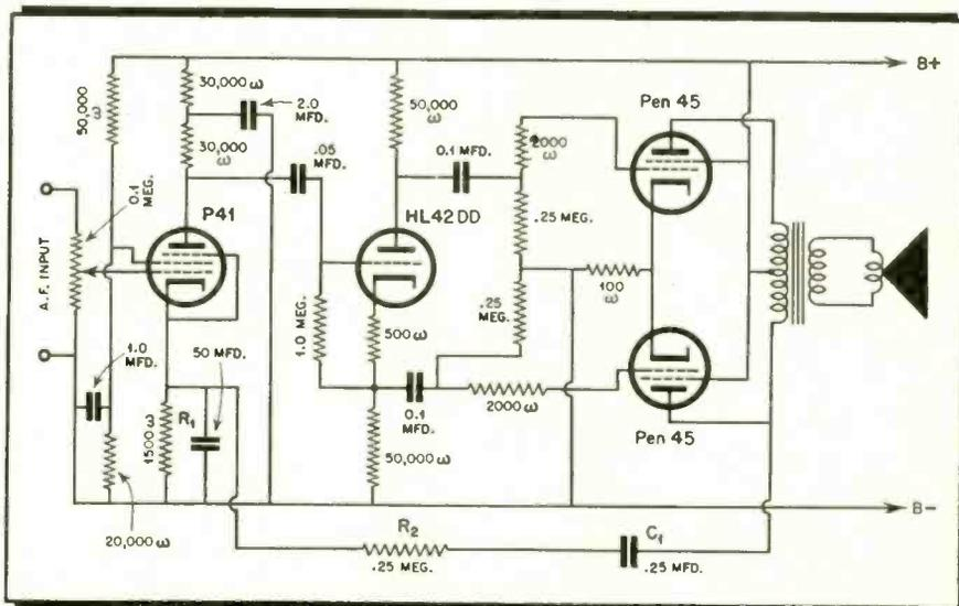
Fig. 4 Negative feedback amplifier
