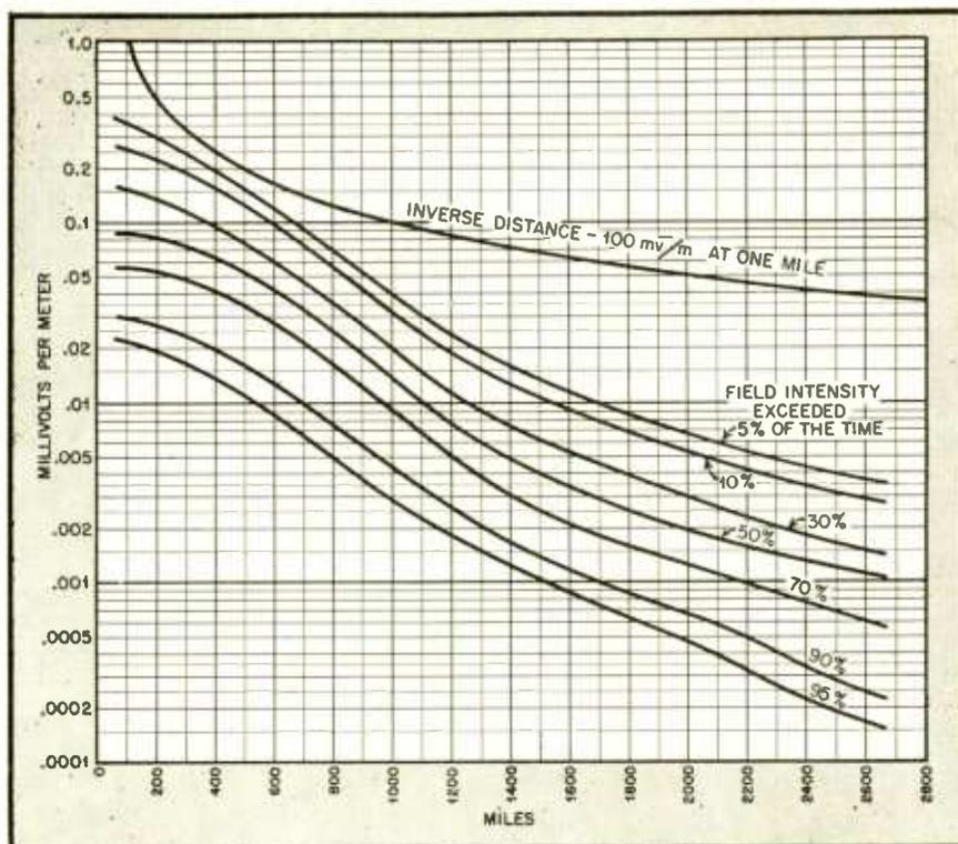
Fig. 5 Propagation curves of sky wave
