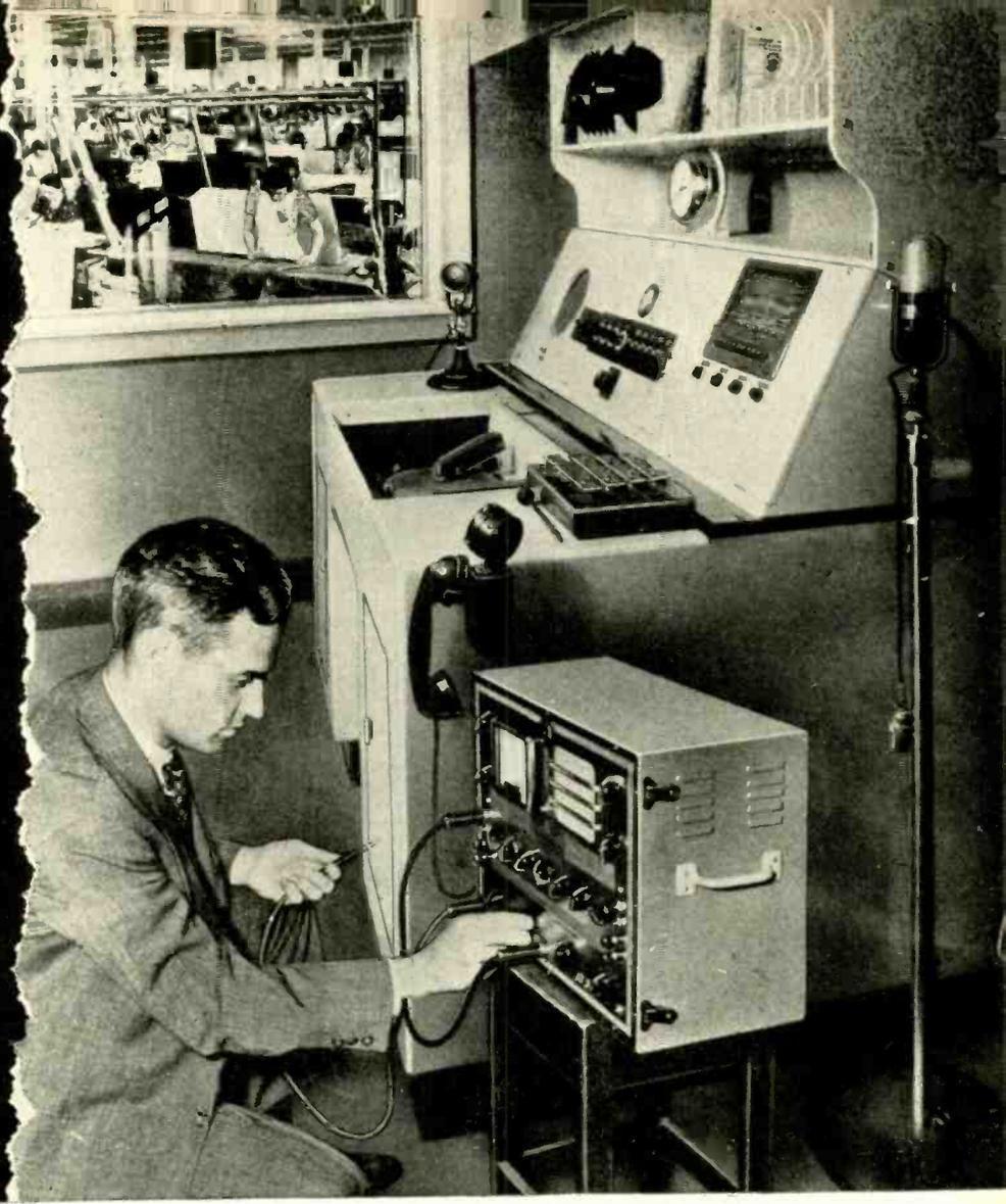
**T**HE new 170-A Audio Chanalyst is a combination testing unit which includes the famous Voltohmyst circuit, a new diode flat through the audio range, a B.F.O. signal source, a gain calibrated amplifier, and speaker and line output connections.
