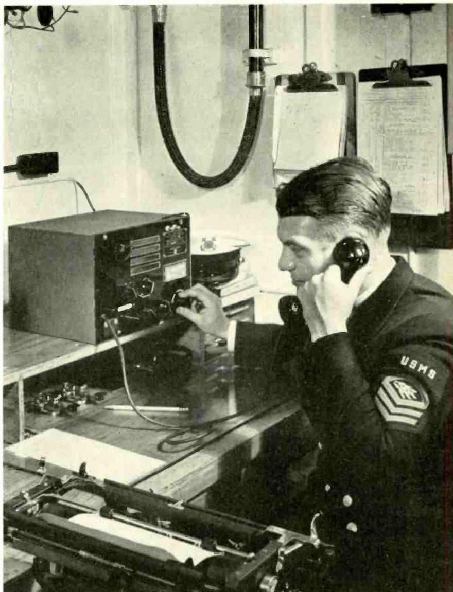
The yachtman's telephone has gone to war. The midget Western Electric 8 watt radio transmitter and receiver which formerly enabled the small boat owner to keep in communication with the Coast Guard, land telephone system and with other radio-equipped vessels, is shown above installed aboard a Merchant Marine training ship.
