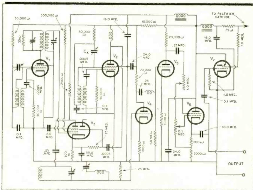
Fig. 5 Audio frequency oscillator
