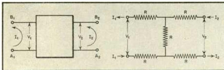
such thing as a telephone transmission line, a transformer, or even a pair of radio antennas located some distance apart. If the input terminals which are called  $A_1$  and  $B_1$  have a current  $I_1$  flowing in  $A_1$  and out  $B_1$ , and if the output terminals,  $A_2$  and  $B_2$  have a current  $I_2$  flowing in  $B_2$  and out  $A_2$  (see figure) then the transducer is said to be a linear transducer if
