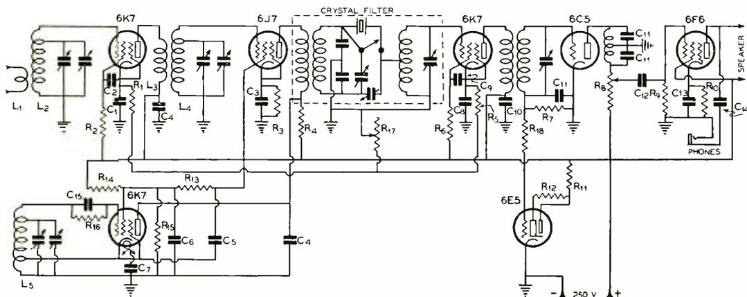
The Bandsread Special 20 Meter Phone Receiver Wiring Diagram
