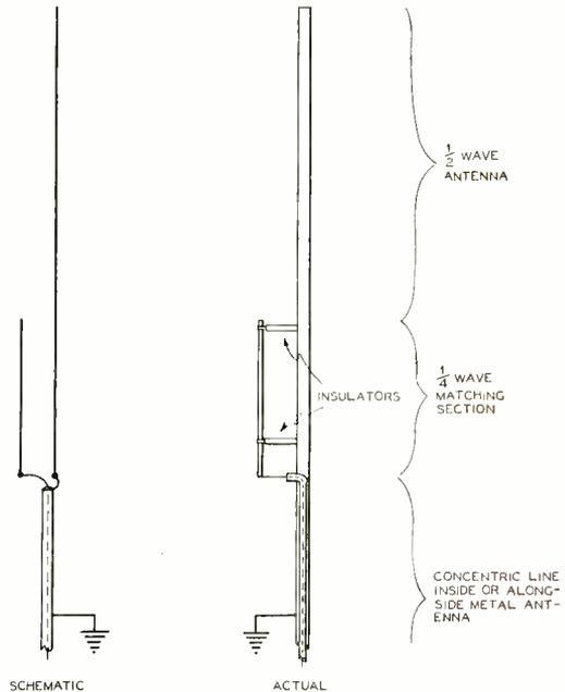
One method used to match a low-impedance line to an end-fed antenna with a matching section.
