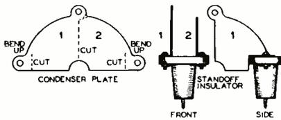
A very inexpensive neutralizer for 35-T's, RK35-37, 834, T-55, etc., can be made from a Johnson no. 24 stand-off insulator and one stator plate robbed from a National type DX condenser. Capacity is varied by rotating one plate. Directions: Cut, bend, mount, use.
