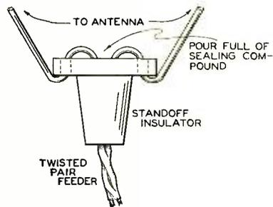
sizes, a suitable size being chosen for the particular feed line to be used. I used a Birnbach type 866-SJ with the hardware removed. After all connections are made, the insulator is poured full of sealing compound. This prevents moisture from getting into the crotch of the transmission line.—W9NBE.
