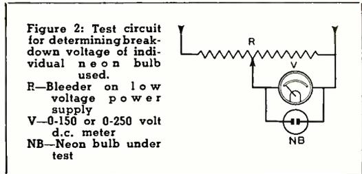
Figure 2: Test circuit for determining breakdown voltage of individual neon bulb used.
