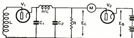
Figure 2: Simplified Schematic of Modulation Monitor
