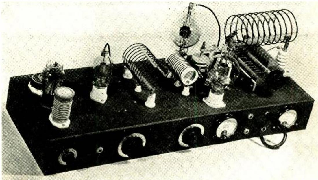
Looking down on the transmitter. The small flashlight bulb connected in series with the crystal is hiding behind the 6L6-G. It is screwed into a small hole in the Masonite and connections soldered to it.
