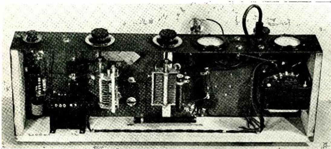
The under side of the chassis. The filament transformers are mounted directly on the chassis to keep the leads short and reduce voltage drop. No. 10 enamelled copper wire should be used for all tank circuit leads and for filament leads to the 100-TH's.
