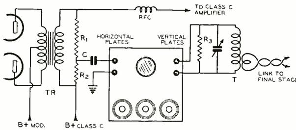
Figure 2: Connections for Trapezoidal Patterns
