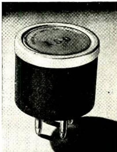
Clarostat Mfg. Co., Inc. These plug-in resistors were originally developed for use in resistance bridges and other test equipment employed in the Clarostat laboratory and plant. Housed in a standard 4-prong tube base, these units are available in values of 1 to 10,000 ohms, with any accuracy up to  $\frac{1}{10}$ th of 1 per cent. Due to the design, they are quite inexpensive.
