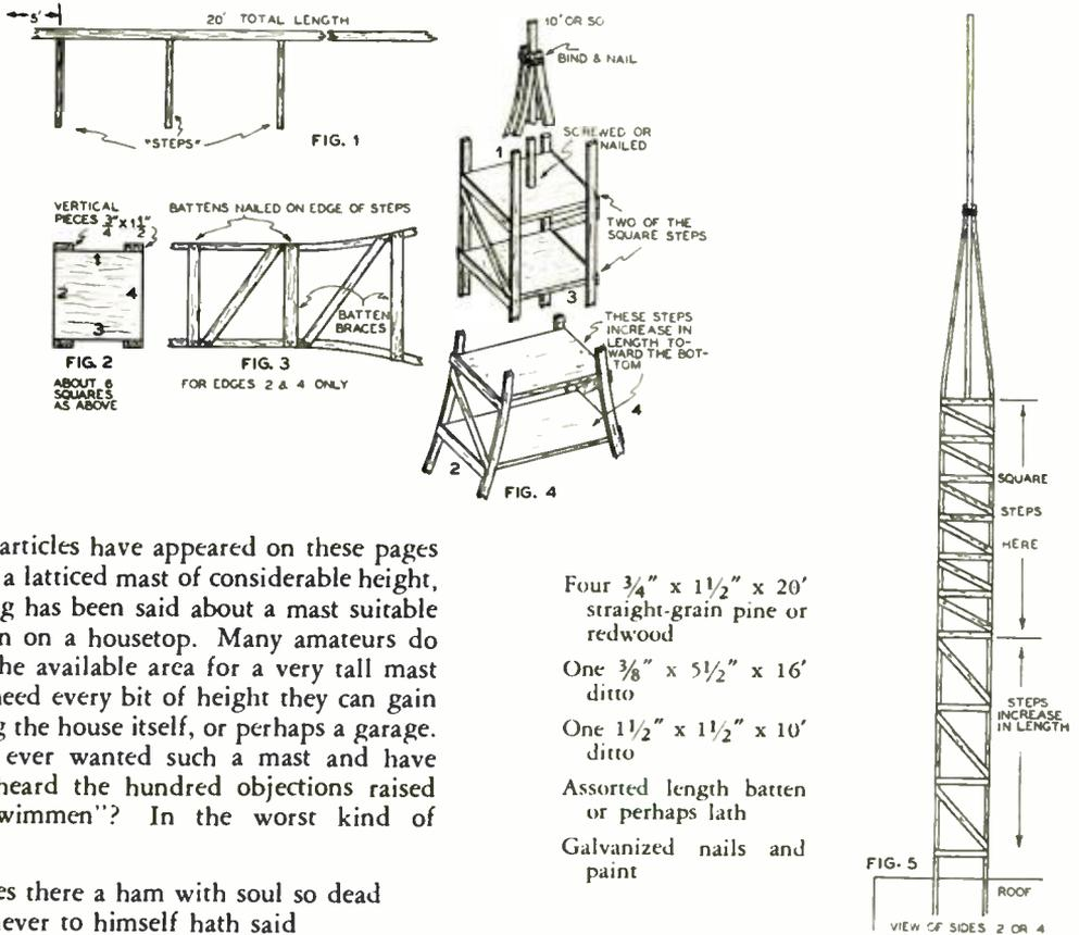
Several articles have appeared on these pages describing a latticed mast of considerable height, but nothing has been said about a mast suitable for erection on a housetop. Many amateurs do not have the available area for a very tall mast and thus need every bit of height they can gain by utilizing the house itself, or perhaps a garage. Have you ever wanted such a mast and have you ever heard the hundred objections raised by the "wimmen"? In the worst kind of rhyme . . .
