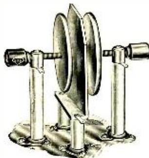
Bud ultra-high frequency condensers are constructed of aluminum plates with highly polished surfaces. The two round plates are 2 3/16" in diameter and 3/16" thick,
