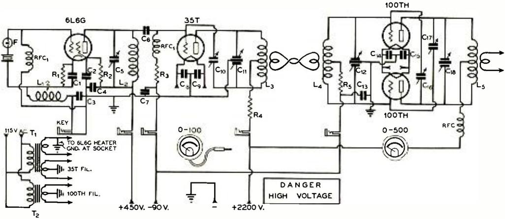
General Wiring Diagram of the 100-TH Transmitter
