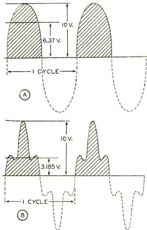
Figure 5: Audio Waveform to Meter
