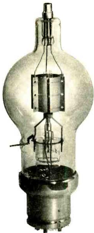
At any plate voltage and at any frequency the 250TL and 250TH tubes provide an economical answer to the problem of obtaining high power.
