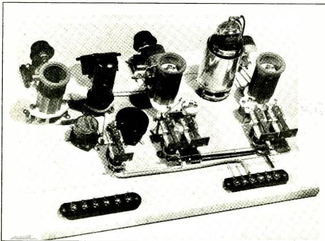
The QRQ-QSY exciter used at W4DHz. QSYing is done remotely with a single switch by means of relays and padding condensers in the tank circuits.
