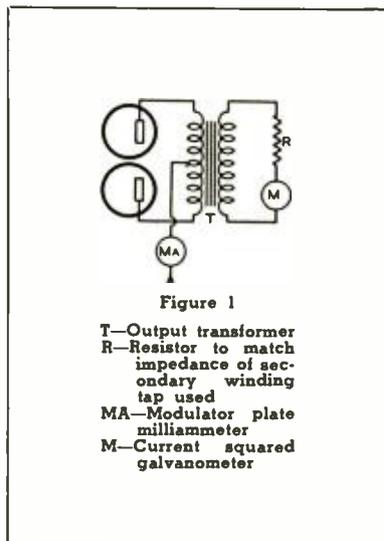
the plate current on the tubes reaches the rated value or until further increase in the gain gives no increase in output. The output power can then easily be calculated from equation (5) or (6).
