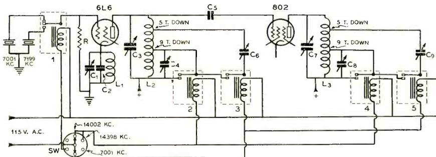
Wiring Diagram of the Exciter, QSY Portion Only
