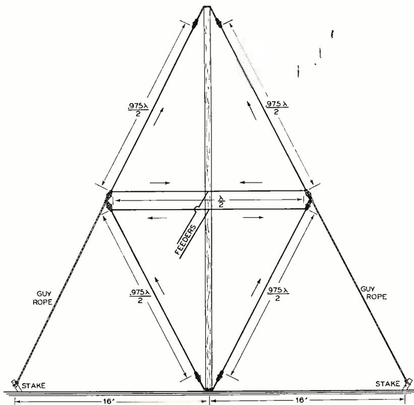
Figure 4: The Array Requires But One Pole, and Is Easily Rotated
