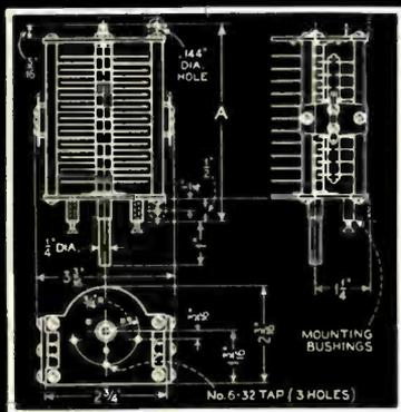
A NEW popular series of transmitting condensers for high frequency and ultra-high frequency medium and low powered units. The construction of these condensers is so rugged that even rough handling will not damage them. Though low in price, these condensers include all constructional features necessary in quality transmitters of all kinds. High operating efficiency has been attained by extensive research in materials and design plus careful workmanship.
