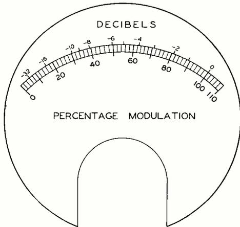
Figure 9: Scale Layout of the Indicating Meter
