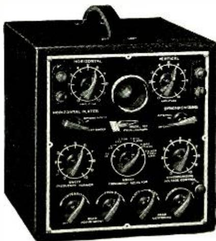
Notwithstanding these advantages, the model 105 is offered for about one-half former oscillograph prices. It is supplied complete with tubes for direct operation from 110 volts, 60 cycle power supply. Special models for other voltages and currents are available.
