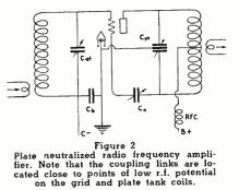
in d.c. grid current. When the amplifier is perfectly neutralized there will be no change in d.c. grid current when the plate tank condenser is tuned across resonance. The amplifiers shown utilize link coupling but the procedure is exactly the same for any coupling method.
