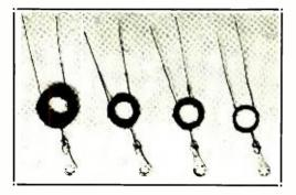
Balance Coils for 20, 40, 80, and 160 Meter Bands
