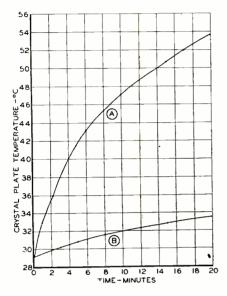
Figure 1 Temperature increase with and without the cooling system described in the text. Curve "A" is for conventional mounting, curve "B" with holder mounted upside down on chassis.
