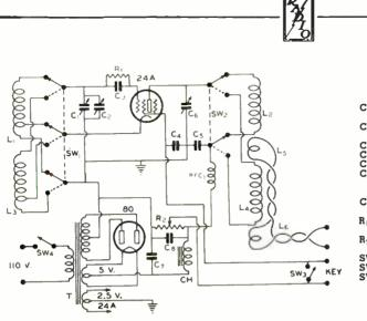
capacity to ground around the bulb in the vicinity of the plates. Consequently, a wide strip of aluminum was bent so that in addition to serving as the capacity to ground it serves as a means of mounting the bulb to the shield can. The rest of the construction is quite ordinary and becomes self-explanatory through the circuit diagram and photographs.
