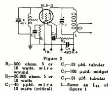
of figure 1 does not depend upon the cathode coil for oscillation, as evidenced by the fact that it may be shorted out and the circuit will still work, though with low efficiency on the harmonics (see figure 2). In spite of improved performance over the tritet to which it is distantly related (both being descendents of the Dow oscillator), the exciter of figure 1 actually has fewer components.
