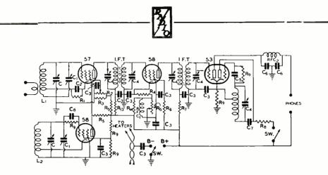
General Wiring Diagram of the Inexpensive Superhet
