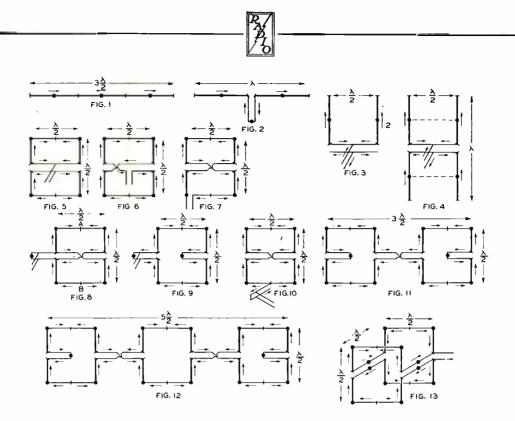
tained by *adding* the gain in db of the components. Five db represents a power ratio of 3.2 times. Thus the structure of figure 4 makes 100 watts sound like 320 watts in the favored direction.
