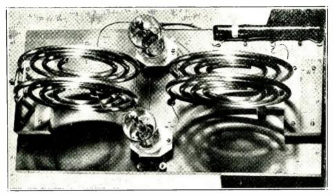
Highly efficient tank circuits in a five-meter oscillator, coiled to permit compact construction
