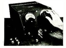
The QX-Checker is a companion instrument of the Q-meter in general use in well-equipped laboratories and engineering departments. This new instrument is intended for use by the production staff, and is set to given tolerances within which must come pro-
