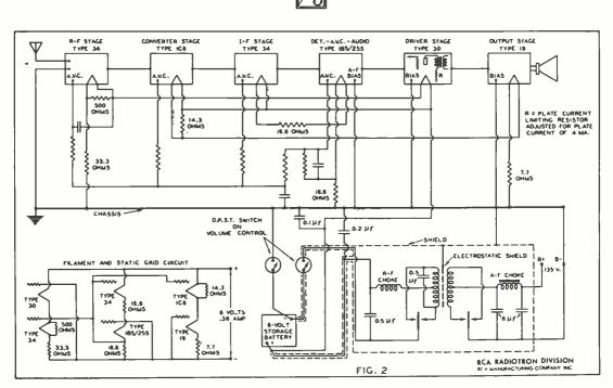
ceiver be run to that point if decently possible, so that there will not be couplings due to circulating currents in the receiver chassis. Incidentally, shields want to be shields in any case, not return-circuits. This holds for the metal cases of receiver and of B unit, also for the cables between them and from the storage battery. In some R.C.A. laboratory tests the soundness of these warnings was shown as follows:
