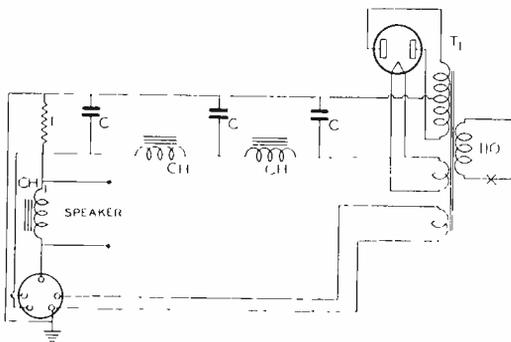
Wiring Diagram of the Power Supply
