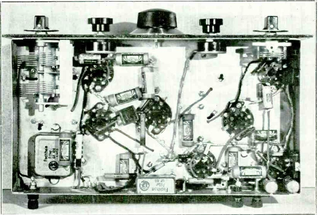
Bottom View of the Receiver. Note the Shielded Wire Used for the "Hot" Filament Lead. The Carbon Resistors Are the New Insulated Type.
