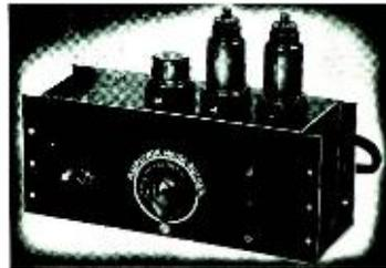
the Amplivox Radio and Sound Labs., and is known as the "Amplivox Noise Bucker". It is attached to most any standard superheterodyne with two or more stages of i.f. by making a few simple connections.
