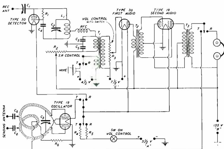
The "Transceptor" Wiring Diagram
