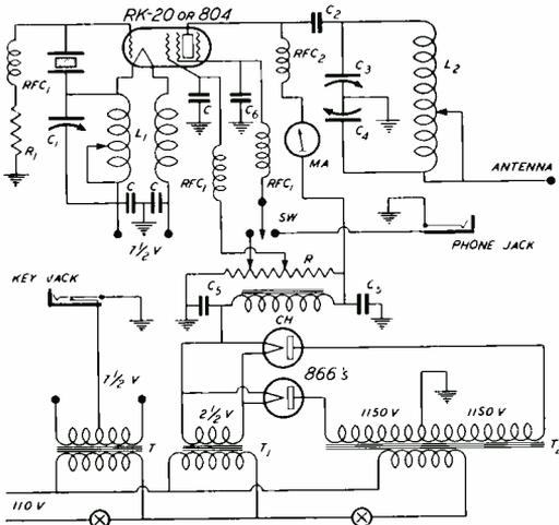
**Wiring Diagram of the Portable Tritet**
