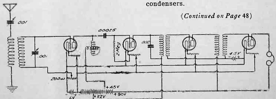
Fig. 1. Circuit for Tuned Plate Receiver.
