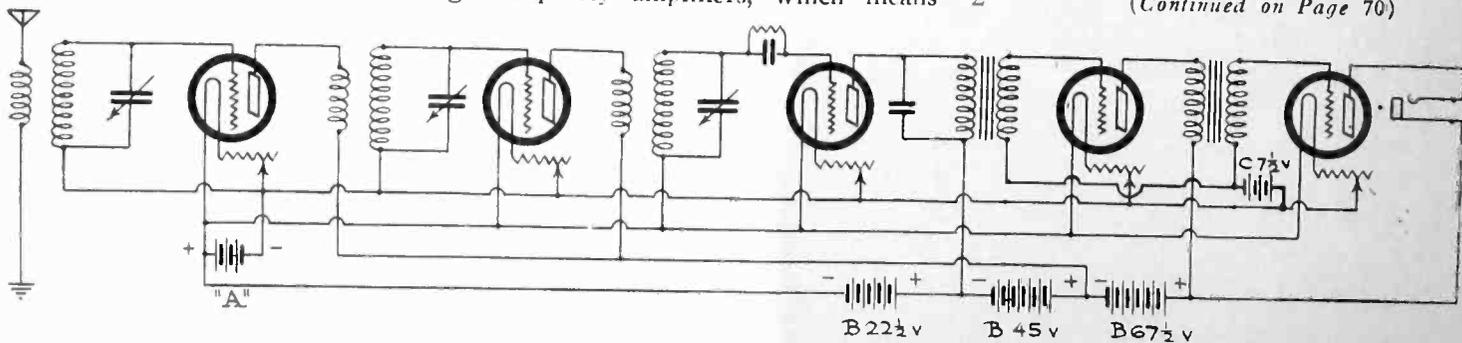
Fig. 6. Two Stages R.F., Detector and Two Stages A.F.
