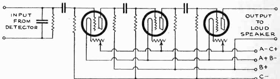
Fig. 11. Resistance Coupled A.F. Amplification.
