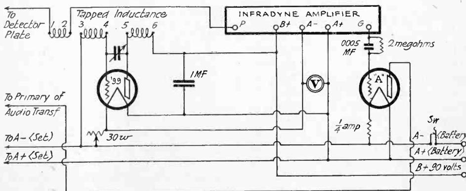
Fig. 1. Circuit Diagram for Infradyne Adapter.
