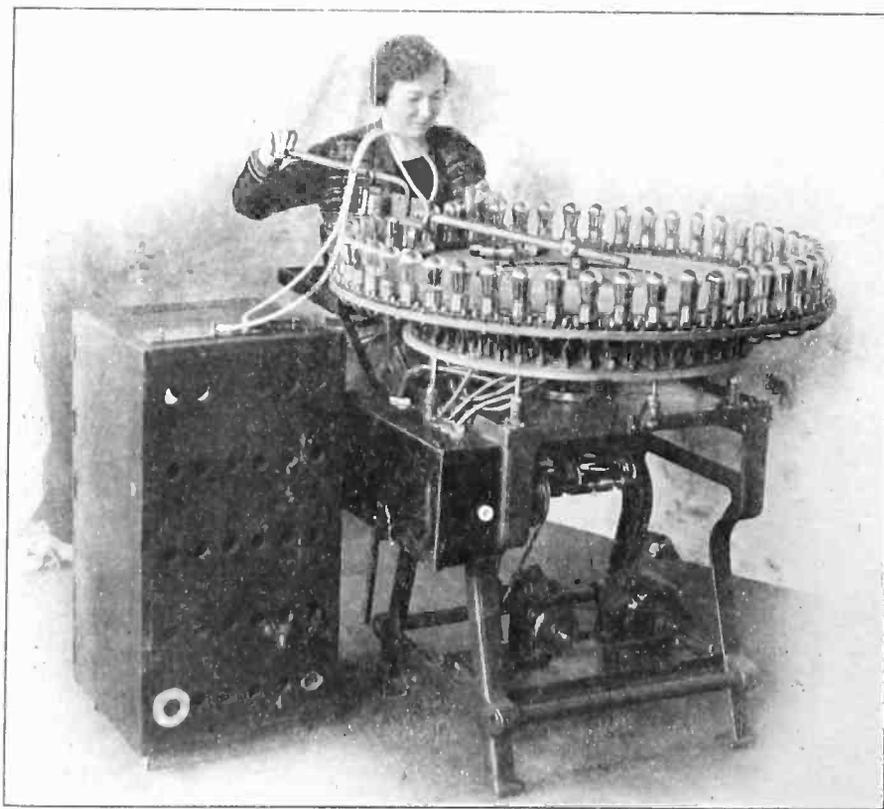
*A Laboratory-Created Tube Ager and Bombarter Which Has Helped to Reduce the Manufacturing Cost of a 201A Tube to 28 Cents.*
