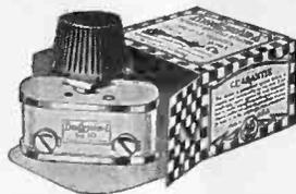
Bradleyohm-E is a new and enlarged Bradleyohm designed especially for B-Eliminator Voltage Control. The extra long columns of scientifically-treated graphite discs insure perfect voltage control over a wide range. It is made in several ranges for various B-Eliminator circuits.
