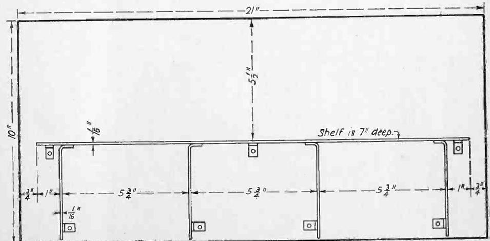
Fig. 3. Assembly for Shielding.
