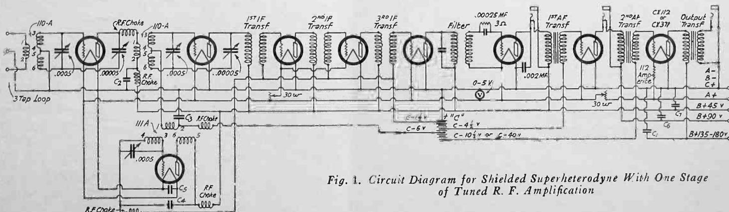
Fig. 1. Circuit Diagram for Shielded Superheterodyne With One Stage of Tuned R. F. Amplification
