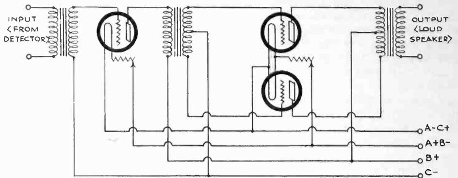
Fig. 10. Push-Pull A.F. Amplification.
