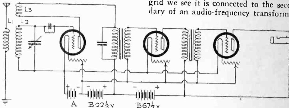
Fig. 5. Regenerative Circuit with Two Stages A.F. Amplification.
