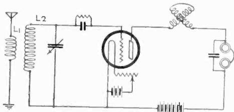
Fig. 4. Tuned Plate Regenerative Circuit.
