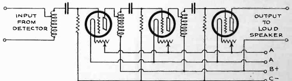
Fig. 12. Impedance Coupled Amplifier.
