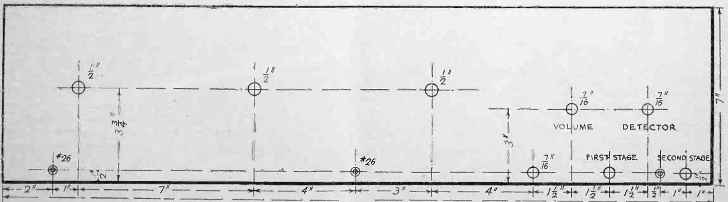
Fig. 3. Panel Drilling Template.
