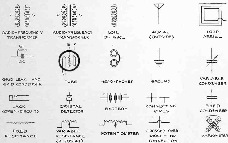
Fig. 1. Conventional Symbols Used in Radio Diagrams.
