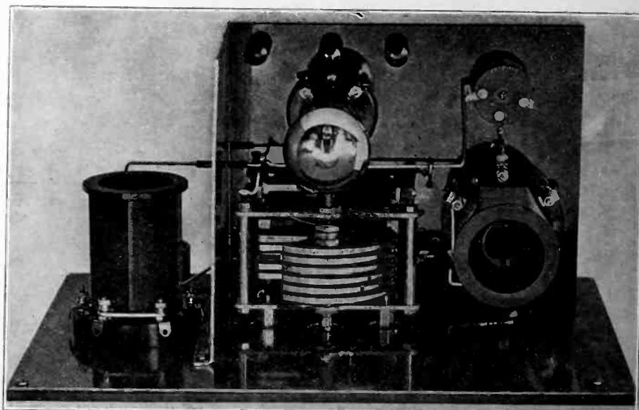
Amplifier Assembly, With Shield in Place.
