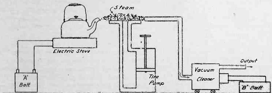
Fig. 1. Mechanical Illustration of Vacuum Tube Action.
