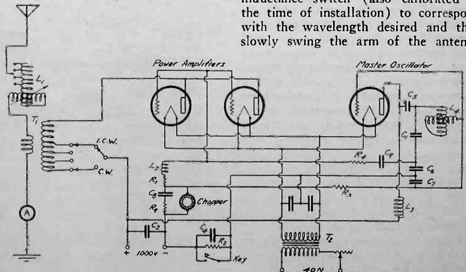
Diagram of Connections of Type ET 3627-A 200-Watt Vacuum Tube Marine Radio Transmitter.
