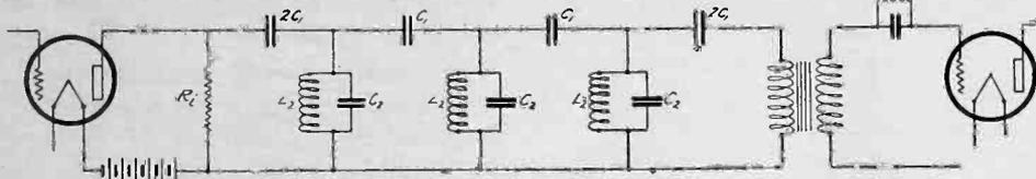
Fig. 3. Actual Arrangement of Elements in Filter.
