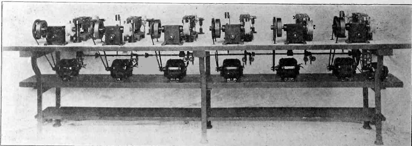
A Battery of Tungsten Filament Wire-Drawing Machines.
