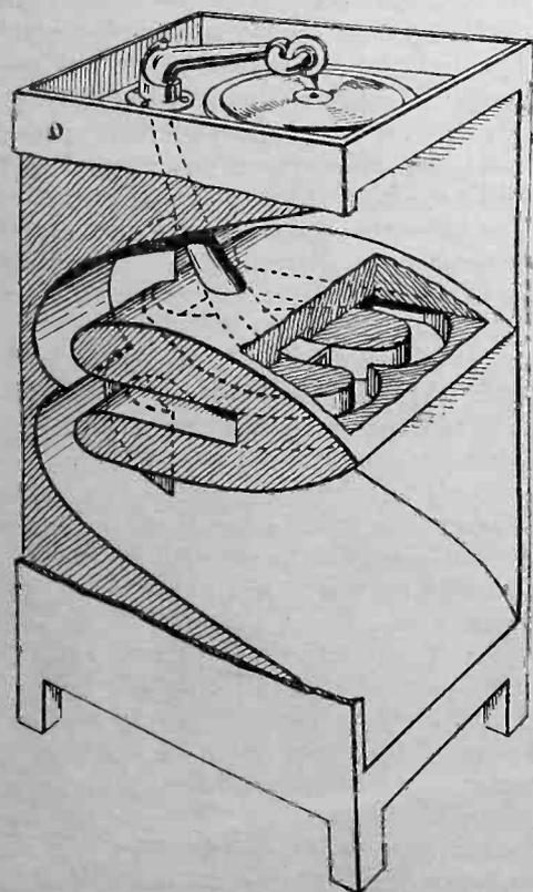
Fig. 1. Sectional View of Horn Type Phonograph.
