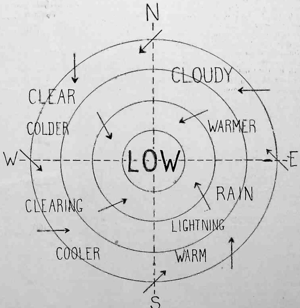
Fig. 3. Internal Structure of a Storm Area.
