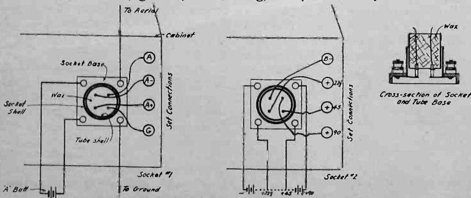
Fig. 1. Handy Antenna-Ground and Battery Connection.
