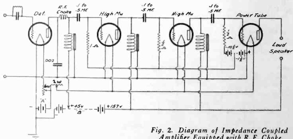
Fig. 2. Diagram of Impedance Coupled Amplifier Equipped with R. F. Choke.
