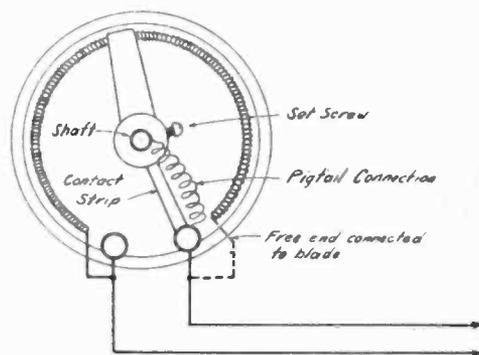
Fig. 2. Pigtail Connection for Rheostat.
