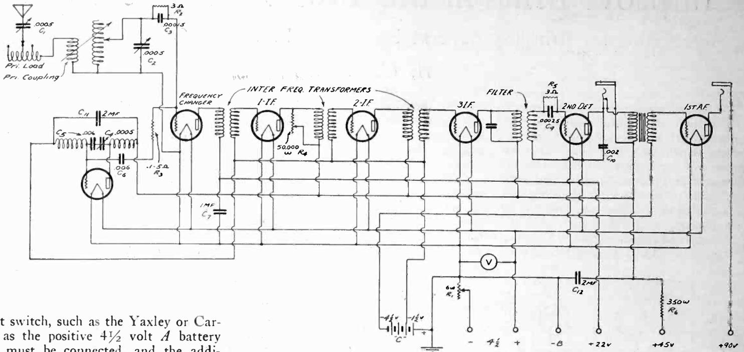
Fig. 3. Shielded all-wave superheterodyne, using all dry cell tubes.
