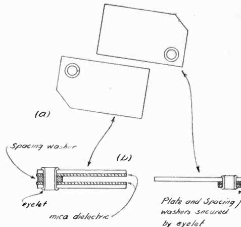
Fig. 4. Method of Adjusting Capacities.
