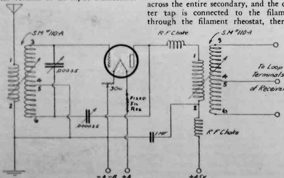
Fig. 1. Schematic Wiring Diagram of R. F. Unit.
