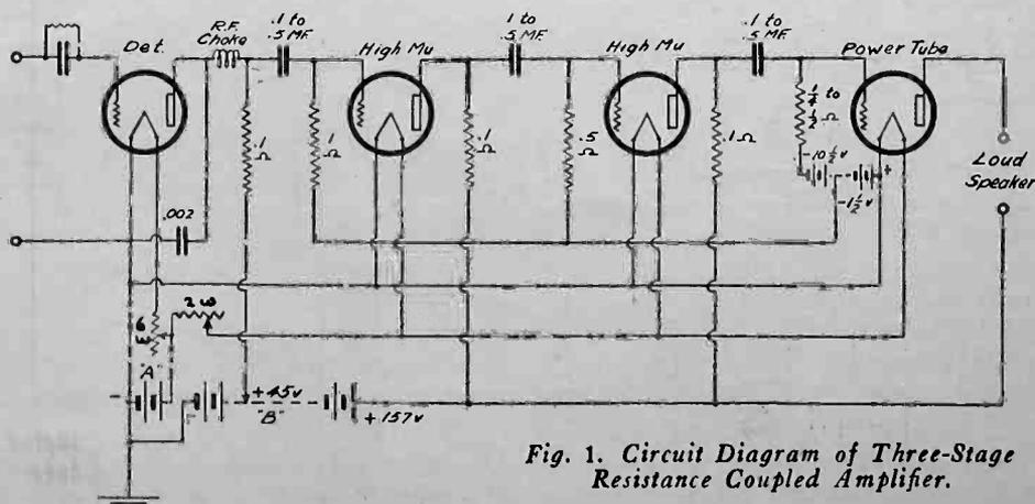
Fig. 1. Circuit Diagram of Three-Stage Resistance Coupled Amplifier.
