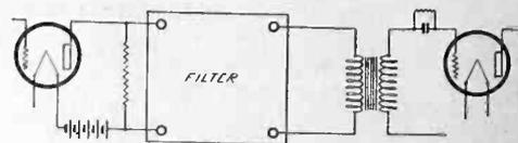
Fig. 1. Schematic Arrangement of Filter in Vacuum Tube Circuits.
