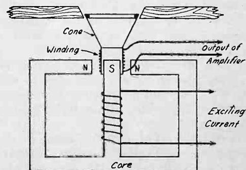
Fig. 3. Cone Speaker Used in Electrically Operated Phonograph.
