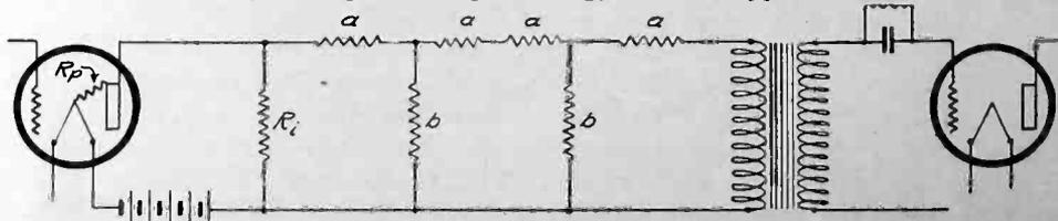
Fig. 2. Equivalent Impedances of Filter Sections.
