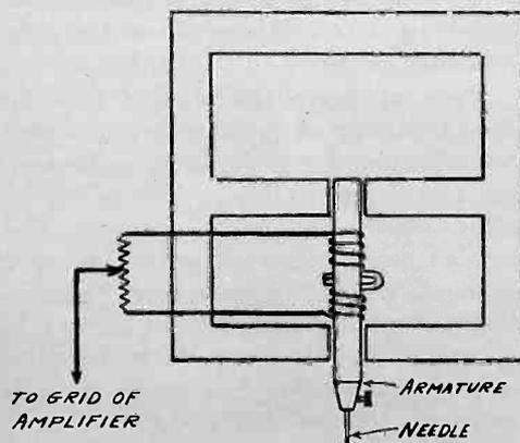
Fig. 2. Construction of Electro-Magnetic Reproducer.
