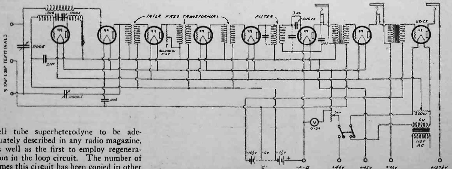
Fig. 2. Improved Best Superheterodyne, with additions, arranged for storage battery power tube.
