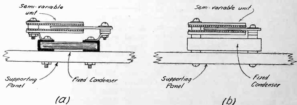
Fig. 5. Method of Mounting Condenser Units.
