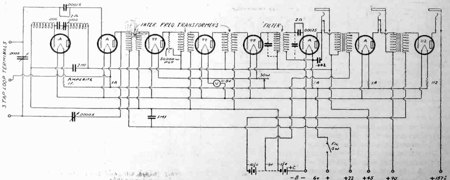
Fig. 4. Modified all-wave superheterodyne, unshielded model, as published in September 1925 RADIO.
