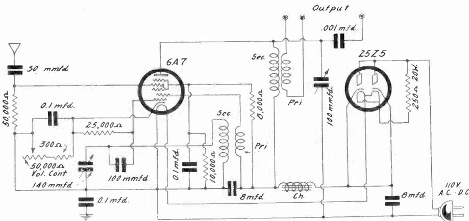
In this circuit, as in the first one shown, there is no tuning ahead of the generator, and practically the only substantial difference is that here the frequency of generation is not affected by antenna conditions. In the previous diagrams the series antenna condenser has an effect on tracking. The circuit is for universal operation.
