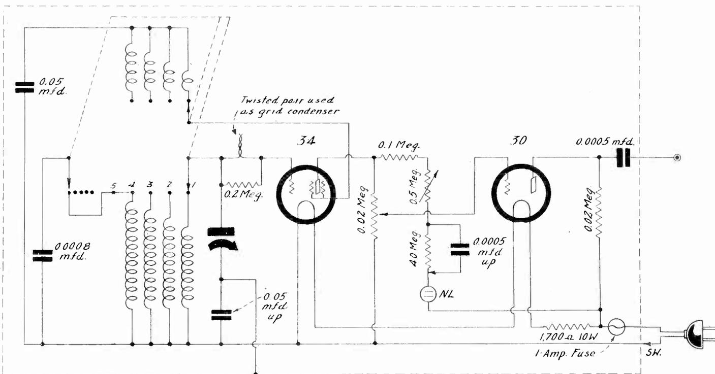
**The 333-AB Signal Generator, covering the following on fundamentals: 83 to 99.9 kc; 140 to 500 kc; 540 to 1,600 kc; 1,400 to 5,000 kc; 5,400 to 16,000 kc. This device can be used by an infallible harmonic system for measurements up to ultra frequencies. There is an amplifier stage to provide plenty of kick.**
