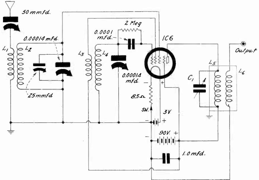
A tuned stage ahead of the generator is the only known method of tending to suppress images. This is also a battery-operated device and may be accepted as one yielding good results. The output is tuned to the frequency used in the receiver for the second level of amplification. L5L6 therefore may be a broadcast coil used backwards, as it were, with C1 the usual 0.00035 mfd. tuning condenser.
