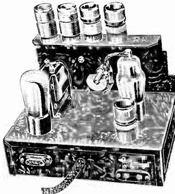
Battery operated S. W. receiver. Novel rack permits placing of five coils in proper band order—no groping for coils. Efficient design permits tuning from 15 to 200 meters. The regular broadcast band can be tuned with a broadcast coil (200 to 550 meters) at additional cost of 39c. Uses a 232 and 233 tube.
