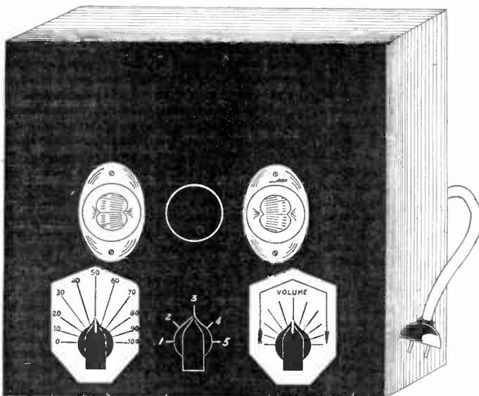
Front view of the 333-AB signal generator. The combination percentage modulation control and modulation on-off switch, applicable only to d-c use, is at left. The coil switch is at center. At right is the combination attenuator and a-c switch.
