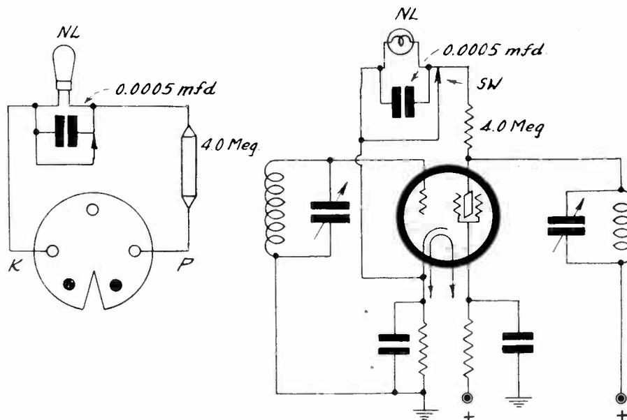
The same principle of a neon-tube audio oscillator, used for station-siren purposes, applied to a tube having a five-pin base. The control grids in both instances are brought out at top of the tubes. The same system, different wafer, may be applied to four-pin tubes.
