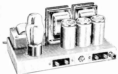
Supplies clear, hum-free power, regardless of circuit sensitivity. Especially designed for use with Dictator of the Air battery receivers. Delivers 180 volts with taps at 135, 90 and 45. Supplies 2½ volts at 10 amps. Uses 280 rectifier tube. Wired and tested with tube.....\$5.95
