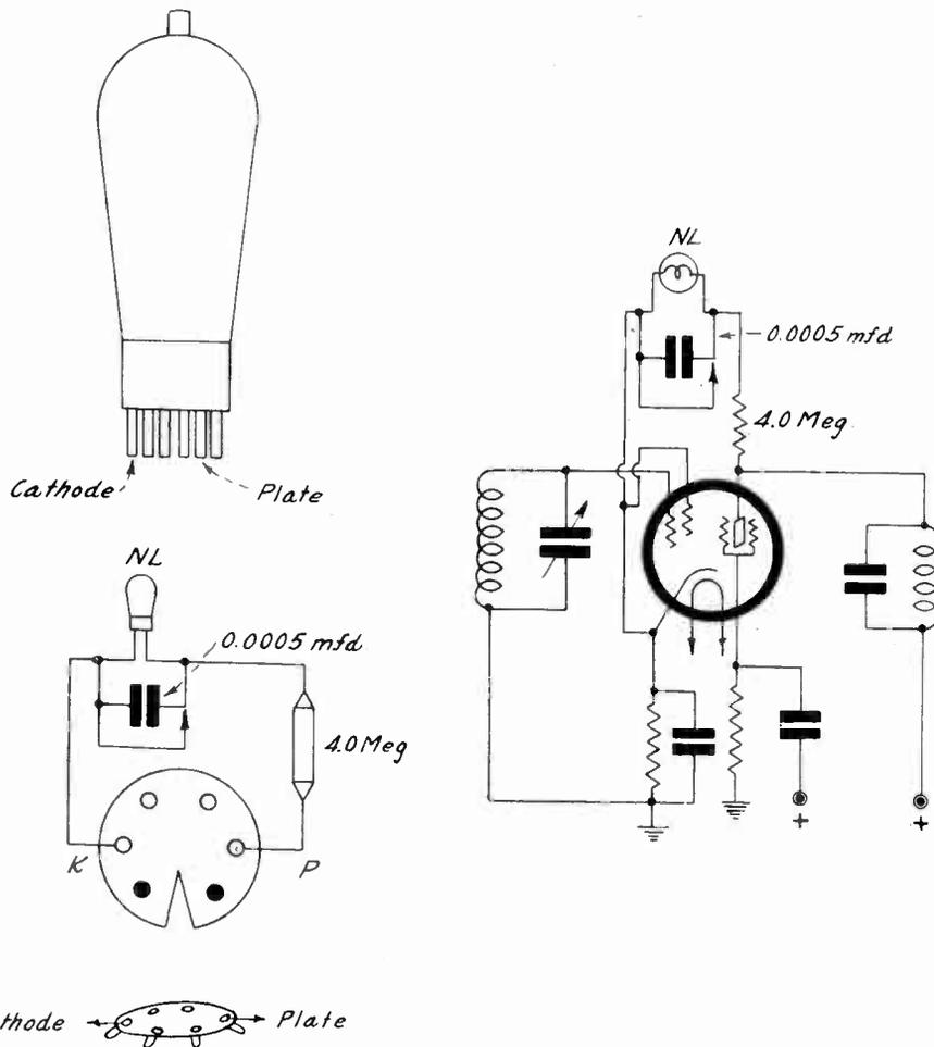
Removing a tube from a socket, placing a wafer between tube and socket, bringing out the plate cathode leads from the wafer, enables insertion of a neon audio oscillator network for service as a "station siren." The case of the six-pin tube is cited.
