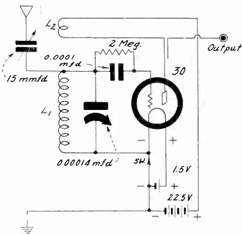
The simple circuit shown above serves as a short-wave converter of no consequence. It is well to build this little device, just so that one may appreciate what image interference is.
