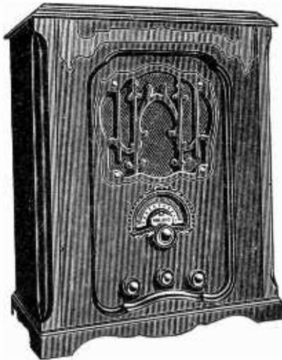
**B**LUEPRINT No. 627, full-scale, with schematic diagram also included, as well as a list of parts, is our most popular star circuit, since it is a-c operated and covers from 80 to 550 meters. Thus you can tune in television, police calls, some relay stations and the broadcast band. It uses five tubes: two vari-mu, either —35 or —51, one —24, one —47 and one —80. The chassis is 14½x7¾ inches, so may be fitted into a midget cabinet as illustrated.
