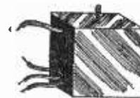
Three Supertone non-inductive fixed condensers of 0.1 mfd. each, (250 v.) in steel case, provided with a 6/32 mounting screw, built in. The black lead is common to the three condensers, the three red leads are the other sides of the respective capacitances. Size, 1 1/4" square by 7/8" wide. Order Cat. SUP-31, list price, \$1.00; net price, 57c.
