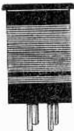
WOUND on 1.25 inch diameter finest bakelite forms, with flange for gripping, these short-wave plug-in coils afford high efficiency. Tube sockets serve as receptacles for these coils. The coverage with four coils is 13 to 200 meters with 0.00014 mfd. capacity. Also 0.00015 mfd. may be used without change. The coils may be used for any of the popular short-wave circuits.
