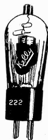
**A**FTER having tried many screen grid tubes, many specialists have made Kelly 222 their choice. Our 222 stands up! Filament is not critical, but 3.3 volts work best. Plate voltage may be from 90 to 180, but negative bias of 1.5 volts remains the same. The screen grid voltage, G post of socket, may be 22 to 45 volts, depending on how much amplification you want. A working amplification of 60 is easily obtainable (60 mu.).
