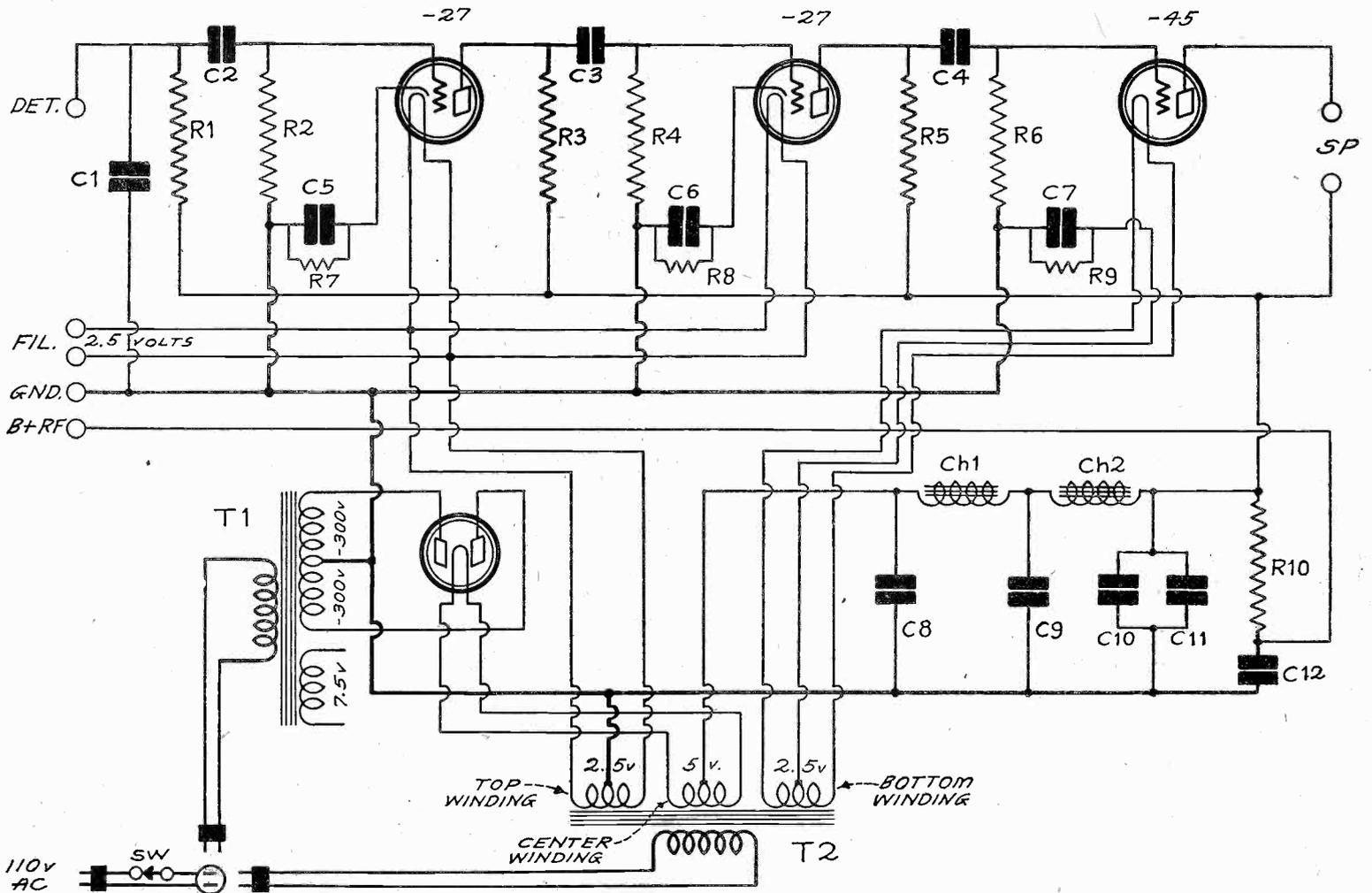
**A THREE-STAGE RESISTANCE COUPLED POWER AMPLIFIER FOR OPERATION FROM THE 105-120 VOLT 60 CYCLE AC LINE. THE FILAMENT VOLTAGE FOR HEATER TYPE TUBES OF AN INDEPENDENT RECEIVER IS SUPPLIED, ALSO B VOLTAGE FOR THE RECEIVER. COMPLETE STABILITY IS ASSURED. QUALITY IS EXCELLENT, VOLUME HIGH. NO MOTORBOATING.**
