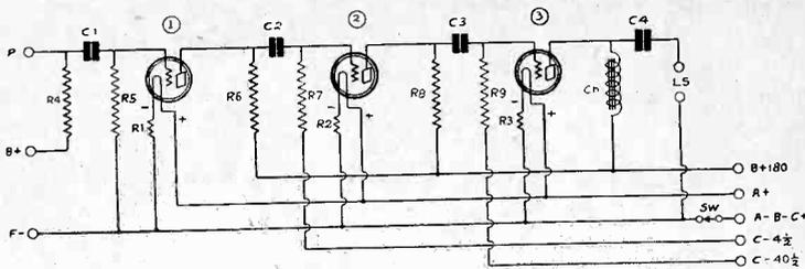
all in the "plate circuit" and all useful. The current then would be 1.5 milliamperes, if the bias were zero, but as a negative bias is used, the current is less. Hence resistance coupling brings about low plate current consumption.
