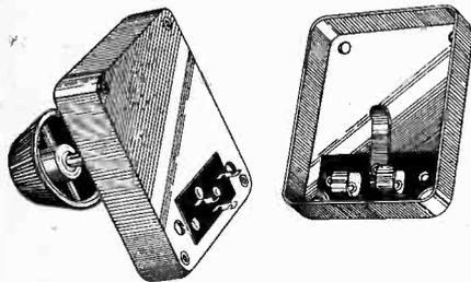
**THE NEW VOLUME CONTROL, AT LEFT, AS IT ACTUALLY APPEARS. AT RIGHT THE FRONT IS REMOVED TO EXPOSE THE RESISTANCE MECHANISM**
