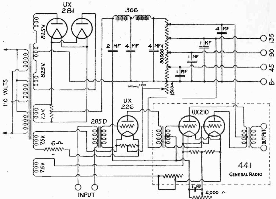
COMPLETE CIRCUIT DIAGRAM OF THE PUSH-PULL AMPLIFIER AND POWER SUPPLY DESCRIBED BY MR. WILSON. AN OUTPUT VOLTAGE OF 750 VOLTS DC IS PROVIDED FOR.
