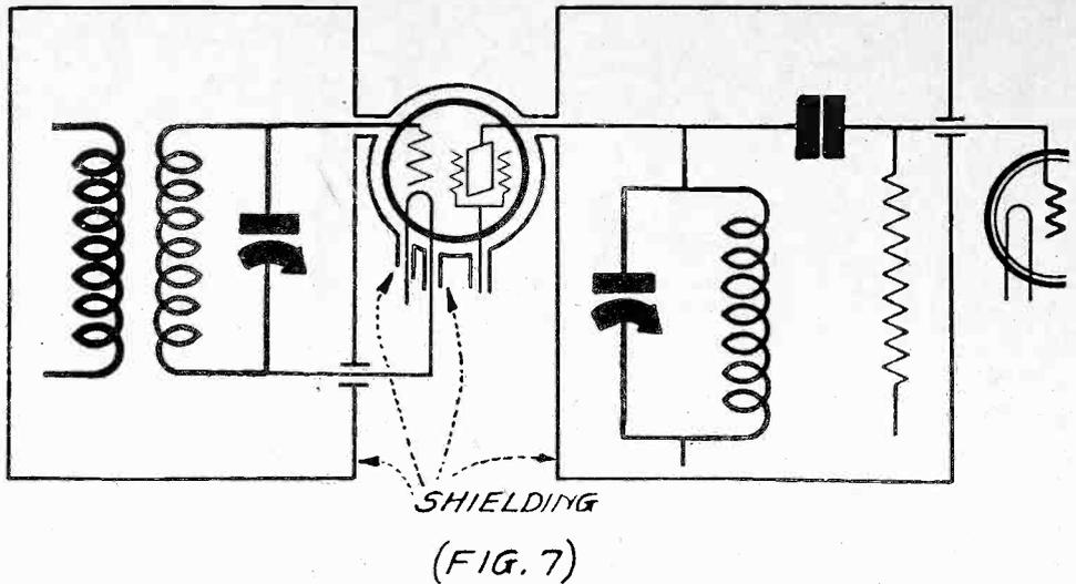
**FIG. 7—THE EFFECT OF THE SHIELD GRID DOES NOT EXTEND BEYOND THE TUBE ITSELF, AND THEREFORE CAREFUL SHIELDING OF THE EXTERNAL PARTS OF THE CIRCUIT MUST BE DONE.**
