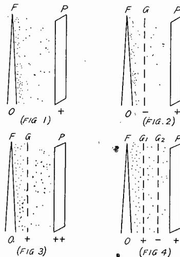
FIG. 1—THE APPROXIMATE SPACE CHARGE DISTRIBUTION BETWEEN THE PLATE AND THE FILAMENT WHEN NO GRID IS INTERPOSED. MOST FREE ELECTRONS ARE NEAR THE FILAMENT.
