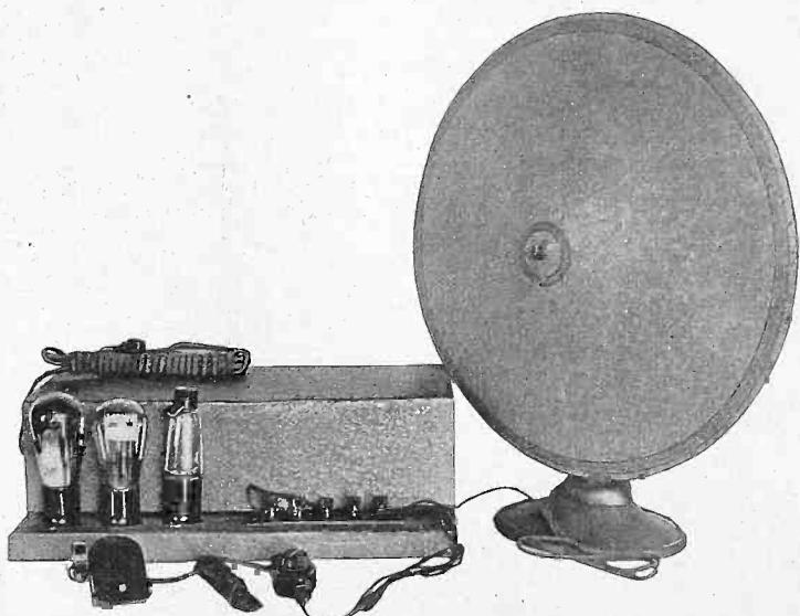
A POWER AMPLIFIER AND B SUPPLY, WITH PHONOGRAPH PICKUP [PHONOVOX] INTRODUCED IN A SPECIAL WAY, HAS BEEN DEVELOPED BY LOUIS G. PACENT. AN ADVANCE VIEW OF THE EXTERIOR IS SHOWN. SOON THE CONSTRUCTION WILL BE DESCRIBED. THE TUBES USED ARE ONE 281 (RECTIFIER) ONE 227 OR KELLOGG OR McCULLOUGH, AND ONE 210. IT IS ESPECIALLY ADAPTABLE FOR HOUSING IN PHONOGRAFS.
