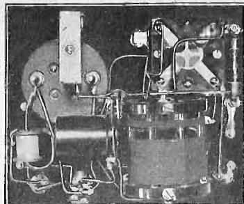
AN INTERIOR VIEW OF THE ADELMAN UNIVERSAL TESTER SHOWING THE PLACEMENT OF THE DIFFERENT PARTS. THE ELECTRIC METER IS SHOWN AT THE UPPER LEFT CORNER, THE TUBE SOCKET AT THE RIGHT. IN THE LOWER TIER THE VOLTAGE MULTIPLIER IS AT THE LEFT, THEN THE RADIO FREQUENCY CHOKE COIL AND AT THE RIGHT, THE OSCILLATING COIL. ON THE PANEL ARE SEEN THE TELEPHONE JACK, THE FILAMENT RHEOSTAT AND THE SWITCH.
