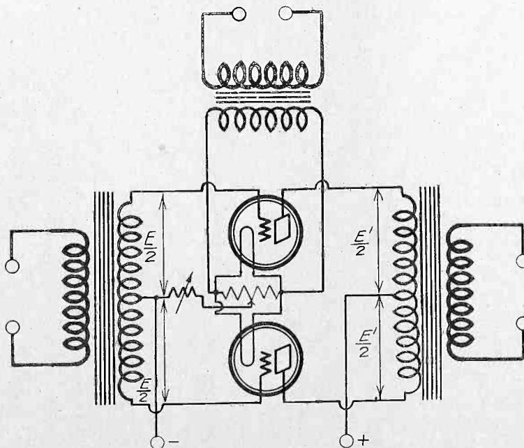
ONE STAGE OF PUSH-PULL AMPLIFICATION WITH AC HEATED FILAMENTS. THE INPUT VOLTAGE  $E$  IS DIVIDED EQUALLY BETWEEN THE TWO TUBES. EACH AMPLIFIED HALF  $E\frac{1}{2}$  APPEARS ACROSS HALF OF THE PRIMARY OF THE OUTPUT TRANSFORMER, AND THE TOTAL OUTPUT VOLTAGE IS  $E'$ .  $R$  SUPPLIES THE GRID BIAS WITHOUT DETRIMENTAL EFFECTS.
