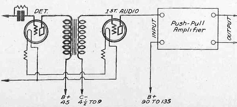
HOW THE OUTPUT OF A STAGE OF TRANSFORMER COUPLED AUDIO FREQUENCY AMPLIFICATION IS HOOKED ON TO THE INPUT OF THE GENERAL RADIO TYPE 441 PUSH-PULL AMPLIFIER IS DIAGRAMMED ABOVE.
