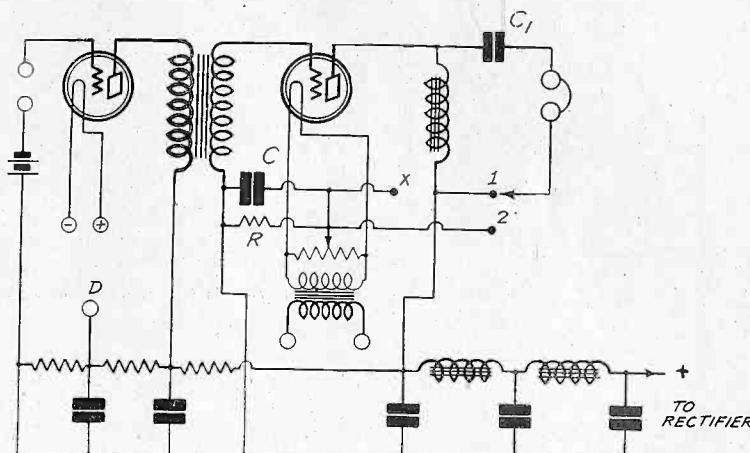
THIS DIAGRAM ILLUSTRATES THE EFFECTS OF THE GRID BIAS RESISTOR ON THE QUALITY OF REPRODUCTION, AND IT INDICATES THE PREFERRED CONNECTIONS OF BY-PASS CONDENSERS AND THE LOUD-SPEAKER TO MINIMIZE THE EFFECTS.
