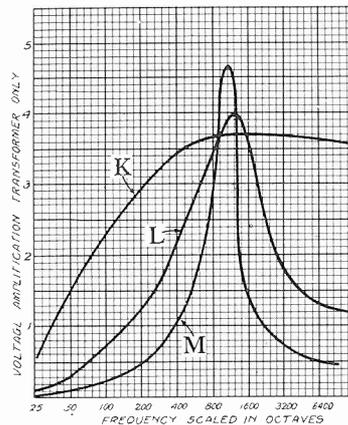
THESE CURVES ILLUSTRATE PHASE SHIFT AS RELATED TO AMPLIFICATION. AT OR VERY NEAR THE HIGHEST POINT ON EACH CURVE THE PHASE SHIFT IS ZERO. WHERE THE AMPLIFICATION IS DOWN THE PHASE SHIFT IS HIGH.
