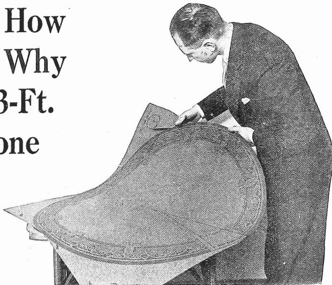
paste the edges together by pressing gently on the same, starting at the inner apex and working outward. Allow cone to dry for a few minutes and then paste in the small cone which is cut from corner of sheet as shown in Fig. 1. This small cone goes on the inner apex when pedestal or wall cone is made and on the outer apex when console type is made. The small cone makes the large cone rigid. When cone is completed, lay it face down and bend back the edge on the scored line.
