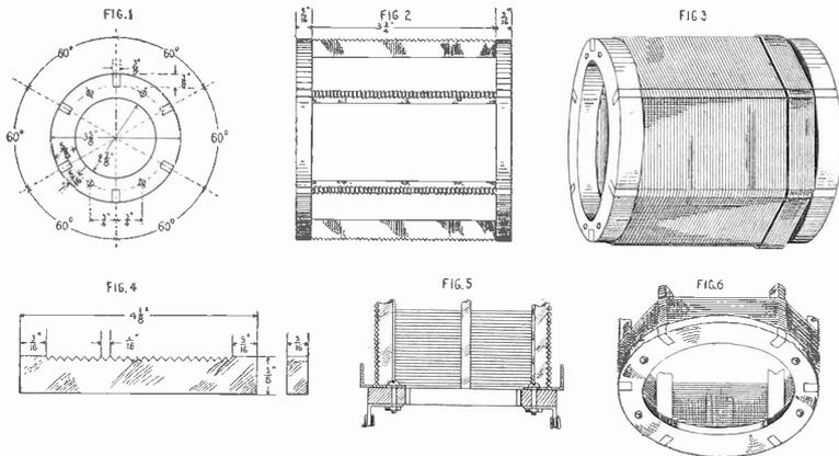
FIG. 575 How to make a tuned radio frequency coil.
