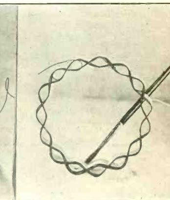
FIG. 10—Showing how a sparing application of collodion is made to render the coil more secure. A little collodium is not harmful, but a lot of it is injurious, causing severe losses.
