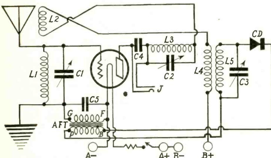
THE 1-TUBE Reflexed Superdyne diagrammed above, affords fine signal quality because of the crystal used as the rectifier. This circuit is not selective enough for those living in cities. L1L2 are both on one tubing and are fixed coupled. All the coils may be made at home. There are three controls, the variable condensers C1, C2 and C3. This is a good reflex for the beginner to build. It is not a DX set. The circuit was described in the December 6 issue.
