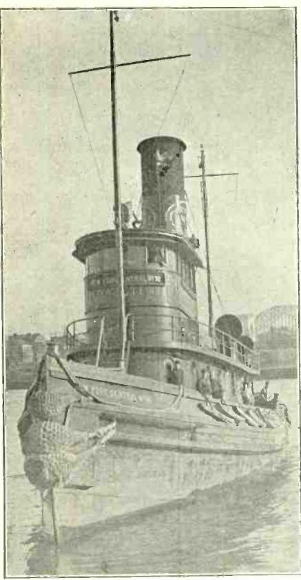
THE PROUD TUGBOAT, first to be equipped with radio for commercial purposes in New York Harbor, is known as New York Central No. 18. Orders directing the movement of the tug are received on a short-wave set, instead of being telephoned over land wires and the message "called for" at a pier. (Kadel & Herbert)
