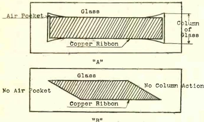
Fig. 1. Diagrams showing unsuccessful and successful methods of sealing a copper ribbon in glass.
