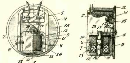
New method of locating the magnets of a telephone with regard to the diaphragm.
