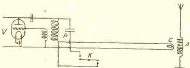
W. T. Ditcham's method of using inductive coupling in sustained wave transmission.
