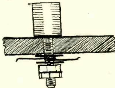
Fig. 2. Method of fastening the string to get good contact. It is wrapped around the shank under the washer.
