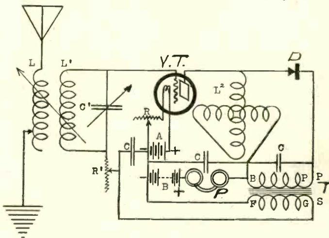
A highly selective reflex circuit using one tube and a crystal detector.
