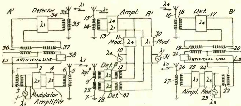
Colpitts' new method of modulating telephone signals.
