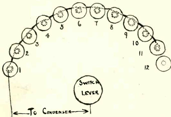
Fig. 1. Method of making a variable grid leak by fastening an India ink soaked string under the nuts of taps.
