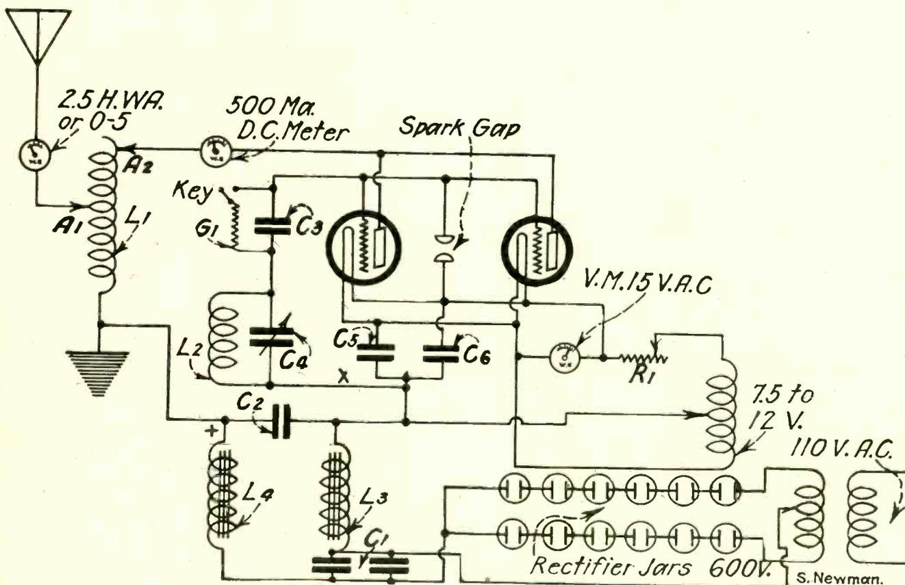
A neat and powerful CW or phone transmitter circuit. If you have been looking for an efficient transmitter construct this and you won't go wrong.
