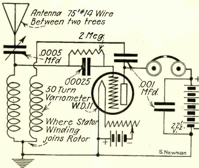
Mr. Turnbull's new circuit which permits the construction of a simple set with but two controls, yet which will satisfy the seekers of super-selectivity.
