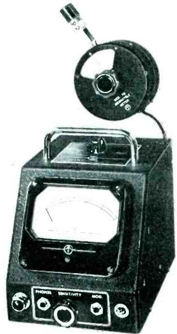
Technical specifications are as follows: Frequency range—2.2 to 400 mc with seven plug-in coils; Modulation—c.w. or 120 cycles fixed approximately at 30% at 15 mc, or external.
