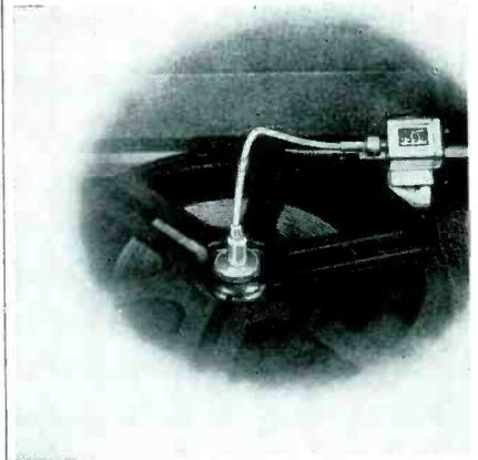
A cueing indicator counts each revolution of the wire or tape spool, and reverses when the wire or tape is rewound, automatically bringing the reading back to zero after the rewinding is completed. Average accuracy is within approximately one second of recording time on standard spools of wire or tape. Literature available on request.
