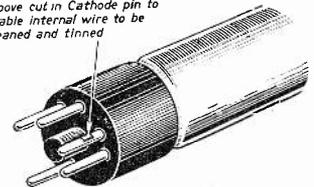
To effect a repair, a small groove was carefully filed into the cathode pin at a position approximately one third of the length from the tube end. This exposed the internal connecting wire, which was carefully cleaned and the complete groove filled in with solder and finally cleaned to the original pin diameter. This effected a complete cure.—J.E.R., Nottingham (921).
