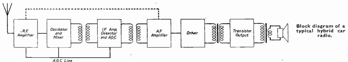
Block diagram of a typical hybrid car radio.
