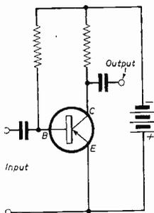
Left: Basic circuit of a grounded emitter stage.
