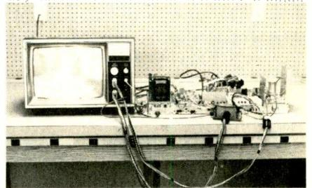
Fig. 3—Photo taken in ETD's test laboratory showing the test jig in operation, producing a well proportioned TV picture.
