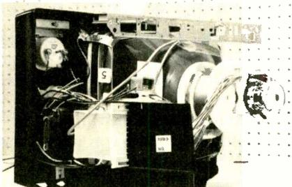
Fig. 2—Side view showing the principal components employed in Sylvania's Chek-A-Color test jig.
