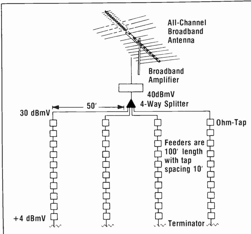
Fig. 3—Functional diagram, or layout, of a typical "all-channel" MATV system.
