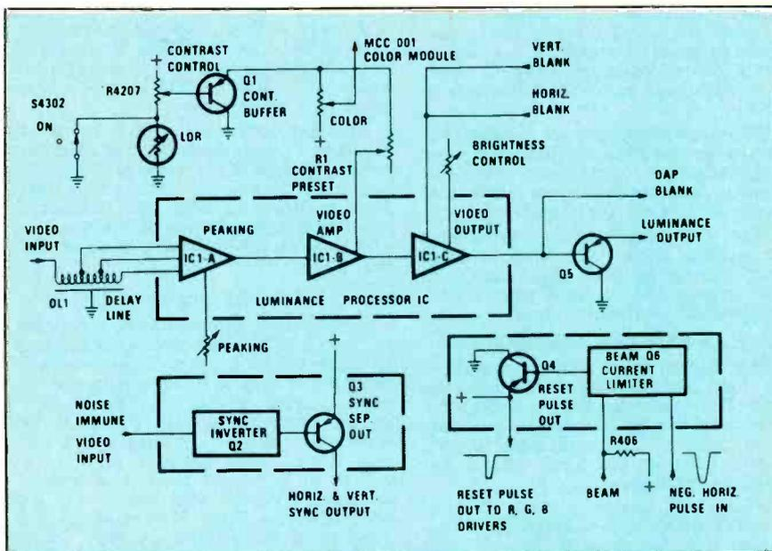
Fig. 4—Block Diagram of the Luminance Module MCL001 and associated circuitry.
