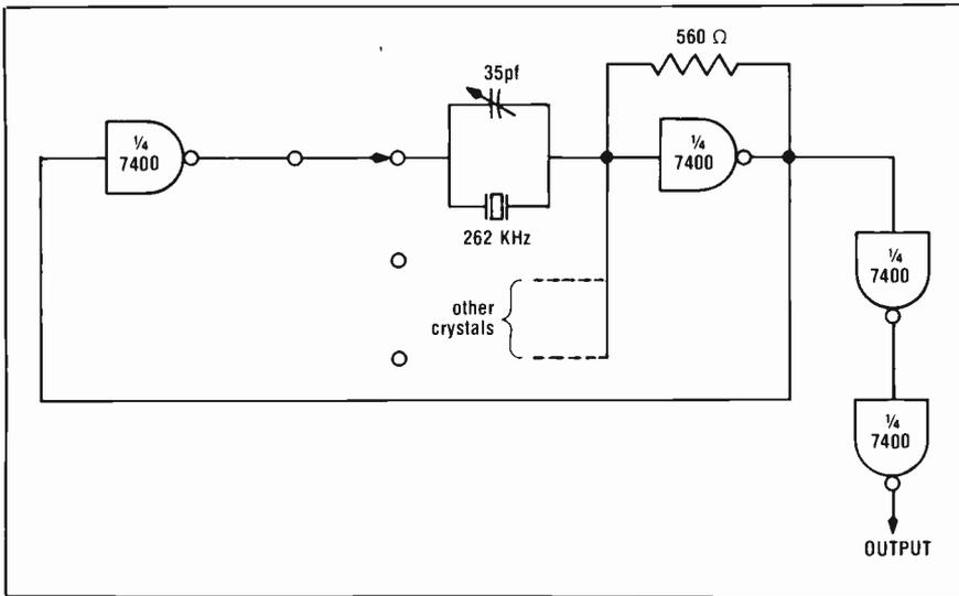
Fig. 4—Crystal-controlled, 100-KHz to 2000-KHz oscillator, most of the circuitry of which is contained in a single type SN7400 TTL integrated circuit. (Crystals for this oscillator circuit and that in Fig. 3 are available from a number of sources, including JAN Crystals, 2400 Crystal Dr., Fort Meyers, Florida 33901. Specify for a 32-pf load and whatever type of holder you want—type HC6/V or HC25 are recommended.)
