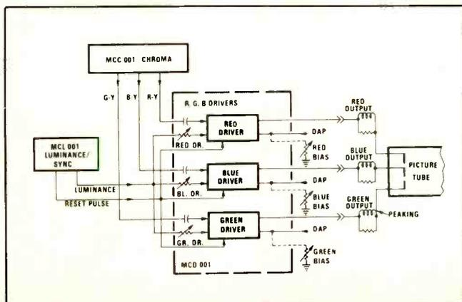
Fig. 5—Diagram of the Red, Green, Blue Driver Module MCD001 and associated systems.
