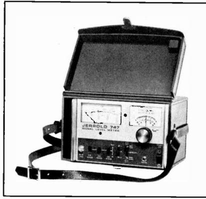
Fig. 1—A typical field-strength meter.
