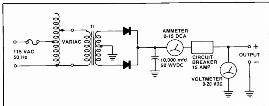
Fig. 1—Power supply for car radio/tape player servicing.
