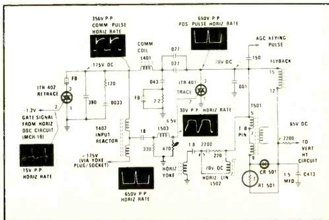
Fig. 6—Trace and Retrace circuits employed in the CTC74 color chassis feature Intrinsic Thyristor Rectifiers (ITR).
