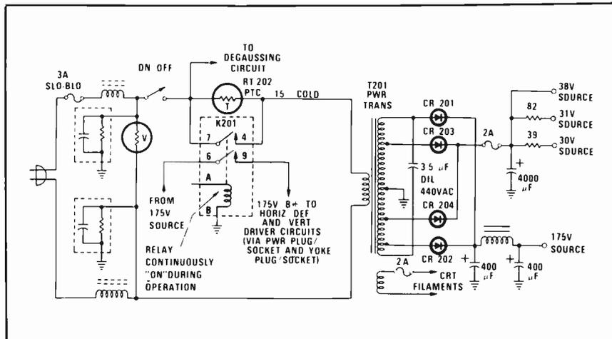
Fig. 8—Basic CTC74 and CTC81 color chassis power supply circuit employing a constant voltage transformer. Photos and illustrations supplied through the courtesy of RCA.
