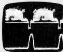
Video waveforms can be checked quickly and precisely with the RCA Dual-Tracer. Top: Composite video waveform. Bottom: Color burst keying pulse. Sweep: TV/H.
