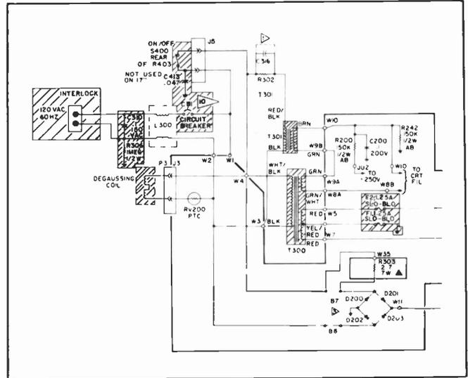
proper operation. The capacitor is designated C316 and the schematic has a footnote indicating which capacitor is required. If a wrong value capacitor is used, the transformer will overheat.
