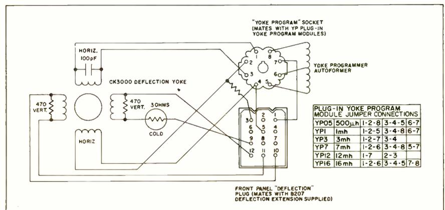
Schematic diagram of deflection circuit employing a Yoke Programmer Autoformer.
