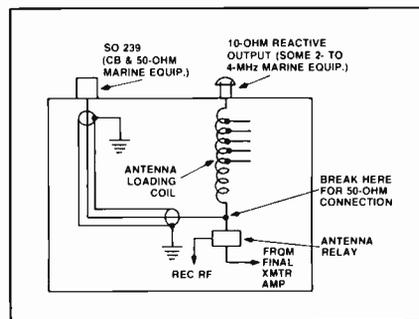
Fig. 1—Composite illustration which shows the locations of the 50-ohm output test points in typical types of SSB equipment.
