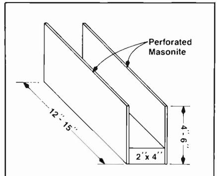
Fig. 6—Auto radio holder devised by Frank Weisel, Norfolk, Virginia.
