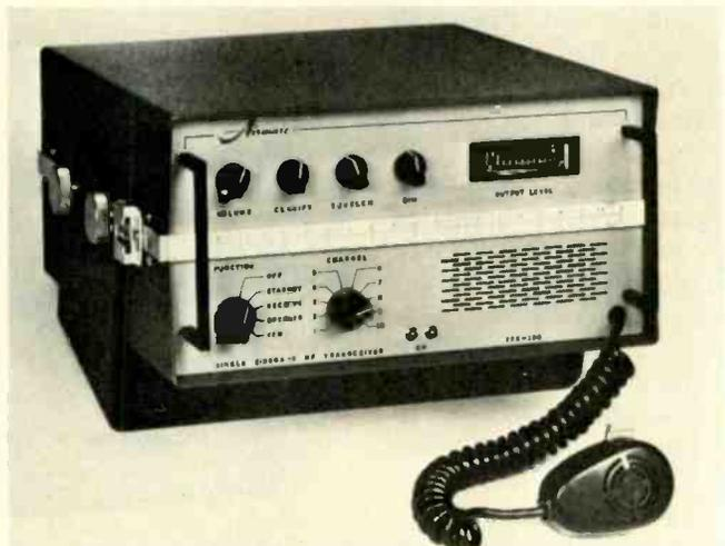
A 10-channel SSB marine radio. Courtesy of Airmarc Marine Products.
