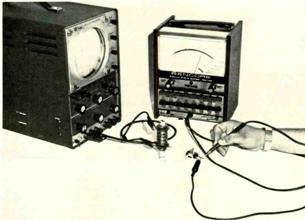
Fig. 14—An electronic technician is shown measuring the resistance of a potentiometer to determine the ac resistance of the coil.
