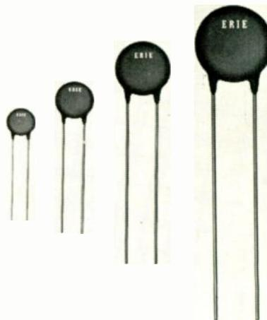
Capacitors to 0.47  $\mu$ f, 25 vdcw, is offered in the "Transcap" line of ceramic capacitors. A new style offers 0.22  $\mu$ f in a case size of only 0.895 in. x 0.156 in. thick and 0.47  $\mu$ f in a case size of only 0.895 in. dia x 0.200 in. thick. Besides a very high capacitance per unit volume, another advantage cited for these capacitors is that the high resistivity
