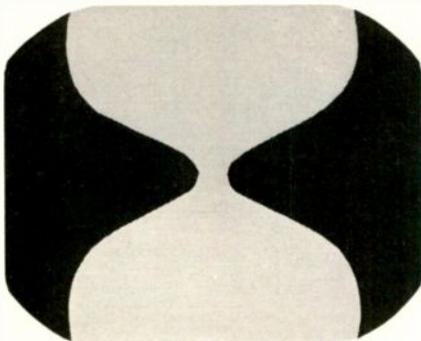
"Hour-glass" raster distortion results from 60 cps ripple impressed on the horizontal output grid circuit.
