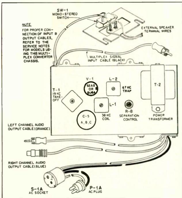
Tube and alignment point locations for Emerson Stereo Multiplex Chassis 471362.
