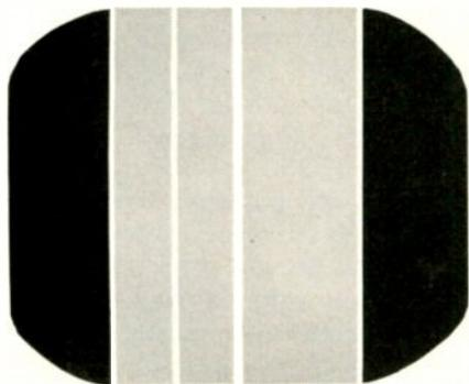
Pattern generated by a receiver having a shorted boost capacitor and with damper tube removed.
