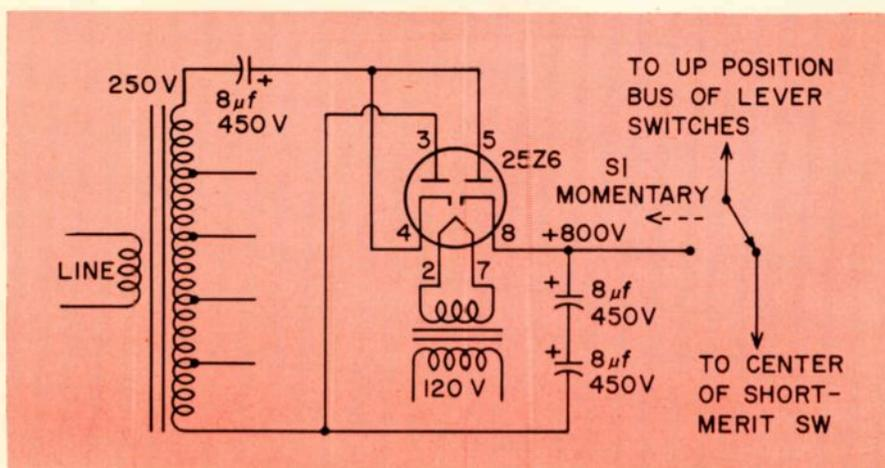
Circuit modification to convert tube testers into rejuvenators.
