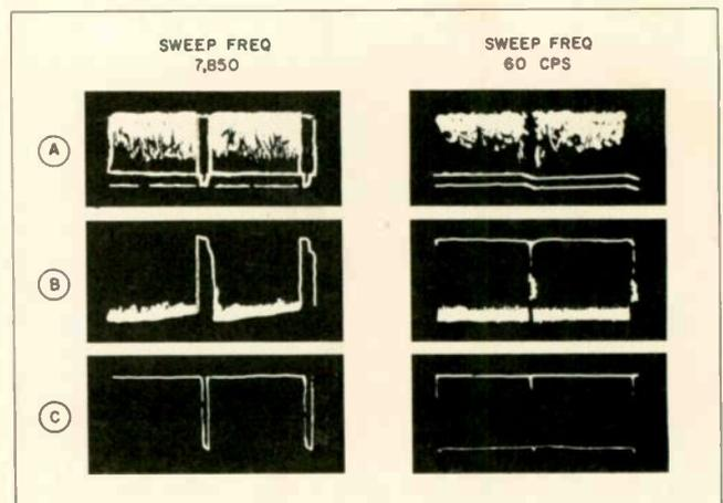
Fig. (A) — Horizontal and vertical waveforms at the input to the sync amplifier. (B) — After being processed in the first sync separator most of the video has been clipped and the pulse is amplified. (C) — An additional clipper removes all video from the sync.
