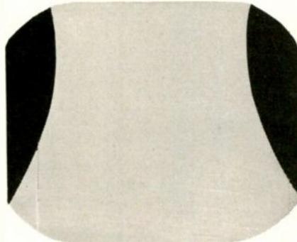
Less severe form of "hour-glass" is usually called "coke bottle." Causes are the same as for more severe distortion.
