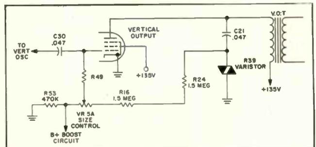
The vertical size compensation circuit used in Philco 13G20 chassis.
