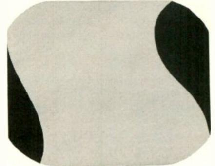
"S" distortion unaffected by video content is frequently caused by a heater-to-cathode short in the output tube.
