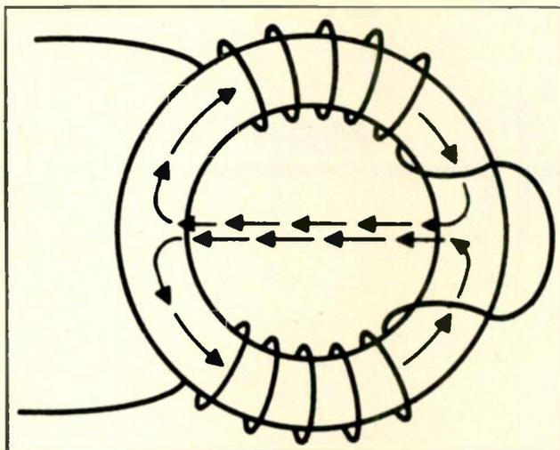
Method used to wind a toroidal coil.
