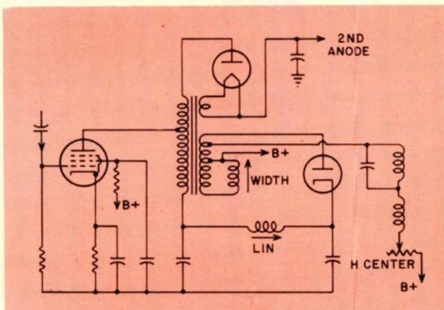
Typical Horizontal output system schematic.
