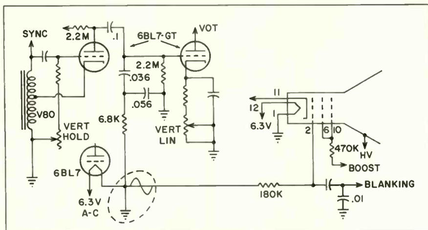
Poor ground caused "cycling" foldover.
