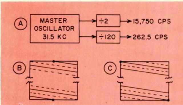
Fig. 2 (A) — Exact odd-line relationship between vertical and horizontal rates as maintained by divider circuits from a common oscillator. Odd ratio between rates causes scan to end on a half line on one field and a full line the next field. (B) — Beginning and end points of the half-scan line field. (C) — Beginning and end points of the field preceding or following the half line field.
