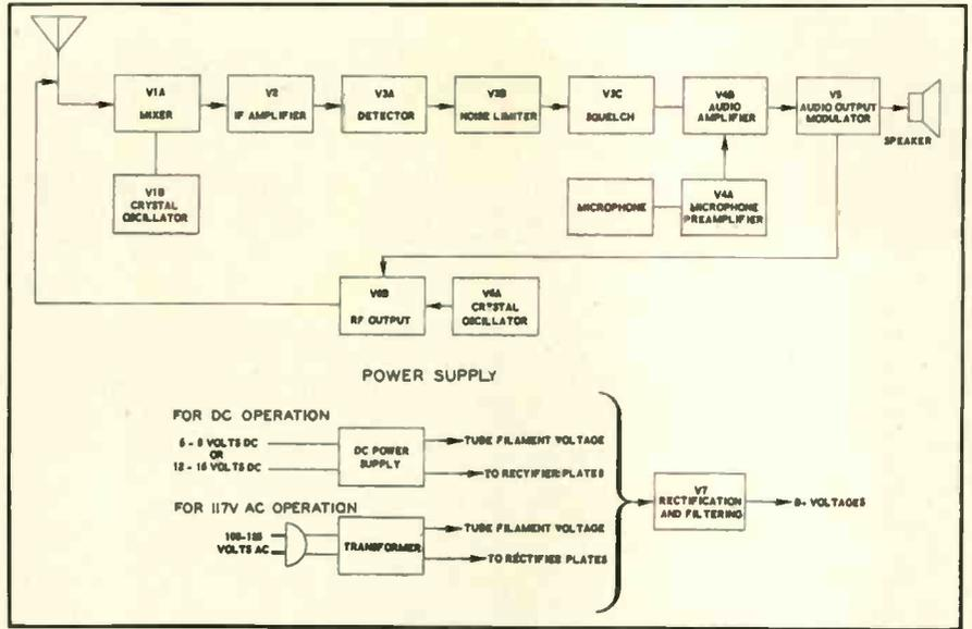
Fig. 1 — Block diagram of Heath's GW-12. Transceiver power supplies shown are external and optional. Switching components are not shown for clarity. One coil is employed for the antenna input and RF tank circuits.
