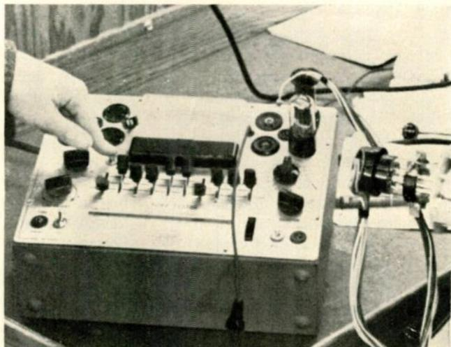
Completed tester with rectifier tube plugged into the spare socket. The adapter cable is attached in the same manner as for CRT testing.
