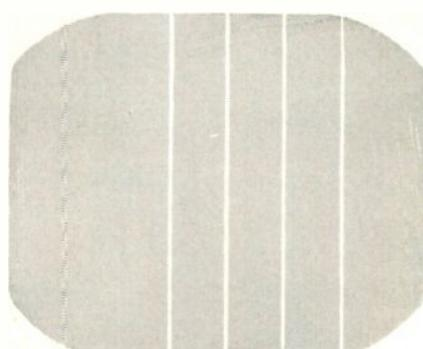
Damper tube or yoke are most frequently at fault when light wrinkles appear in raster.
