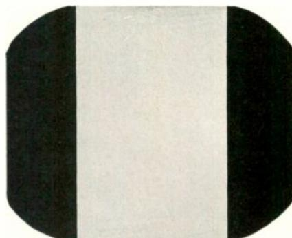
Insufficient width but with no foldover may be caused from aging of several components. This is most easily cured with "over-riding" circuit additions.
