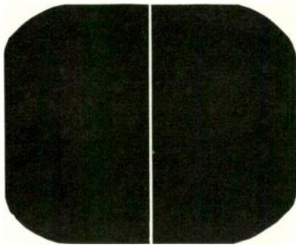
Open yoke winding sometimes causes a single vertical line and reduced high voltage. High voltage reduction may be insignificant.
