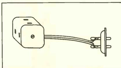
Adapter for cheater cord has outlets for several instruments.
