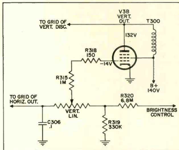
Vertical output circuit used in the Westinghouse V-2438 Chassis.
