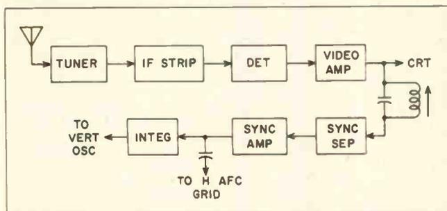
Sync flow path through most TV receivers. The sync separator clips video from the composite signal leaving only horizontal and vertical sync pulses.
