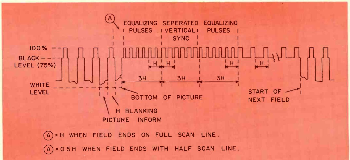
Fig. 1 — Sync pulse structure varies on odd and even scan fields. Equalizing pulses and the serrated vertical sync pulse maintain proper horizontal oscillator frequency during vertical blanking and sync time.
