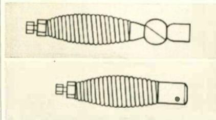
give the user positive grip. Made of stainless steel, these non-corrosive springs adapt to the firm's Mobile VHF antennas and are rigid enough to resist wind but flexible enough to bend for low clearances. Both a standard base and a ball-joint to allow mounting on angular surfaces are available. G. A. M. Electronics, Inc.
