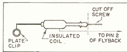
I took an ordinary width coil and inserted it between the primary of the flyback transformer and the plate of the horizontal amplifier, as shown in the sketch. When the receiver was tried after this change, it immediately worked as it should.
