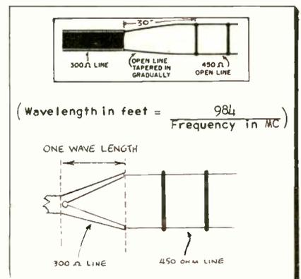
Fig. 3—Methods of matching 450-ohm open-wire line to 300-ohm twin lead. Top sketch: the open wire is tapered down to the twin lead over a distance of 30 inches from the first "spreader," as shown. Bottom sketch: 300-ohm line is split over one wave length, and fanned out to the connecting points on the open-wire line.
