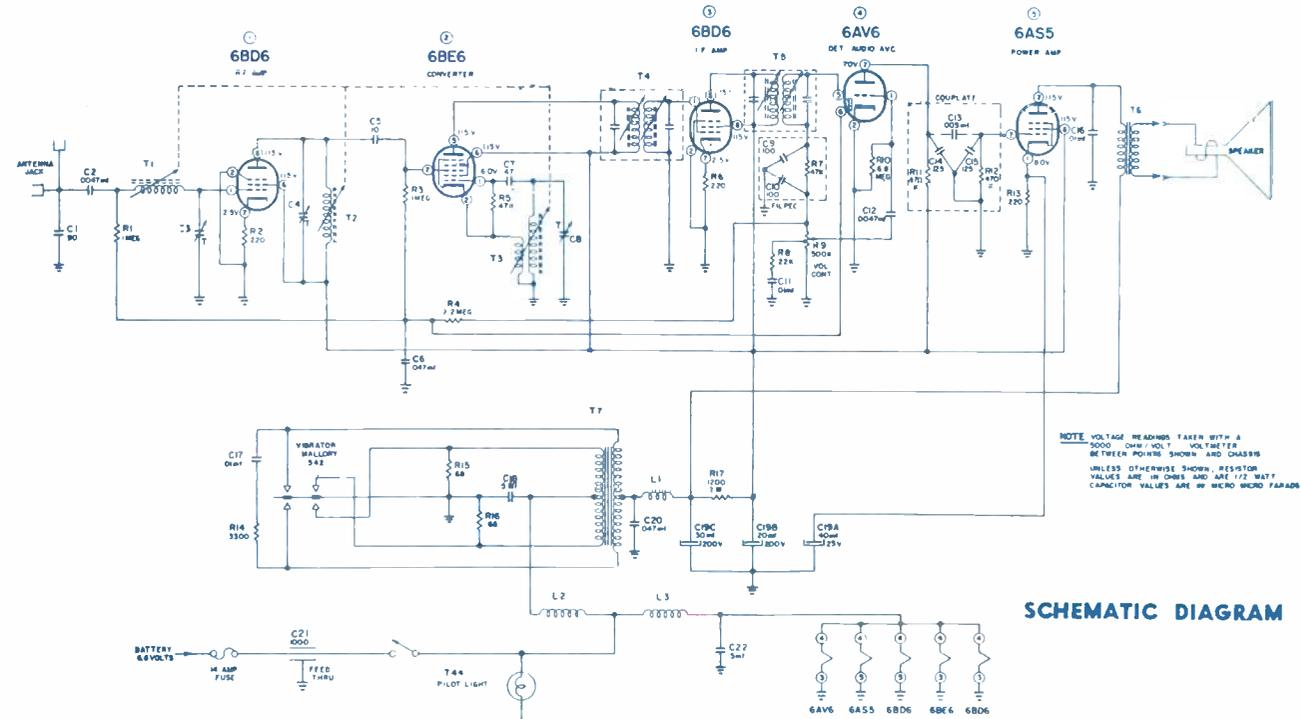
NOTE: VOLTAGE READINGS TAKEN WITH A 5000 OHM PER VOLT VOLTMETER BETWEEN POINTS SHOWN AND CHASSIS UNLESS OTHERWISE SHOWN. RESISTOR VALUES ARE IN OHMS AND ARE 1/2 WATT. CAPACITOR VALUES ARE IN MICRO MICRO FARADS.
