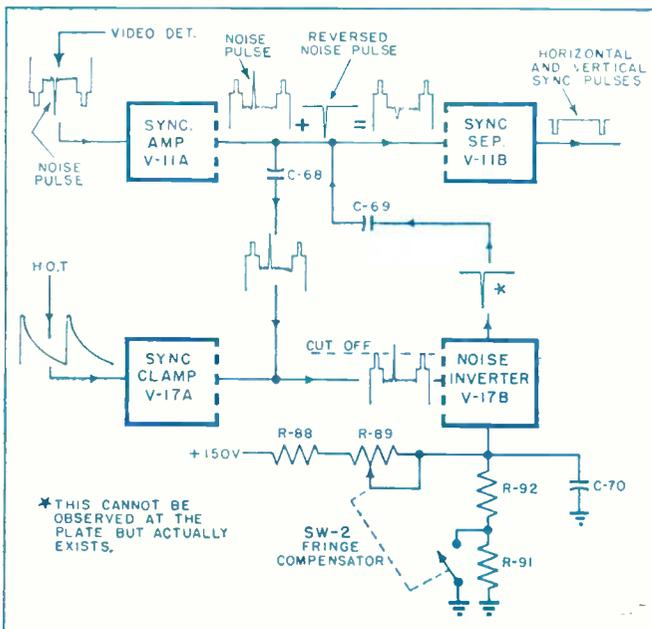
Fig. 2—Noise inverter and associated circuits used in Emerson chassis 120174-B, 120198-D. For complete schematic, refer to Emerson Circuit Digest in this issue.
