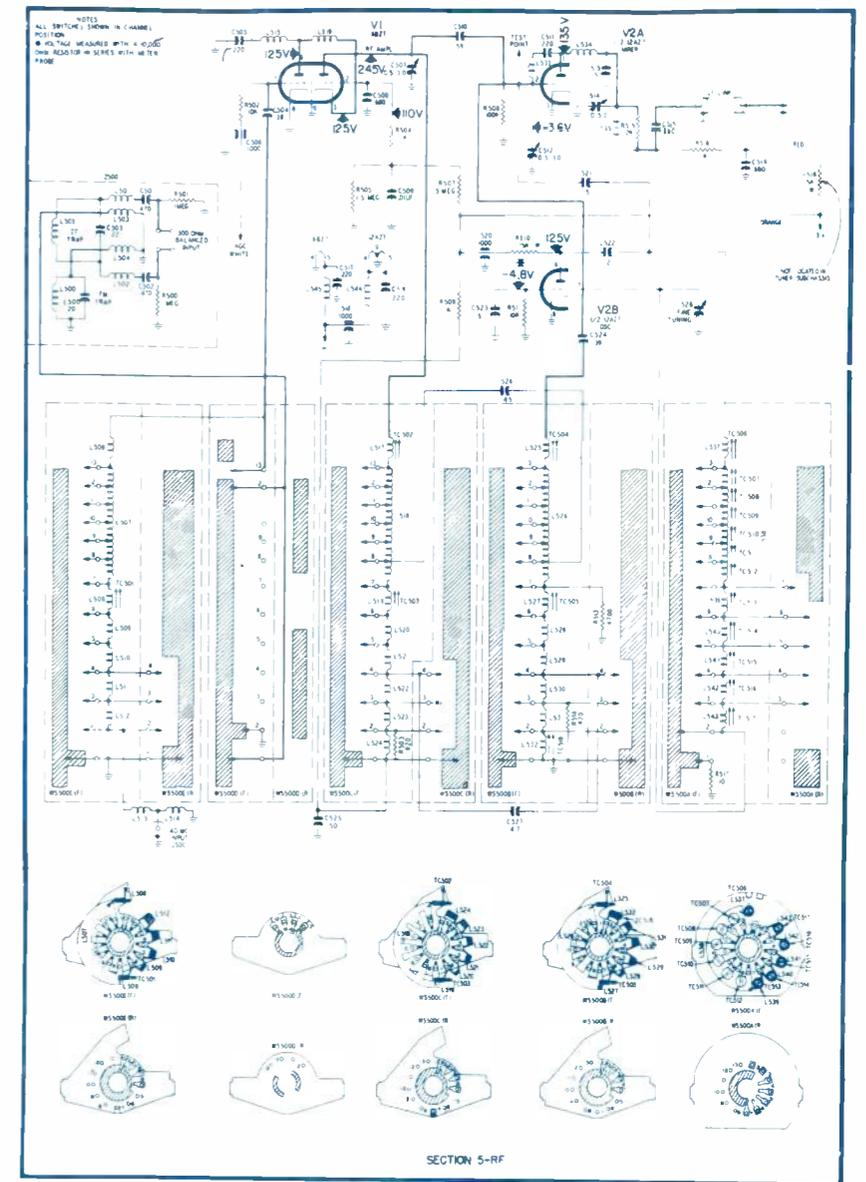
**Television Tuner, Part No. 76-7600-3, Schematic Diagram**
