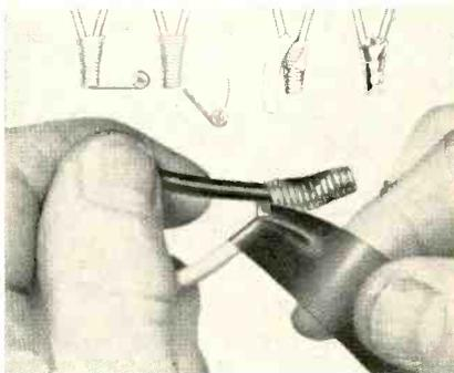
is snapped off. The electrical tape is started on the connector and brought forward to seal its bell end. Then, wrapped around the connector until it extends  $\frac{1}{2}$ -in. beyond the small end of the connector, the tape is folded back and further wound toward the bell end to complete the splice. Minnesota Mining & Mfg. Co., St. Paul 6, Minn.—TECHNICIAN.
