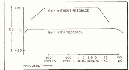
Fig. 5—Response of typical amplifier with and without feedback.
