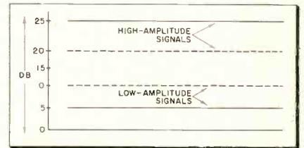
Fig. 11—Graph indicating effects of amplitude compression on high and low-amplitude audio signals. Dotted lines represent high and low-amplitude signals after compression.
