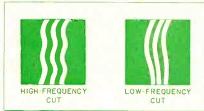
Fig. 9—Comparison of high and low-frequency cuts made by stylus. Grooves shown for both frequencies were made with the same signal amplitude applied to the cutting head. Note the reduced separation between grooves in the low-frequency cut.
