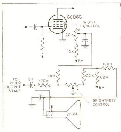
Fig. 3—An increase in the 22K resistor connecting to the brightness control caused an excessive CRT bias, dimming picture and raster greatly. This bias could not be reduced below -30V by manipulation of the brightness control.
