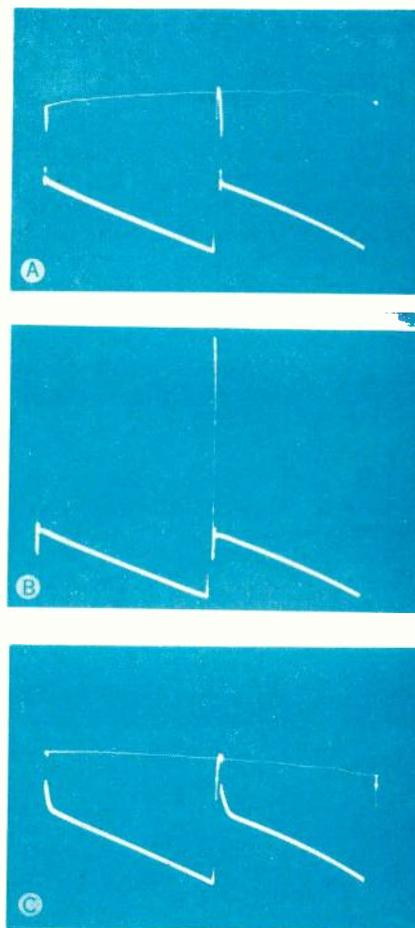
Fig. 2—Actual plate voltage waveforms for the vertical output tube, under the conditions of Fig. 1.
