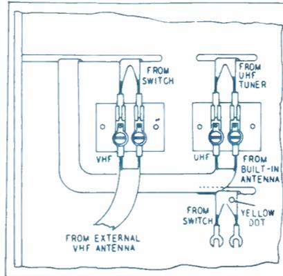
**Antenna-Lead Connections, VHF External and UHF Built-In Antennas**
