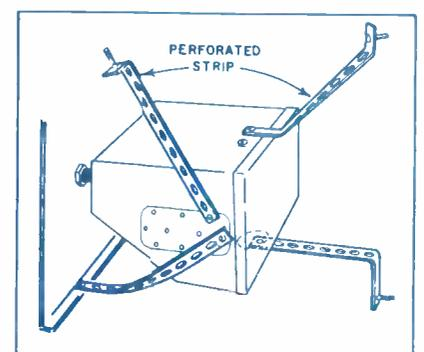
Figure 11. Receiver Mounting
