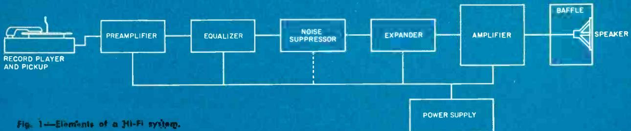
Fig. 1—Elements of a Hi-Fi system.
