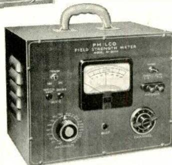
**Model M-8104—TV Field Strength Meter** • Offers more features than any unit at this popular price . . . Super Colorado Tuner for low noise and high gain . . . May be used to check TV boosters, antenna combinations, interfering signals and picture signal strength.
