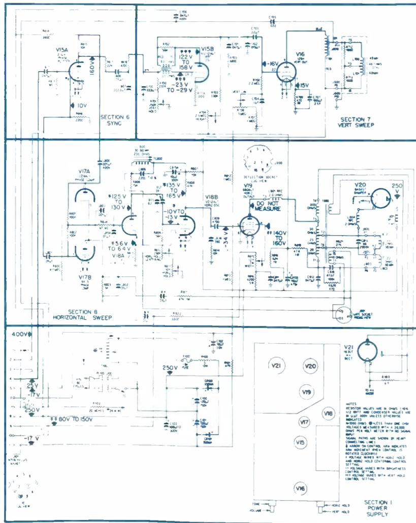
**Deflection Chassis D-201, Schematic Diagram**
