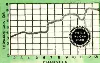
**CAUTION:** It is the policy of VEE-D-X not to falsify gain charts for advertising purposes. This Tru-Gain Chart is exact and is based on standard specifications using a single dipole as reference.
