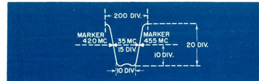
10. Adjust L311 bottom, L312 bottom, T200 bottom, T300 bottom, and C305 for maximum gain and optimum response with markers at 42.0 mc and 45.5 mc. Re-adjust if necessary to obtain proper response, curve, bandwidth, etc., while using sweep width of 6 mc. at center frequency of 43.75.
