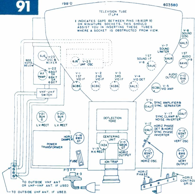
**NOTE:** THE R.F. AMP. TUBE PRESENTLY USED IS A 6BK7 IN THE FUTURE A 6BQ7, 6BQ7A OR A 6BZ7 MAY BE USED. THESE THREE TUBES ARE INTERCHANGEABLE, BUT DUE TO POSSIBLE VARIATIONS IN INTERELECTRODE CAPACITIES, SEVERAL TUBES MAY HAVE TO BE TRIED FOR BEST RESULTS.
