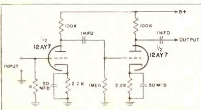
Fig. 10—One type of RC equalizer and its output curve. Equalizers compensate for the attenuation of low-frequency audio signals during recording.
