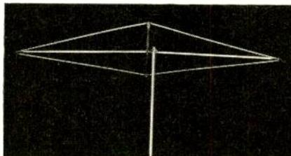
scopic insulators, weatherproofed terminals and resistor, and is designed to provide an impedance match to 300-ohm transmission line. Brach Mfg. Corp., Div. of General Bronze Corp., 200 Central Ave., Newark 4, N. J.—TECHNICIAN.
