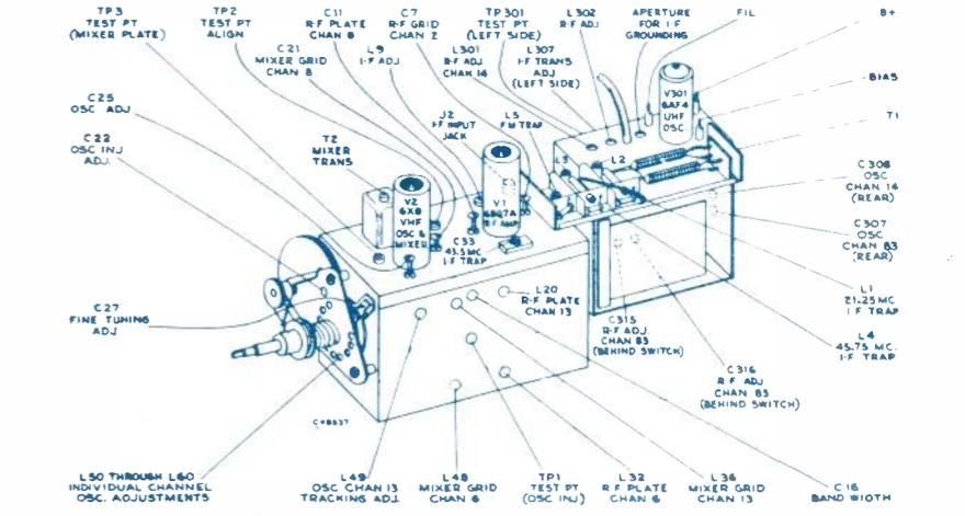
Figure 9—KRK29A/27 Tuner Adjustments
