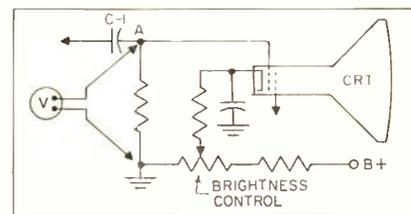
Fig. 4—Conventional brightness control circuit. A check for leakage in C-1 is made by connecting the voltmeter between point A and ground.
