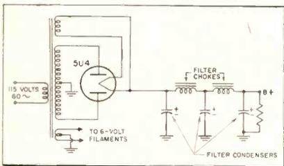
Fig. 7—Schematic of simple but satisfactory power supply.
