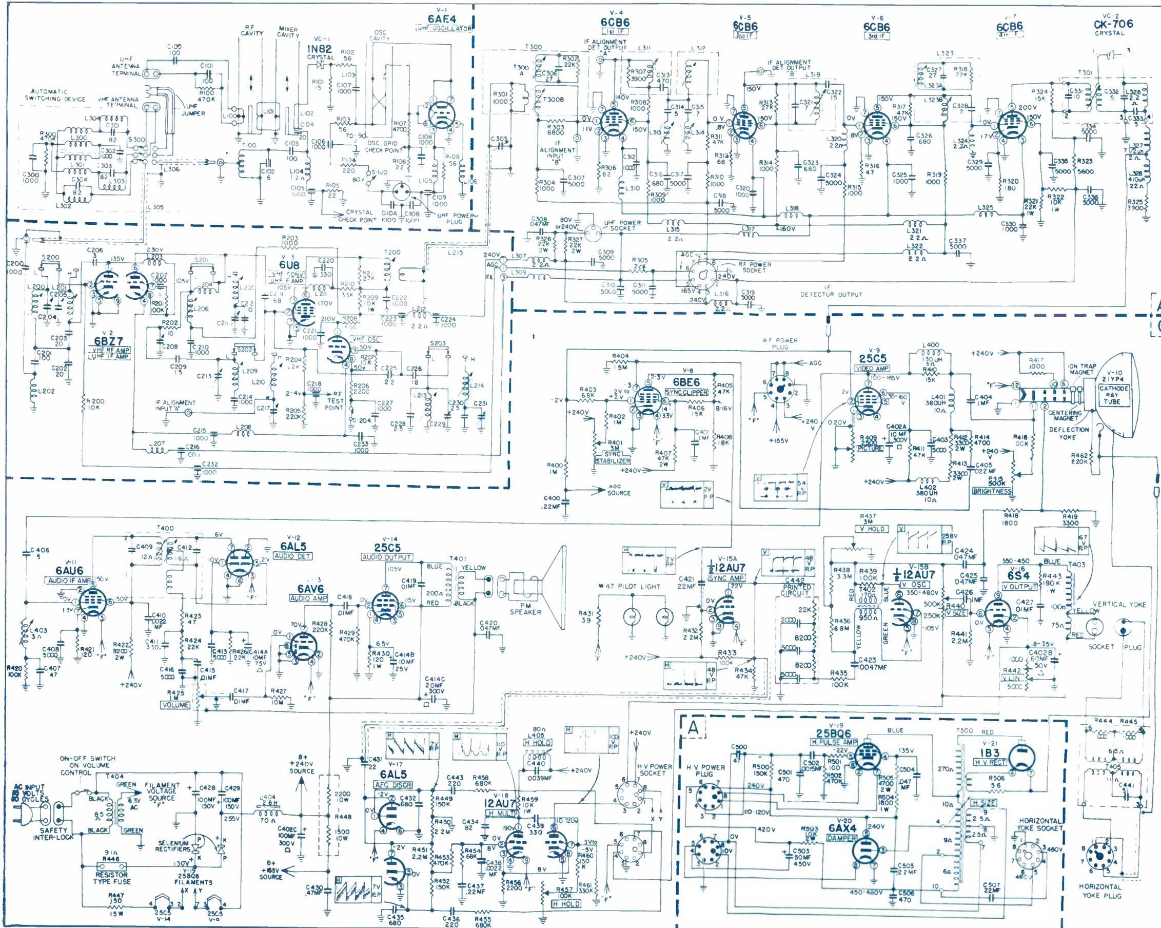
**CAPACITORS** Capacitor values are represented in Micro-microfarad (M $\mu$ F) unless otherwise indicated. "M $\mu$ " denotes microfarad.
