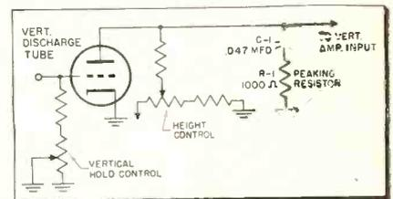
Fig. 4—Vertical discharge tube circuit, showing location of peaking resistor.
