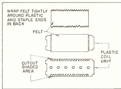
tacts, and remove the coils and forms. Clamp the plastic body of the coil unit in a vise, and file out the shaded areas, within the dotted lines, as shown in the illustration. Cut a piece of hard felt to the width of the filed-out notch. Wrap the felt around the coil unit, fitting it into the filed notches. Pull the ends tight and staple or sew them together. Repeat this job with the second coil unit.
