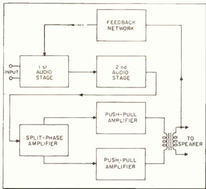
Fig. 4—Block diagram of Hi-Fi Amplifier.
