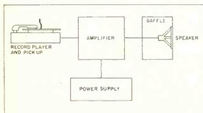
shows the basic requirements for a Hi-Fi set-up; usually what the ordinary enthusiast starts out with, perhaps periodically adding optional units to expand the system to that shown in Fig. 1.
