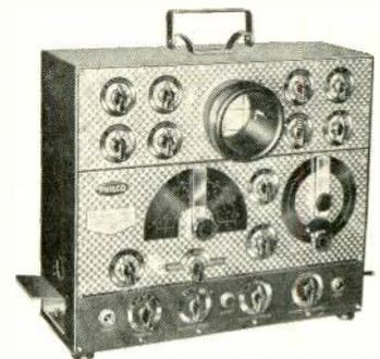
**Model 7008—Visual Alignment Generator** • Combines in one economical unit functions ordinarily found only in a cumbersome collection of costly devices . . . Includes extra sensitive built-in oscilloscope . . . AM, FM, and audio generators. Sweep output flat to within .2 DB/MC.
