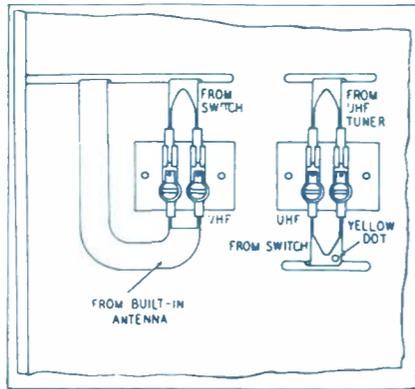
**Antenna-Lead Connections, Common Built-In Antenna**
