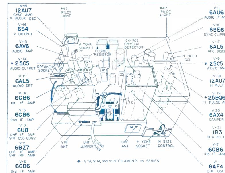
PRELIMINARY ALIGNMENT PROCEDURE FOR 21T8 and 24T2 CHASSIS
