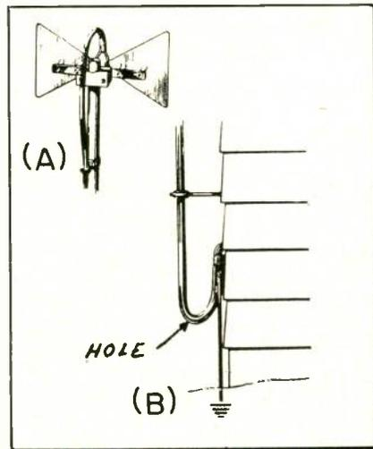
Fig. 2—A) Downward loop is made at antenna when tubular line is employed. B) "Drip loop" is also provided at a point near the one where the tubular line enters the house. A small hole is cut at the point indicated, for drainage.
