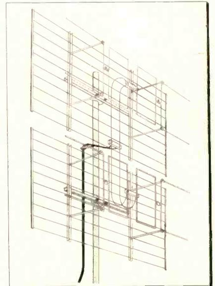
are of aluminum construction throughout, including the screen. Both antennas require only one transmission line. Each model is available in three variations—502 and 504A, B, and C. The A-B-C variations are designed to peak on the following channel range: A, Channel 14 through 32; B, Channel 29 through 55; C, Channel 53 through 83. A stacking arrangement is also available for double stacking the two-bay unit. Finney Co., 4612 St. Clair Ave., Cleveland 3, Ohio.—TECHNICIAN.
