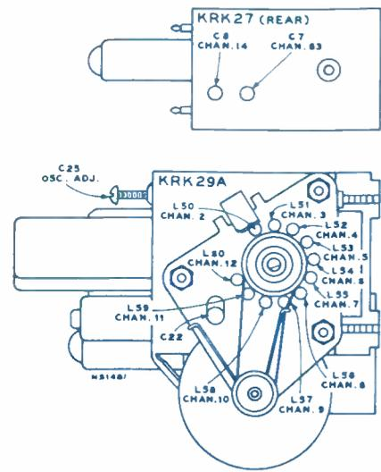
Figure 10—KRK29A/27 Oscillator Adjustments
