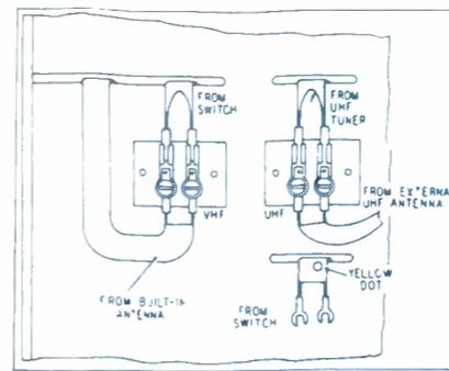
**Antenna-Lead Connections, VHF Built-In and UHF External Antennas**
