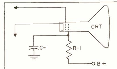
Fig. 5—If R-1 in this circuit open-circuited intermittently, a slow fade-out but rapid reappearance of the picture would tend to take place.
