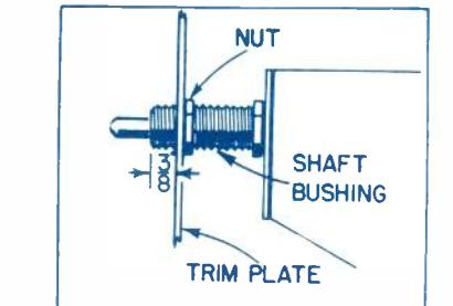
Figure 11. Adjusting Nuts on Shaft Bushing
