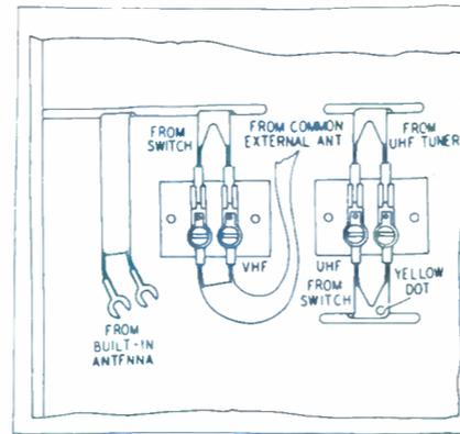
**Antenna-Lead Connections, Common External Antenna**
