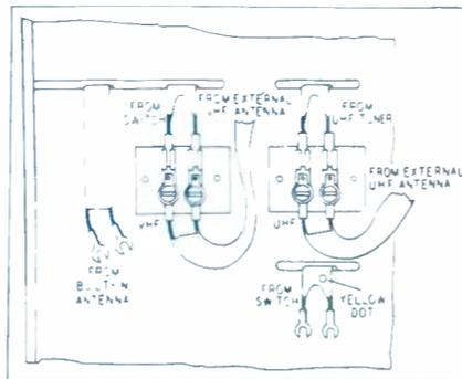
**Antenna-Lead Connections, Separate External Antennas**
