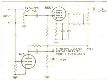
Fig. 12—Volume expander. This circuit compensates for amplitude-compression during recording.
