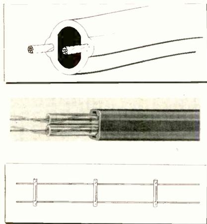
Fig. 1—(Top) Tubular line. (Center) Rectangular line. (Bottom) Open-wire line.
