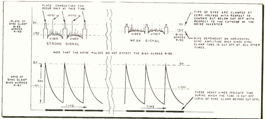
Fig. 3—Waveforms at plate and grid of sync clammer, illustrating why noise pulses do not affect the bias supplied to the noise inverter by the sync clammer.
