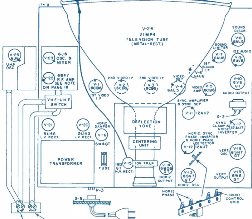
**I** INDICATES GAPS BETWEEN PINS 1 & 7 (OR 9) ON MINIATURE SOCKETS. THIS SHOULD ASSIST YOU IN INSERTING THESE TUBES WHERE A SOCKET IS OBSTRUCTED FROM VIEW.
