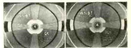
Fig. 5—A—Normal test pattern at left. B—Nonlinear pattern resulting from a reduction in the primary inductance of the vertical output transformer. The Moire effect in the photos is not due to poor interlace—it is the result of the process employed in reproducing the photos.
