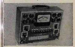
cluded. Individual switches for separate testing of every tube element are provided. Complete kit is priced at \$29.95. Electronic Instrument Co., Inc., 276 Newport St., Brooklyn 12, N. Y.—RADIO & TELEVISION RETAILING.
