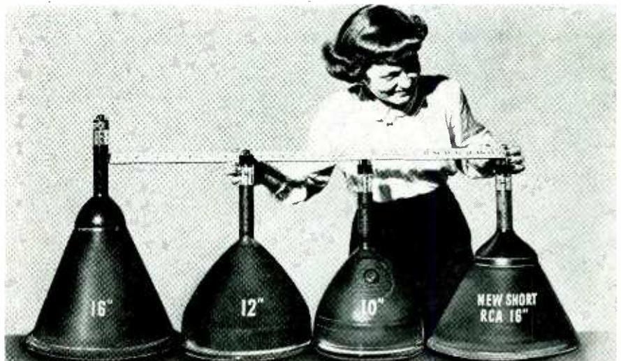
As shown above, the new 16GP4 16-inch metal kinescope is 5 $\frac{3}{8}$  inches shorter than the previous 16-inch tube (16AP4) and is actually shorter than 10- and 12-inch tubes. Shortened length was made possible by the use of 70 degree deflection. The RCA "Filterglass" face plate provides improved contrast.
