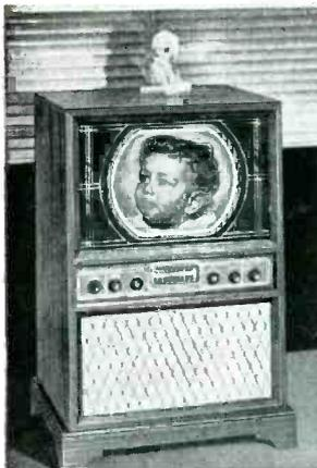
**MODEL CD36**—16" console with AM-FM radio. 36-tube chassis with Voltage Doubler. Mahogany veneer cabinet.
