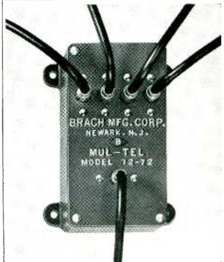
One of three types of distribution units available in the Brach Mul-Tel System. For a 4-set system the cables on the top connect directly to TV sets; in a 16-set system each wire feeds into another distribution unit which in turn supplies 4 sets. Cable on the bottom is 72-ohm coax from the antenna. Provision is made for use of 72 or 300 ohm downlead to any input. (Pat. applied for)
