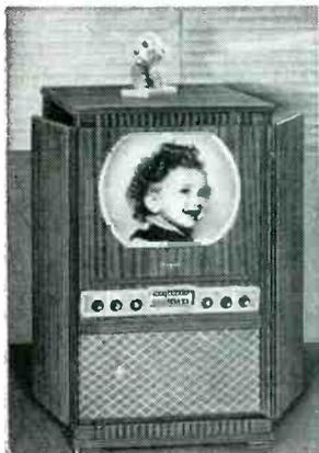
**MODEL 19C36**—19" console with AM-FM radio. 36-tube chassis with Voltage Doubler. Mahogany veneer cabinet with doors.
