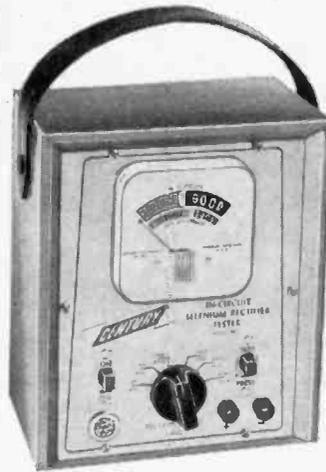
Model SRT-1—housed in sturdy hammertone finish steel case complete with test leads.....only **\$29.50** Net
