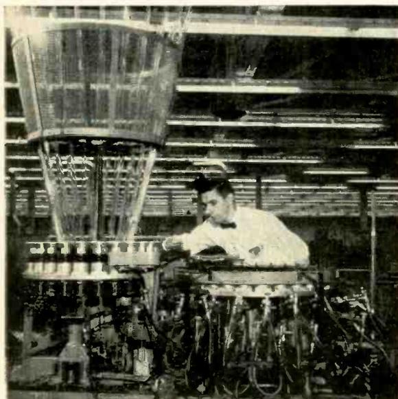
The new double-turret sealex is an important new development. Oil-diffusion pumps work in series with mechanical pumps to produce the most nearly perfect vacuum possible.
