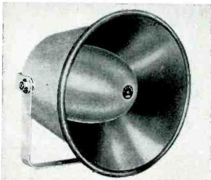
Has 6" cone type driver. Power rating 15 watts; frequency range 140 to 8,000 cps; impedance 8 ohms; dispersion 120°; bell opening 15", depth 12". Atlas Sound Corp., 1451 39th St., Brooklyn 18, N. Y. (ELECTRONIC TECHNICIAN 10-4)
