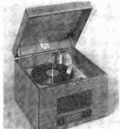
Model 202 radio-phonograph table unit, ac-dc superhet, 6 tubes including rectifier, automatic record changer playing twelve 10" or ten 12" discs. Tunes 550 to 1700 kc, built-in loop antenna, automatic volume control, slide rule dial, Alnico 5 PM speaker. Cabinet of walnut veneers measures 12" by 15 $\frac{1}{2}$ " by 16 $\frac{1}{2}$ ". Weighs 27 lbs. Apex Radio & Television Corp., 192 Lexington Ave., New York 16, N. Y.—RADIO & Television RETAILING
