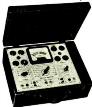
**SPEEDY OPERATION** assured by newly designed rotary selector switch which replaces the usual snap, toggle, or lever action switches.
