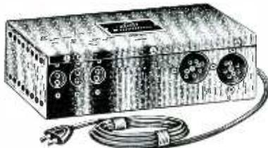
**ELIMINATOR**—An "A" and "B" eliminator for use on 4 to 7 tube 2 volt battery receivers. Operates on 115 volt 60 cycles current; delivers 90 volts of "B" power and required filament voltages. Total power consumption is 14 watts; weight 4½ lbs., list price \$9.95. Electro Products Labs, 549 W. Randolph St., Chicago, Ill.
