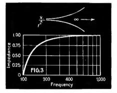
sistance characteristic is 7.5. This should be compared to Fig. 2, a 40 in. mouth shows a variation in resistance of only a few per cent from that of the infinite horn of Fig. 3.
