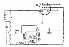
condensers, however, is sometimes the source of an almost impossible-to-find fading difficulty, especially if the condensers have become leaky.
