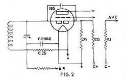
the A.F. going through the 50,000 ohm resistor to the grid of the first A.F. tube and the AVC through the  $\frac{1}{4}$  meg resistor to the grids of the tubes under the AVC action. The disadvantage of
