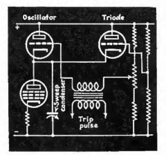
cycle. The frequency of this automatic flashing is determined by the capacity in the circuit and the charging current. To produce a single sweep the oscillator must be prevented from reaching the automatic breakdown point of the sweep oscillator tube. At the same time the tube must be sensitive to a small tripping pulse from an external source.
