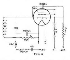
used, should be isolated through the  $\frac{1}{4}$  megohum and 100,000 ohum resistors as shown for best results.
