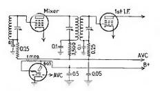
ger the pitch varies as if the dial was being tuned, it is an almost sure indication that the IF tube or tubes are in a state of local oscillation.
