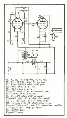
Fig. 2. Diagram of the multivibrator keying circuit. Selenium rectifier type of power supply simplifies construction.
