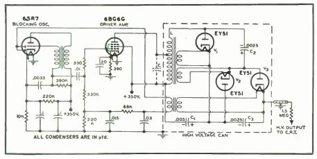
Fig. 6. North American Philips pulse-type high-voltage supply.
