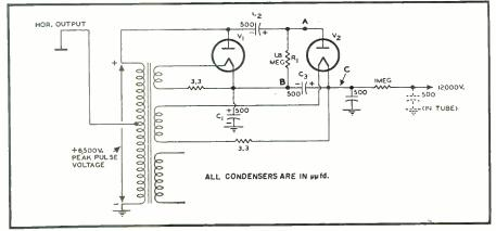
$C_2$  by  $C_1$  reduces the voltage across  $C_1$ . However, after several seconds,  $C_1$  and  $C_2$  are both charged to essentially the full 6500 volts of the pulse.
