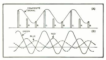
Fig. 6. Operation of the receiving set sampler system.
