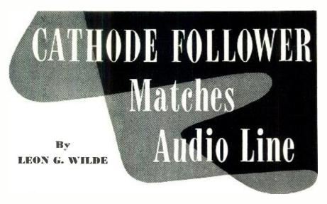
An inexpensive method of matching a 250 or 500 ohm line without a plate-to-line transformer. This system also provides power circuit control over the same line.
