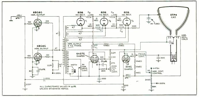
Fig. 4. An extension of the flyback circuit of Fig. 2 to provide 27,000 volts for projection tubes.
