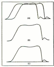
Fig. 1. Video i.f. response curves which indicate proper operation of receiver and test equipment. All curves are normal response of (A) phasing control improperly set. (B) phasing control properly set and (C) blanking switch on generator "On."
