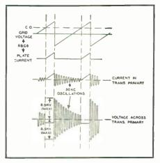
Fig. 7. Operating voltages and currents in the pulse-type unit shown in Fig. 6.
