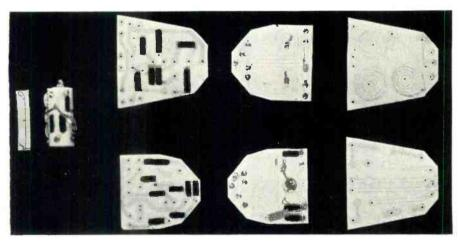
Fig. 7. Partially completed electronic circuits printed on steatite plates and cylinders by the silk-screen process. Light lines are silver conductors and inductors; dark rectangles are resistors; circular disks are ceramic condensers.
