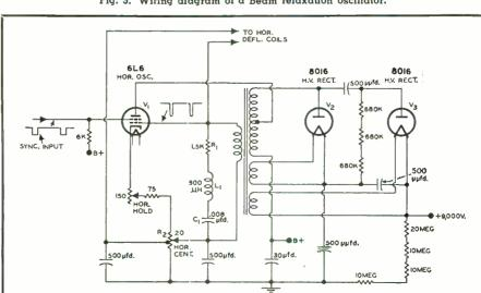
Fig. 5. Wiring diagram of a beam relaxation oscillator.
