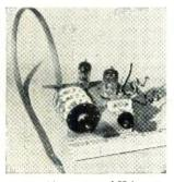
This compact front end hos a stage of RF for extra distance. Made to conform with Telekit or any TV set having a video I.F. of 25.75 Mc. Complete with tubes, pre-wired, pre-assembled. Only four connections to make.
