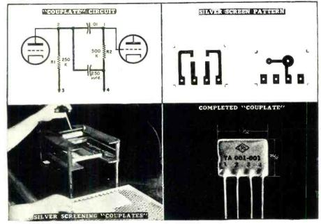
screen are not the only ways in which the conducting and resistor paints are applied. For example, a decalcomania, on which the circuit is printed on a thin flexible film that can be transferred to the final surface, is useful in applying the circuits to cylindrical or irregularly-shaped objects. The film is removed by firing.
