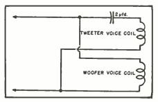
Both the parallel and series type of networks are effective, but listening tests seem to favor the series type (Fig. 2B).
