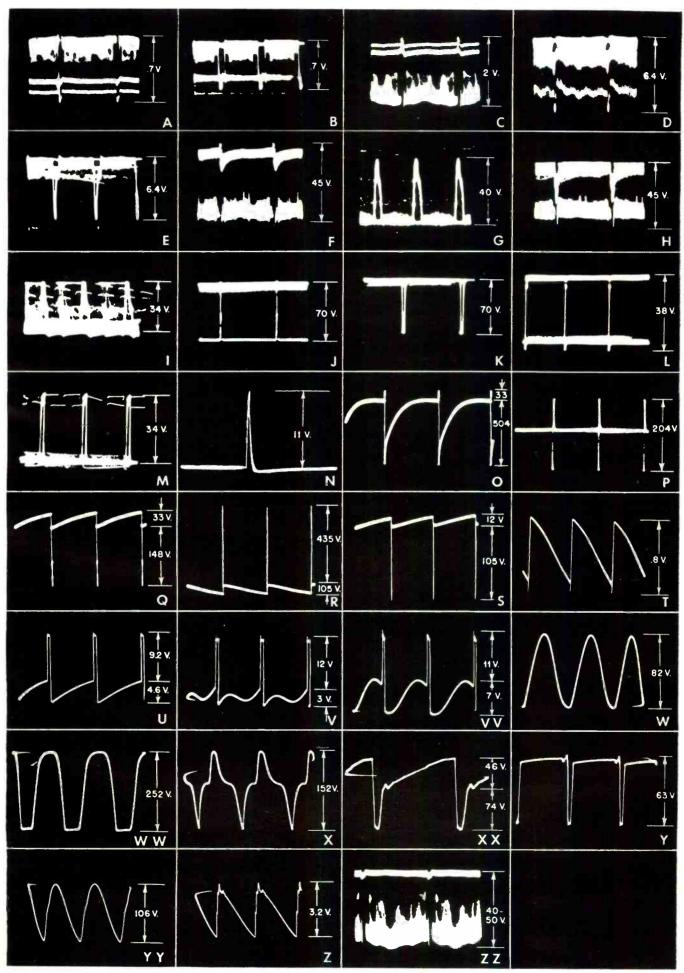
odd number of units is obtained, increase or decrease the vertical gain of the scope until an even number of units can be counted. This will make direct reading of the deflection percentage much easier. Once the scope is calibrated, the amplitude of each waveform can be determined simply by connecting the scope leads to the desired test point.
