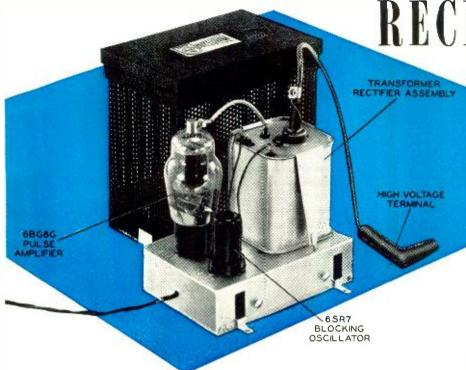
Part 20. A description of flyback and pulse-type high-voltage power supplies that are part of the horizontal deflection systems of TV receivers.
