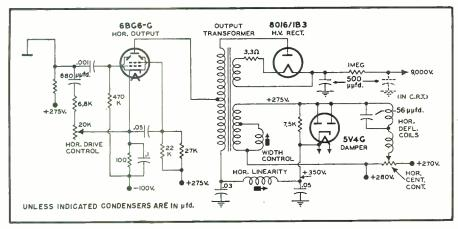
Fig. 1. Conventional circuit diagram of a flyback power supply.
