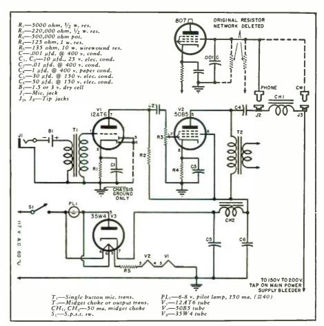
Schematic diagram of the modulator, showing the changes in screen wiring.
