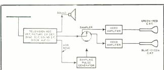
Fig. 3. Block diagram of RCA's color television transmitter.
