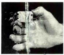
such units are eliminated, and the whole is sealed in solid plastic to keep it moisture, dust, shock, and tamperproof. Pattern for the design was the plug-in type of component used by the Armed Forces. Further details may be had by writing the company at Ford Parkway, St. Paul 5, Minn.
