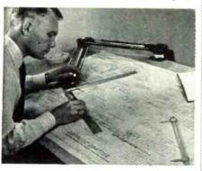
tion and hold it. Other features are a base line clamp for greater convenience in aligning the drafter to the drawing, ball joints on both arms for flexibility, and increased space between the double thumb screws that improve anchorage.
