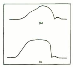
Fig. 5. Effect of overloading on shape of response curve. (A) Response curve of picture i.f. amplifier, showing poor alignment. (B) Response curve of same amplifier with sweep generator output turned up so as to overload amplifier. Notice the false indication of good alignment.
