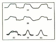
Fig. 2. Effect of oscilloscope on visual alignment waveforms. (A) Normal waveform fed to scope. (B) Distortion introduced if scope does not have good low-frequency response. (C) Effect of low-frequency distortion on normal response curve. (D) Effect of low-frequency distortion on normal response of sound i.f. amplifier. (E) Normal response of sound i.f. amplifier.
