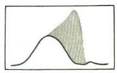
Fig. 4. Effect of oscillation of the picture i.f. amplifier as noted on response curve. The wide beat pattern shown will be seen only when an oscilloscope having good video frequency response is used. If the oscilloscope is not designed to have good video frequency response, then the beat pattern will be narrower, may look somewhat like a marker pip.
