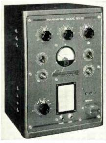
A 50 watt bandswitching transmitter for both phone and c.w., made by Harvey-Wells. Covers all ham bands from 2 to 80 meters.
