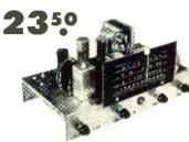
Ideal AC operated superheterodyne receiver for home use or replacement in console cabinet. Comes complete with attractive metal panel for cabinet mounting. Modern circuit uses 12K8 converter, 12SH7 input IF stage, 12C8 output IF stage and first audio 12A6 beam power output stage, 5Y3 rectifer. Excellent sensitivity for distant reception with selectivity which effectively separates adjacent stations.
