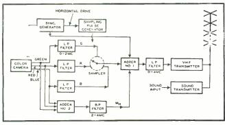
Fig. 4. Method of operation employed in the sampler system.
