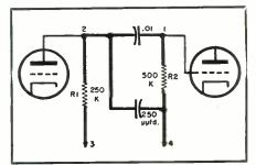
carefully trace out the heavy lines with a small brush which we have dipped into a "paint" made by mixing fine particles of silver together with a liquid binder to hold the particles together and a solvent used to make the mixture thin enough to brush.
