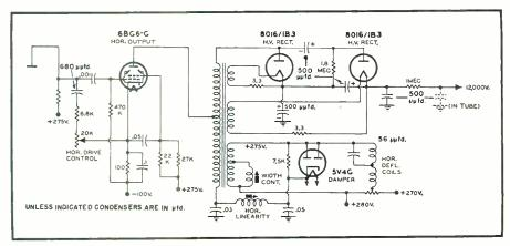
Fig. 2. A flyback high-voltage supply unit capable of producing 12.000 volts.
