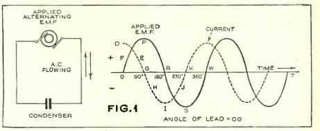
Figure 1-Effect of capacitance on the phase relations between current and applied voltage in an alternating current circuit.
