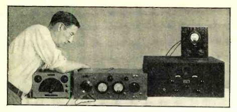
MEASURING RECEIVER SENSITIVITY The author is shown making a set-up for actual measurements of receiver sensitivity, a feat made possible by the unusual V.T. voltmeter described in this article. Below is a "block" diagram of the set-up.
