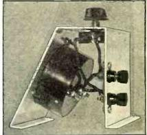
TUNING METER STAND A strip of aluminum is bent as shown to accommodate the meter, its shunt rheostat and binding posts. Wood or bakelite may be used in place of aluminum if preferred.
