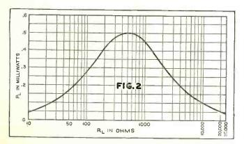
ohms to 500 ohms and see what happens to  $P_{L}$ . The result is shown by the graph in Figure 2. Note that  $P_{L}$  is a maximum when  $R_L$  has the same value as  $R_s$ , which is 500 ohms in this case.
