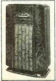
mer capacitor. The photograph shows the model A125 all-wave console which employs 12 metal type tubes.
