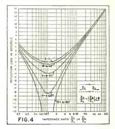
REFLECTION LOSS FOR DIFFERENT PHASE ANGLES Figure 4. Reflection loss plotted against impedance ratio for various values of  $\phi$ ,  $Z_S$  and  $Z_L$  are complex quantities, while the vertical lines around a symbol (as  $\left| \frac{Z_S}{Z_L} \right|$ ) denote the scalar quantities. tity without regard to the phase angle.
