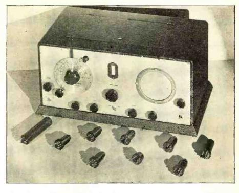
throughout as follows: a 6K7 in the r.f. pre-selector stage; 6L7 as first detectormixer; a 6C5 as the oscillator; a 6K7 as the i.f. stage; a 6H6 as the second detector and avc tube; a 6K7 as the electron coupled beat oscillator; a 6F5first audio, a 6F6 second audio and output tube and a 5Z4 rectifier. The 6L7tube used here has no parallel in the glass tubes.
