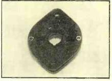
spring-prong contacts. The mounting center spacing is 11/2 inches.
