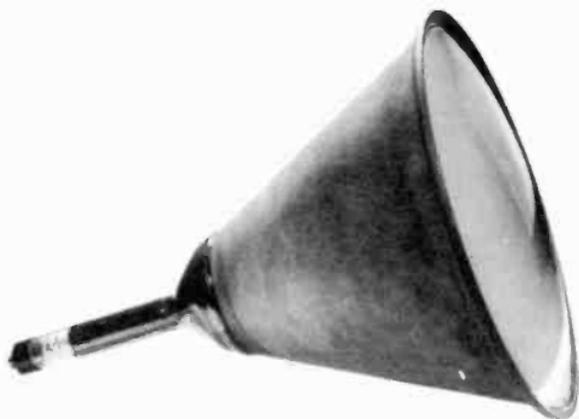
Figure 130. Picture tube with metal funnel.
