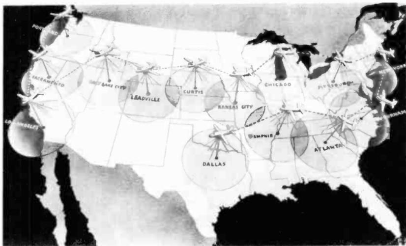
Figure 82. How coverage of United States would be secured using stratovision. (courtesy Westinghouse)
