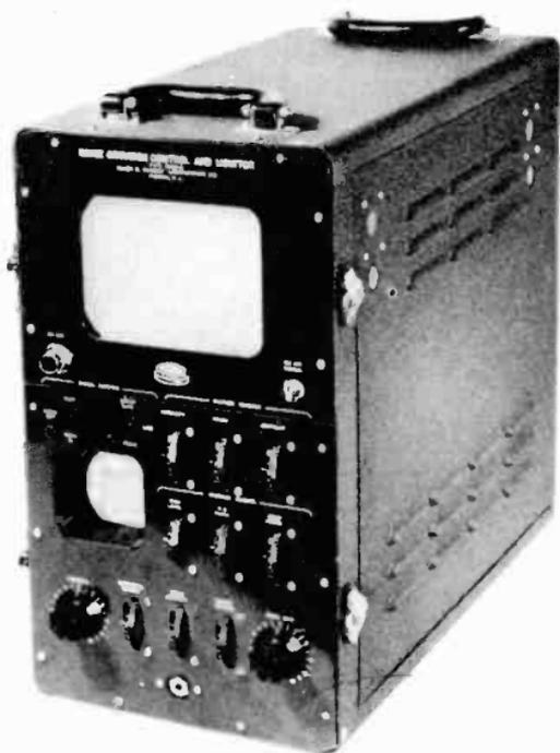
Figure 75. Camera control monitor. (courtesy DuMont)
