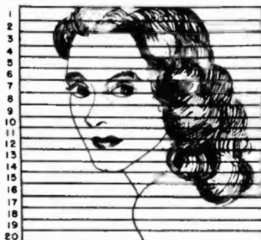
Figure 9. How linear scanning is accomplished.
