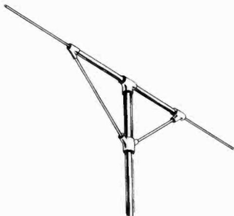
Figure 32. Extended V antenna.
