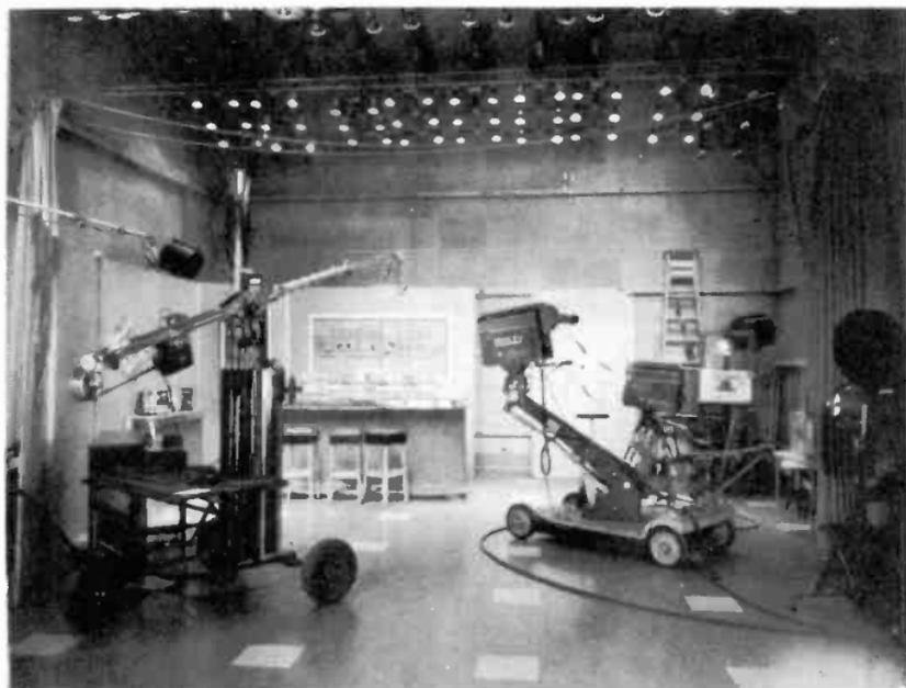
Figure 87. Studio set and boom camera. (courtesy WFIL-TV)
