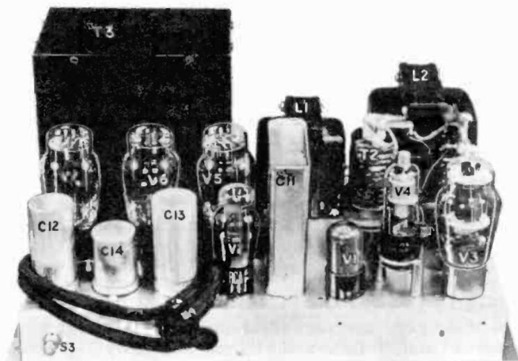
Figure 31. Power supply chassis.
