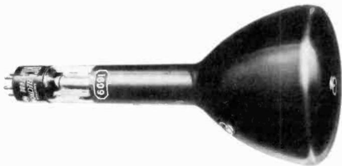
Figure 13. Monoscope tube. (courtesy RCA)
