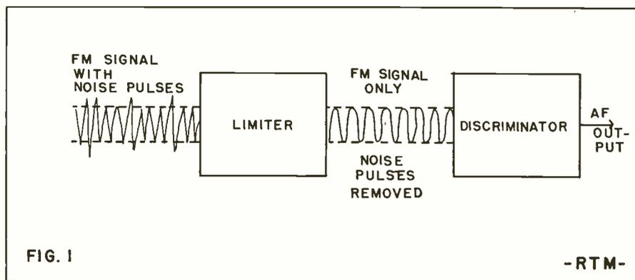
Limiter-discriminator demodulating system used in most present-day FM sets.
