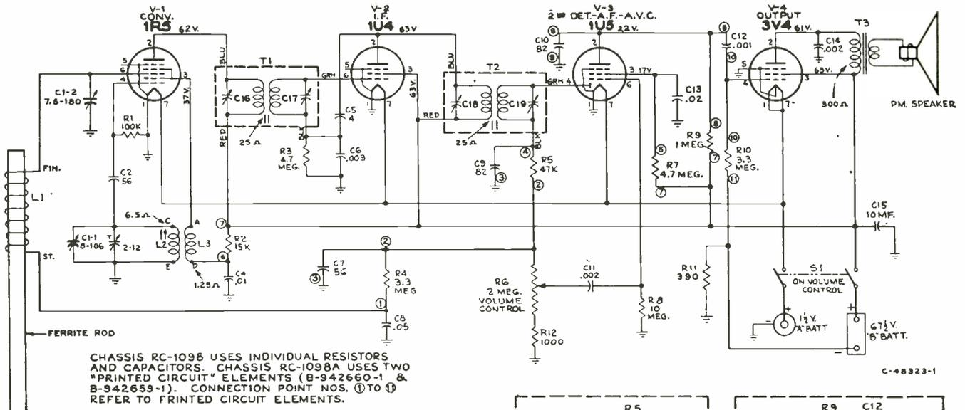
CHASSIS RC-109B USES INDIVIDUAL RESISTORS AND CAPACITORS. CHASSIS RC-1098A USES TWO "PRINTED CIRCUIT" ELEMENTS (B-942660-1 & B-942659-1). CONNECTION POINT NOS. ① TO ⑩ REFER TO PRINTED CIRCUIT ELEMENTS.
