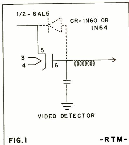
Crystal detector used for demodulation of a TV video signal. Use of crystals in place of vacuum diodes is increasing with TV design development.
