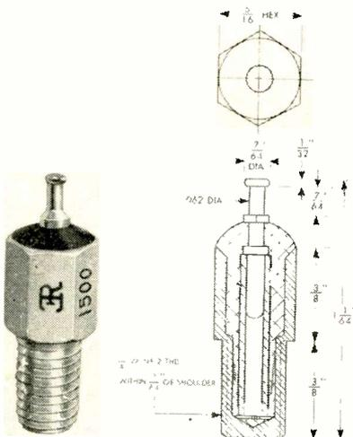
outer electrode at the plane of the chassis. The result is an extremely low and uniform series inductance. In assembly operations both location and length of leads are accurately fixed, resulting in mechanical uniformity. This feature has been demonstrated to be of importance in good VHF and UHF design.
