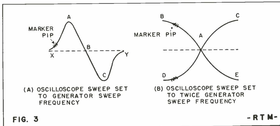
Scope traces found in FM alignment under ideal conditions. At (A), scope's sweep frequency equals generator sweep frequency. At (B), scope sweep is double that of the wobbulator.
