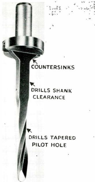
The shoulder on the tool stops the drill at just the right depth, while the size of the drill is slightly smaller than the body of the corresponding wood screw to provide a snug fit. Screw-Mates fit any drill gun, hand drill, or drill press and are available in a variety of sizes.
