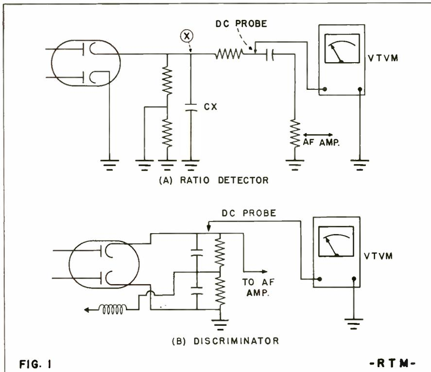
Meter connections for ratio detector or discriminator alignment, for the preliminary quick-check outlined in the text. This check is made to find out whether the FM set under test is in operating condition, and to show how badly it may need alignment.
