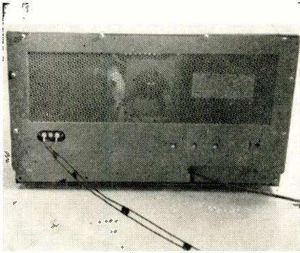
Separate wires spaced with electrical tape can serve as a substitute for 300-ohm transmission line in an emergency.
