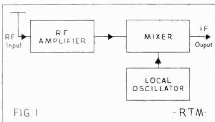
Block diagram of a typical TV tuner.
