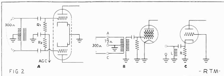
Television input circuits. At A, a balanced 300-ohm input is shown, with a center-tapped choke. Circuit B shows an input with choice of either 300- or 75-ohm input, balanced one way, and unbalanced the other. At C, the 75-ohm input is into a grounded-grid RF amplifier. Input impedance depends largely on the value of resistor R.
