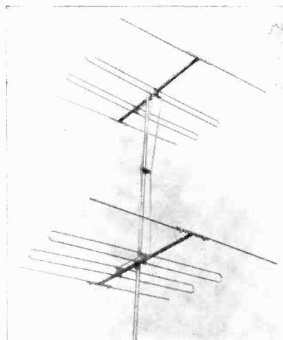
design is said to sacrifice no forward gain, yet to maintain an average of 30 Db front-to-back ratio throughout the entire 6 megacycle bandwidth of the channel for which it is tuned. Terminal impedance has been maintained at 300 ohms to match standard leadin.
