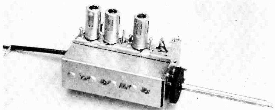
The "Teletuner," a complete front end built by Mallory around its four-gang "Inductuner" (see cut at bottom of page).
