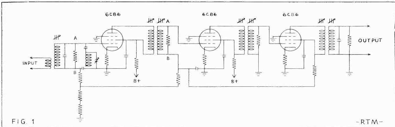
Test points on the grid resistors of video IF stages. Service procedure with only VTVM and other basic field equipment (see text) will usually
