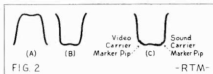
Tuner response curves may be upright or inverted on the 'scope face.
