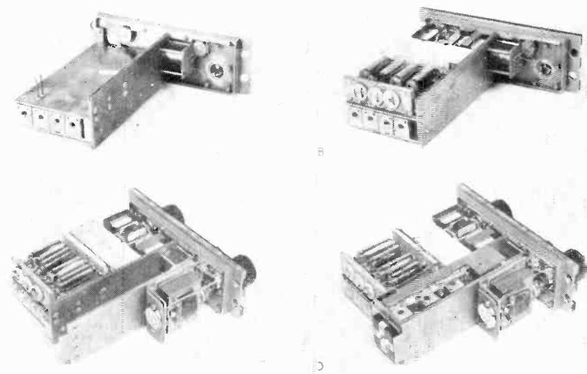
Subassemblies used in the new receiver. A shows tuning assembly and RF inductors in place. At B, RF amplifier and power-filter assemblies have been added. At C, output transformer, potentiometer, and other hardware are in place. At D, IF amplifier, input-output connector are installed and the set is ready to be sealed in its case. Audio output tube assembly is plugged on the outside of case for easy replacement.
