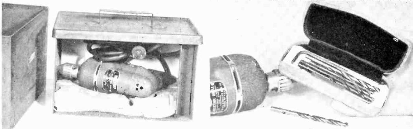
An ammunition carrier can easily be made into a handy carrying case for the quarter-inch drill gun. At left, gun is shown resting on sponge rubber inside the drawer of the case. At right, an old spectacle case makes a good holder for drill bits, chuck tightening key, other small accessories.
